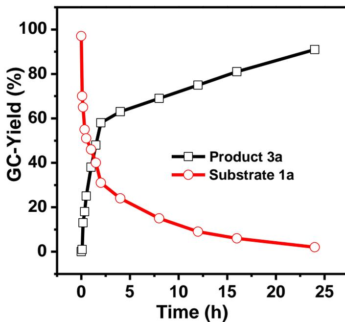
Figure S15 Formation of product 3a and decrease in concentration of 1a with reaction time in presence of catalyst MnPhen@ZIF.
