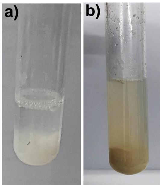
**Figure S5** Physical appearances of Mn-NaOH test for MnPhen@ZIF a) without, and b) with acid.
