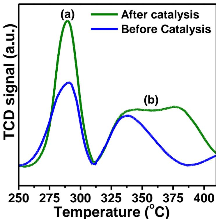
Figure S13 NH<sub>3</sub>-TPD profiles for MnPhen@ZIF before and after catalysis.
