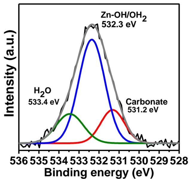
Figure S14 O 1s XPS spectrum of MnPhen@ZIF after catalysis
