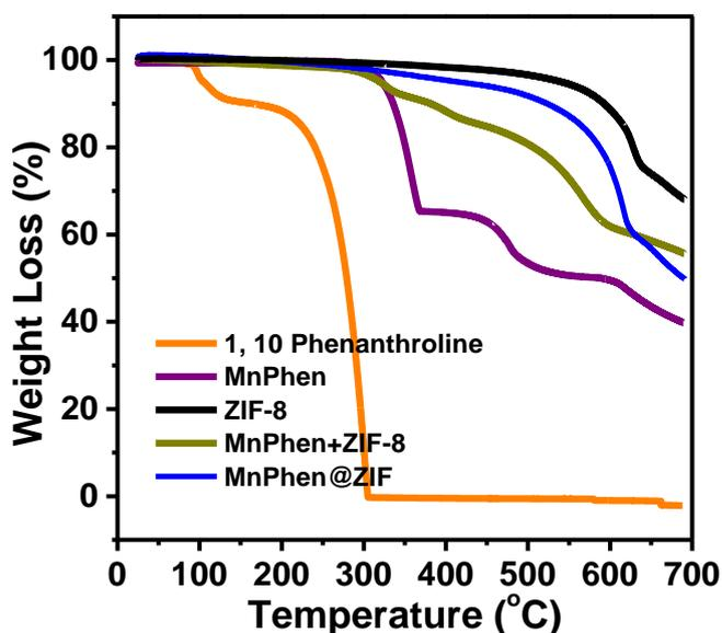
**Figure S12** A comparison of TGA curves of as-synthesized catalyst MnPhen@ZIF, a mixture of MnPhen+ZIF-8 complex, pristine ZIF-8, MnPhen complex, and Phen ligand itself. This data suggests that MnPhen@ZIF and its encapsulated Mn-complex is stable under experimental catalytic reaction temperature i.e; at 140 °C.
