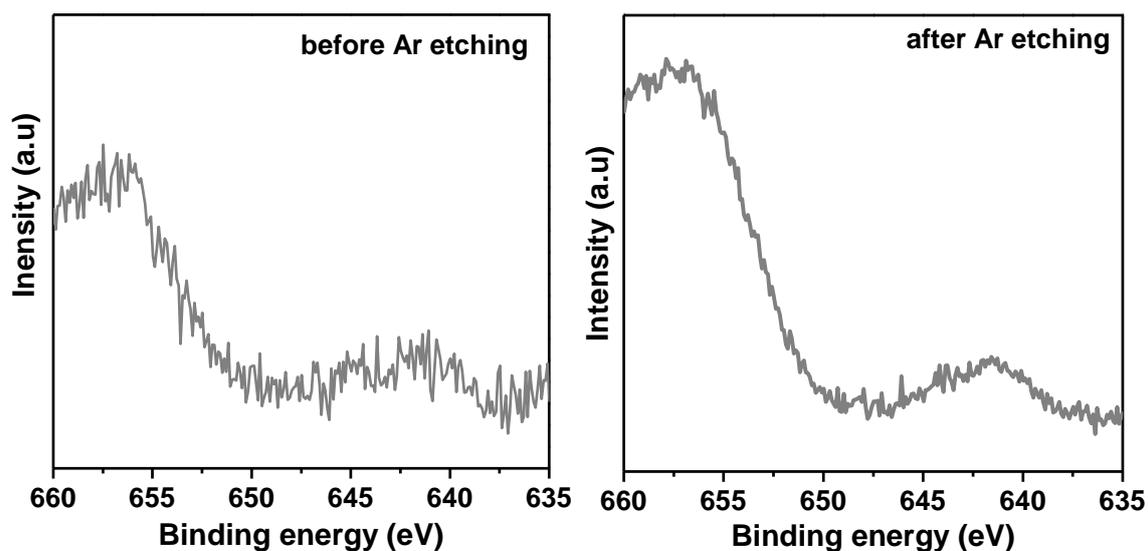
**Figure S3** Mn 2p XPS spectra of MnPhen@ZIF before Ar-etching (left), and after Ar-etching (right). This Ar-sputtering suggests the presence of more Mn in the bulk of MnPhen@ZIF crystals.
