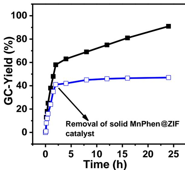
**Figure S11** Hot filtration test indicating no further formation of branched ketone product 3a after removal of solid MnPhen@ZIF catalyst. Black line curve is product formation vs time plot till completion of the reaction (24 h), while blue curve is for second batch of reaction where catalyst was removed by hot filtration at the time of ~2 h.
