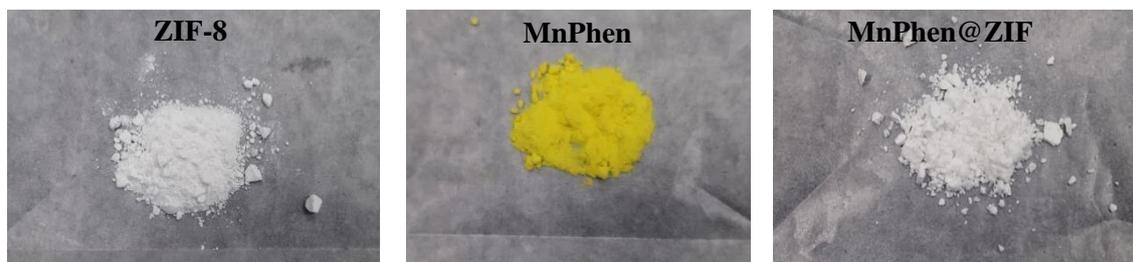
**Figure S4** Physical appearance of pure ZIF-8, manganese phenanthroline complex (MnPhen) and as-synthesized catalyst MnPhen@ZIF.
