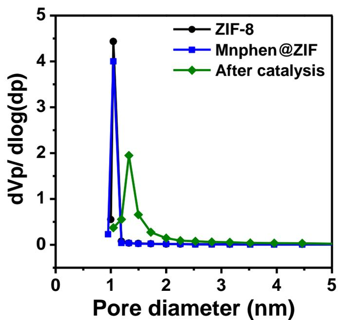
**Figure S10** Pore size distribution of ZIF-8, MnPhen@ZIF (before catalysis), and MnPhen@ZIF (after catalysis).
