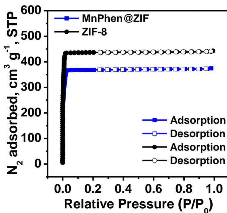
**Figure S2**  $N_2$  sorption isotherms of ZIF-8 (black) and Mnphen@ZIF (blue), recorded at 77 K. Filled and open circles represent adsorption and desorption, respectively.
