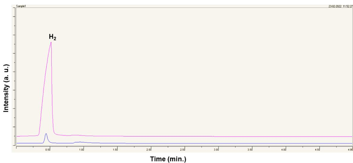
**Figure S7** The set-up made for the collection of generated H<sub>2</sub> gas in the reaction (conditioned were same as mentioned in section 5) (above). Gas chromatographs of the collected gas in reaction mentioned as blue line, which has same retention time as pure H<sub>2</sub> shown in pink line (below).
