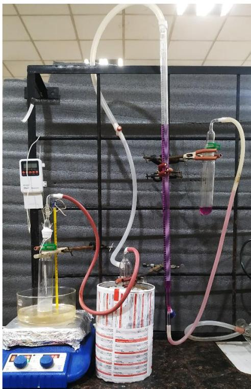
**Figure S6** The set-up made for the measurement of generated H<sub>2</sub> gas in the reaction.
