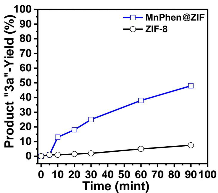
**Figure S16** Comparison of product 3a formation with respect to initial period of time in presence of catalyst MnPhen@ZIF and ZIF-8.
