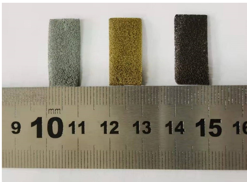
Fig. S1. Optical photographs of the Ni-MOF/NF, Ni-MOF@PBA/NF and the Fe-Ni 3 S 2 /NF with the size of 1.0 × 2 cm 2 .
