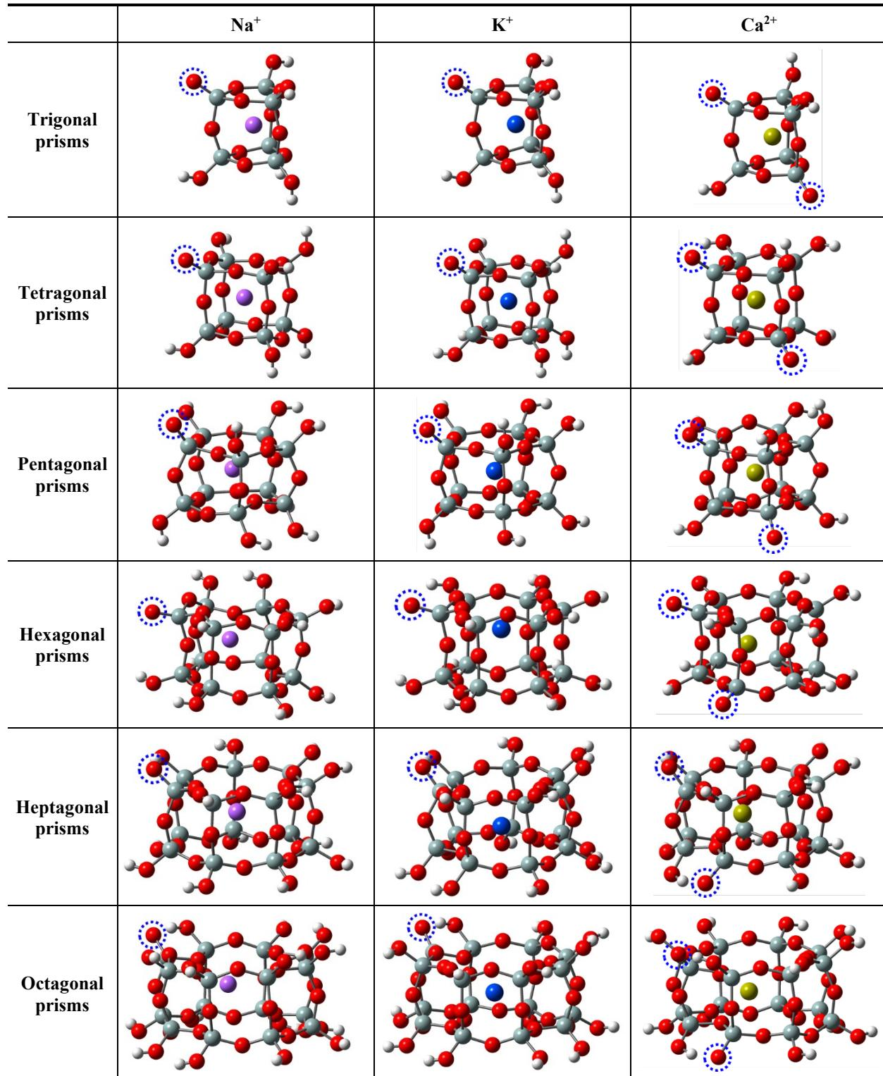
**Table S6.** Optimized molecular structures of aluminosilicate cages with an internal cation (grey ball = Si, pink = Al, red = O, white = H, purple = Na, blue = K, and yellow = Ca). The oxygen sites from which a proton is removed to maintain overall charge neutrality are highlighted with blue dotted circles.
