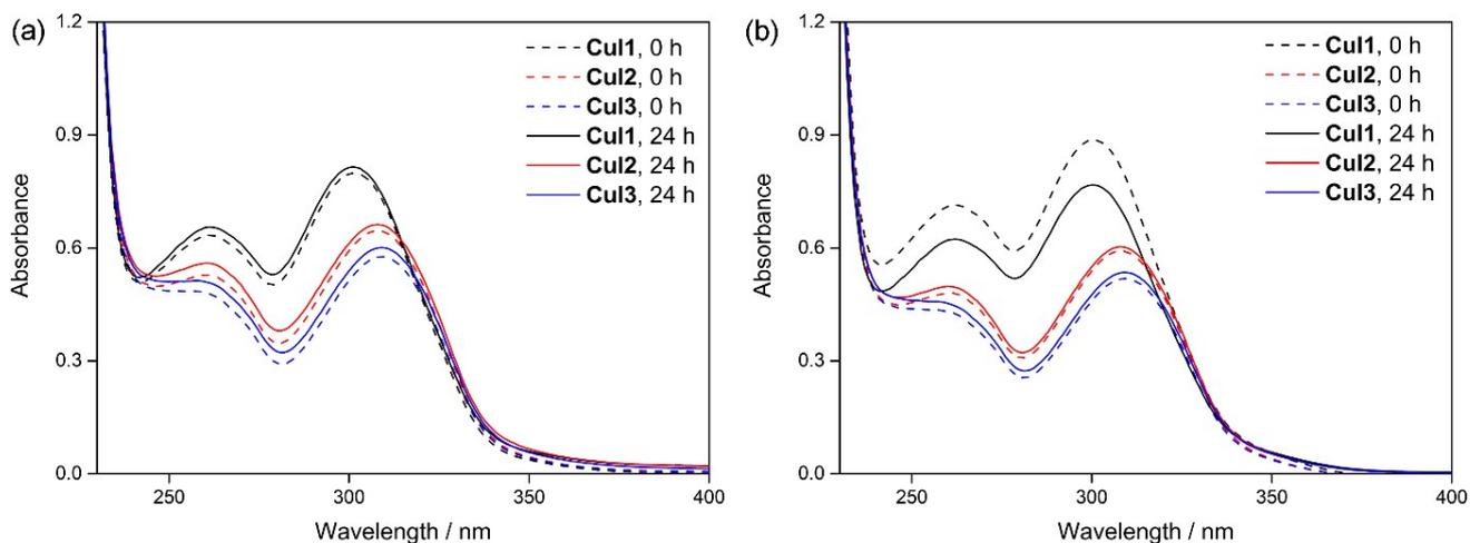
**Fig. S2** UV-Vis spectra of the complexes (50  $\mu$ M) in (a) Tris-HCl/NaCl buffer (pH = 7.2) and (b) PBS (pH = 7.4). Time intervals: 0 and 24 h.
