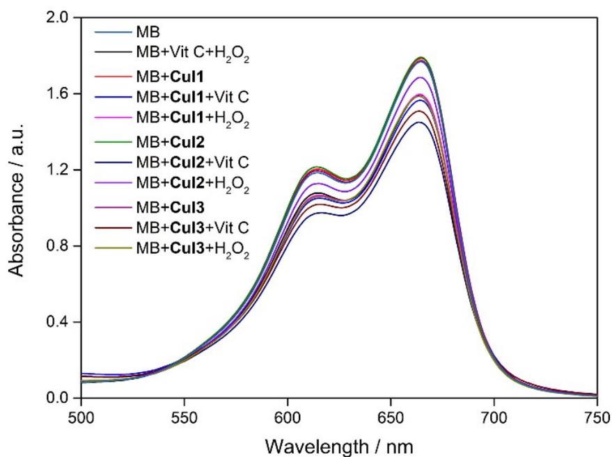
**Fig. S3** Detection of  $\cdot$ OH mediated MB degradation in different solutions by UV-Vis absorption spectra ( $[\text{Cu}] = 0.05 \text{ mM}$ ,  $[\text{H}_2\text{O}_2] = 8 \text{ mM}$ ,  $[\text{Vit C}] = 2.5 \text{ mM}$ ).
