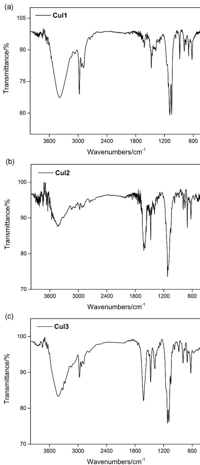
**Fig. S1** Infrared spectra of **CuI1** (a), **CuI2** (b) and **CuI3** (c) with KBr tablets at room temperature.
