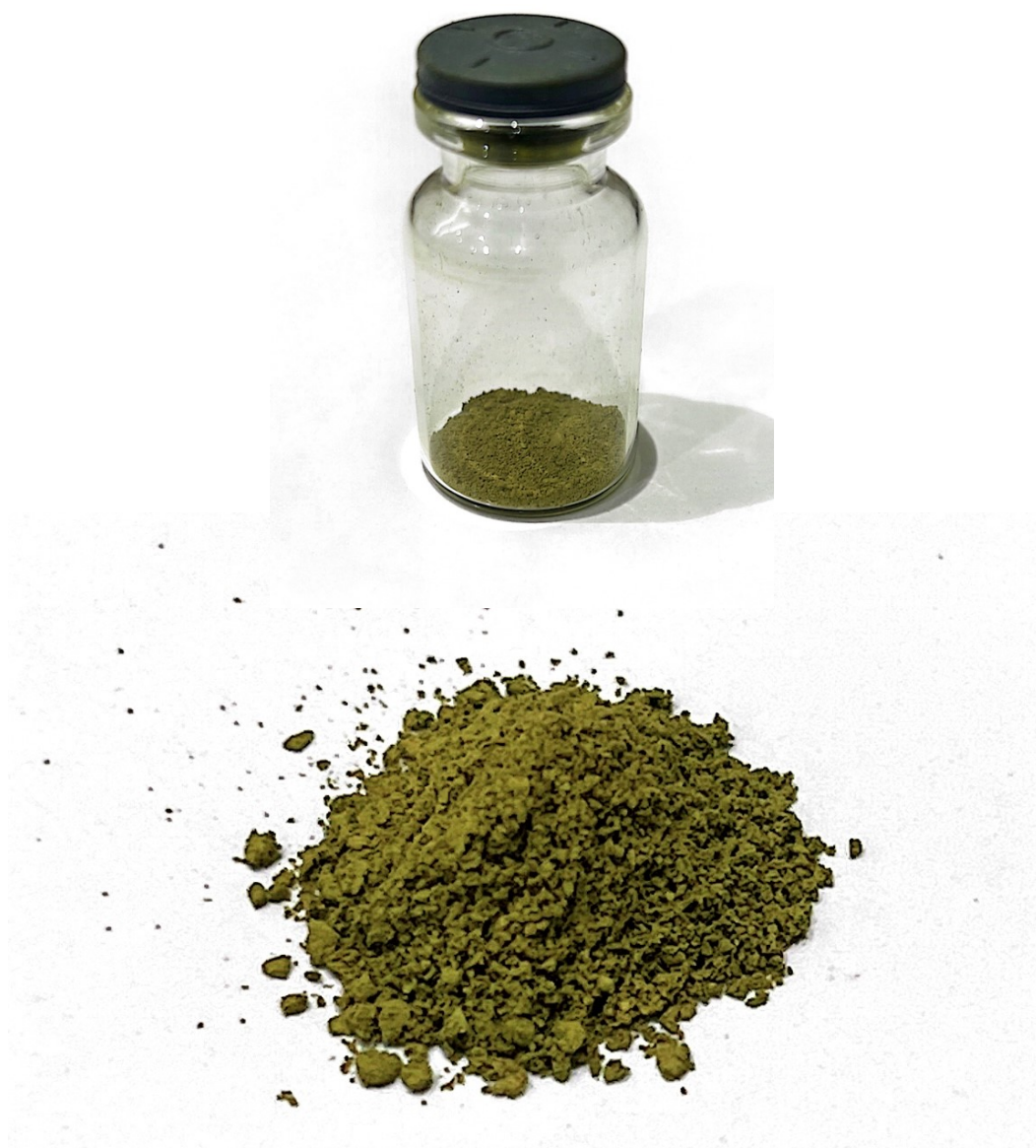
Fig. 30. Green powder (Si-Cu) obtained from the reaction of compound 1 and propionyl chloride functionalized silica gel
