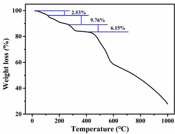
**Fig. S4** The TGA curve for **JXUST-25** under  $\text{N}_2$  atmosphere.
