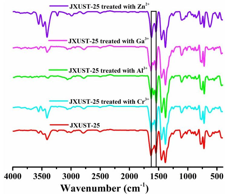
**Fig. S2** The IR spectra of JXUST-25 before and after treated with Cr<sup>3+</sup>, Al<sup>3+</sup>, Ga<sup>3+</sup> and Zn<sup>2+</sup> at room temperature.
