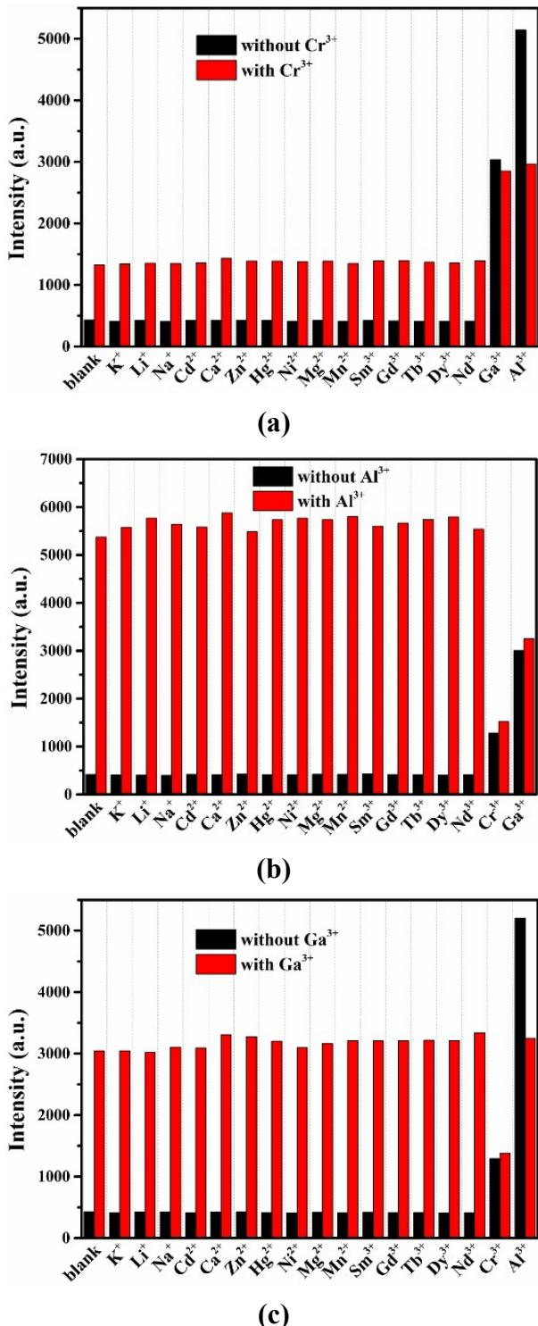
**Fig. S7** Competitive experiments of JXUST-25 in sensing (a)  $\text{Cr}^{3+}$ , (b)  $\text{Al}^{3+}$  and (c)  $\text{Ga}^{3+}$  with the interference of other metal ions (0.2 M) in DMF solution.
