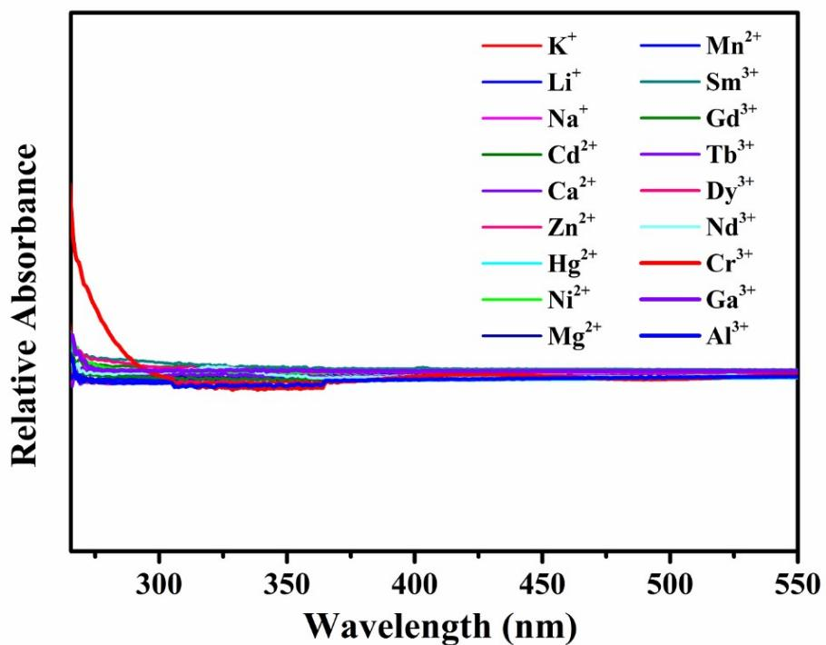
**Fig. S12** UV-vis absorption spectra of different metal ions in DMF solutions.
