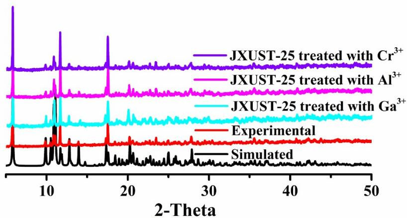
**Fig. S9** The PXRD patterns of JXUST-25 in DMF solution after adding  $\text{Cr}^{3+}$ ,  $\text{Al}^{3+}$  and  $\text{Ga}^{3+}$  for 24 h.
