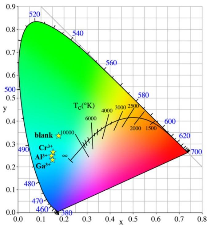
**Fig. S6** CIE chromaticity diagram showing the color coordinates of **JXUST-25** upon the addition of  $\text{Cr}^{3+}$ ,  $\text{Al}^{3+}$  and  $\text{Ga}^{3+}$ .
