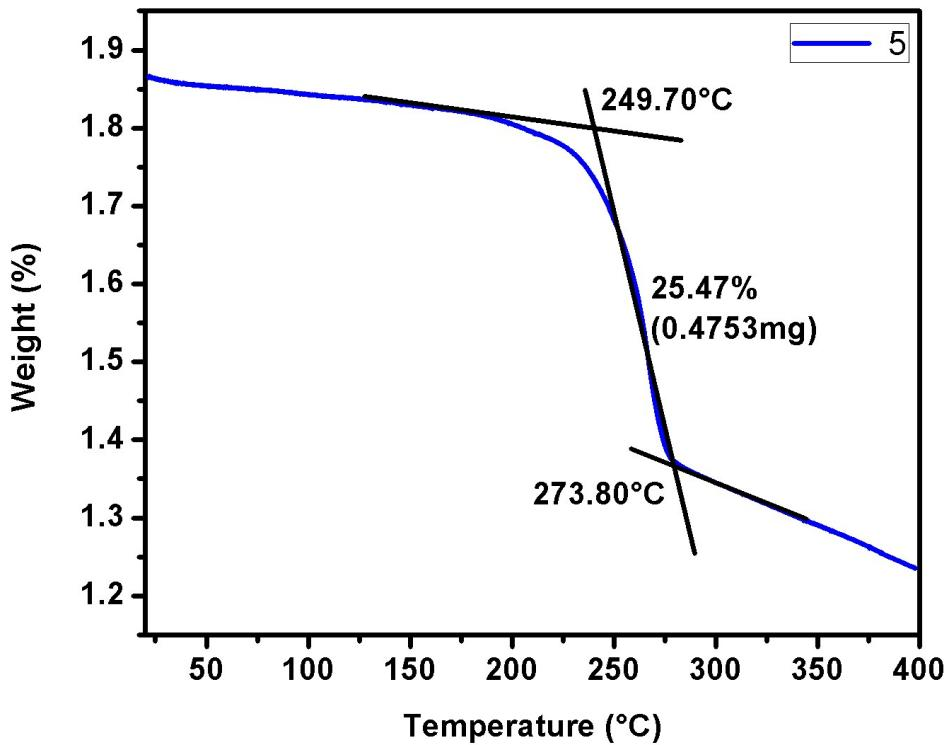
**Figure S22.** TGA thermogram of **5** with heating rate at 5 °C per min.
