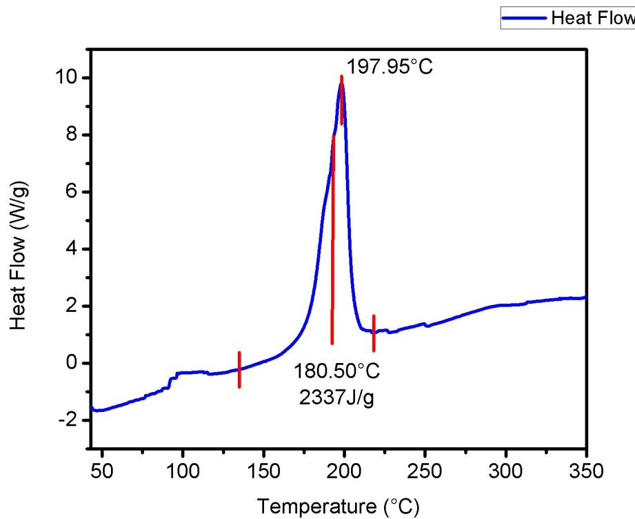
**Figure S18.** DSC thermogram of **3** with heating rate at 10 °C per min.
