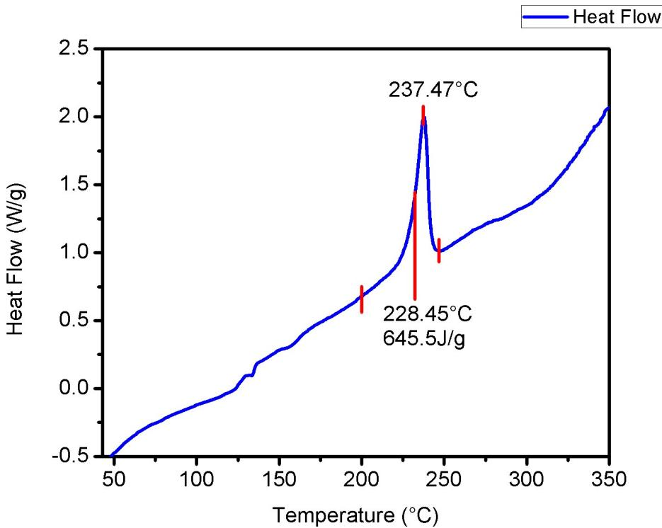
Figure S15. DSC thermogram of **2** with heating rate at 10 °C per min.
