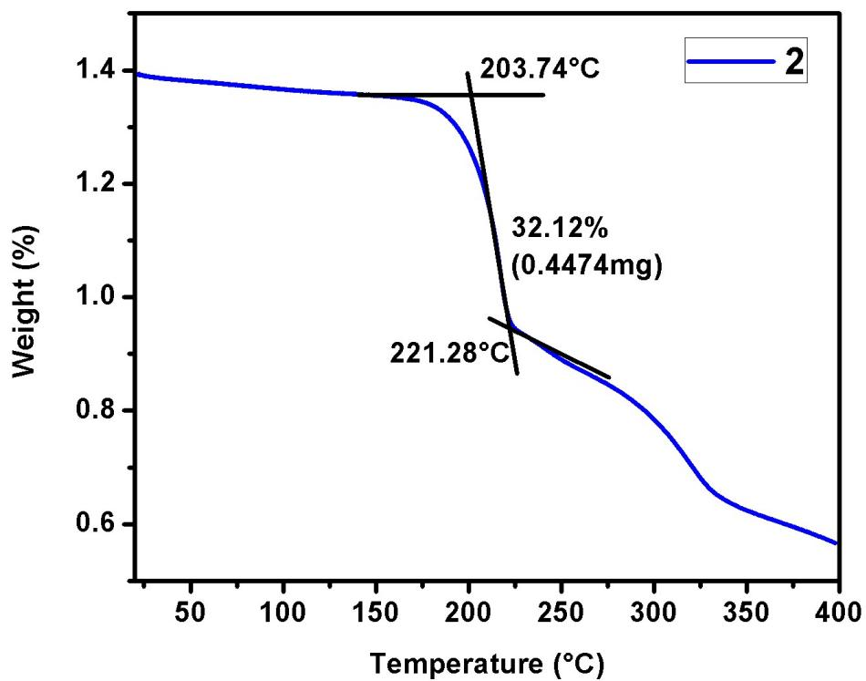
**Figure S16.** TGA thermogram of **2** with heating rate at 5 °C per min.
