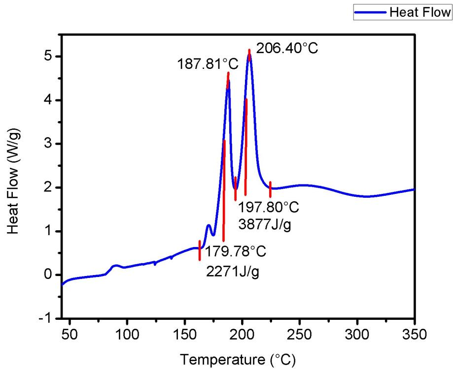
**Figure S17.** DSC thermogram of **3** with heating rate at 5 °C per min.
