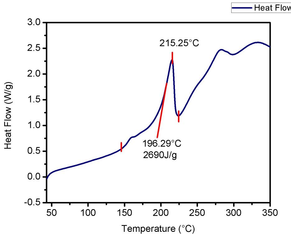
Figure S14. DSC thermogram of **2** with heating rate at 5 °C per min.
