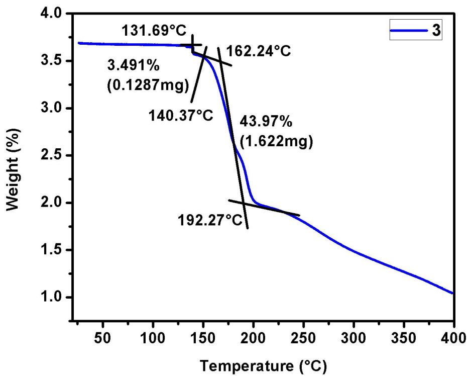
**Figure S19.** TGA thermogram of **3** with heating rate at 5 °C per min.
