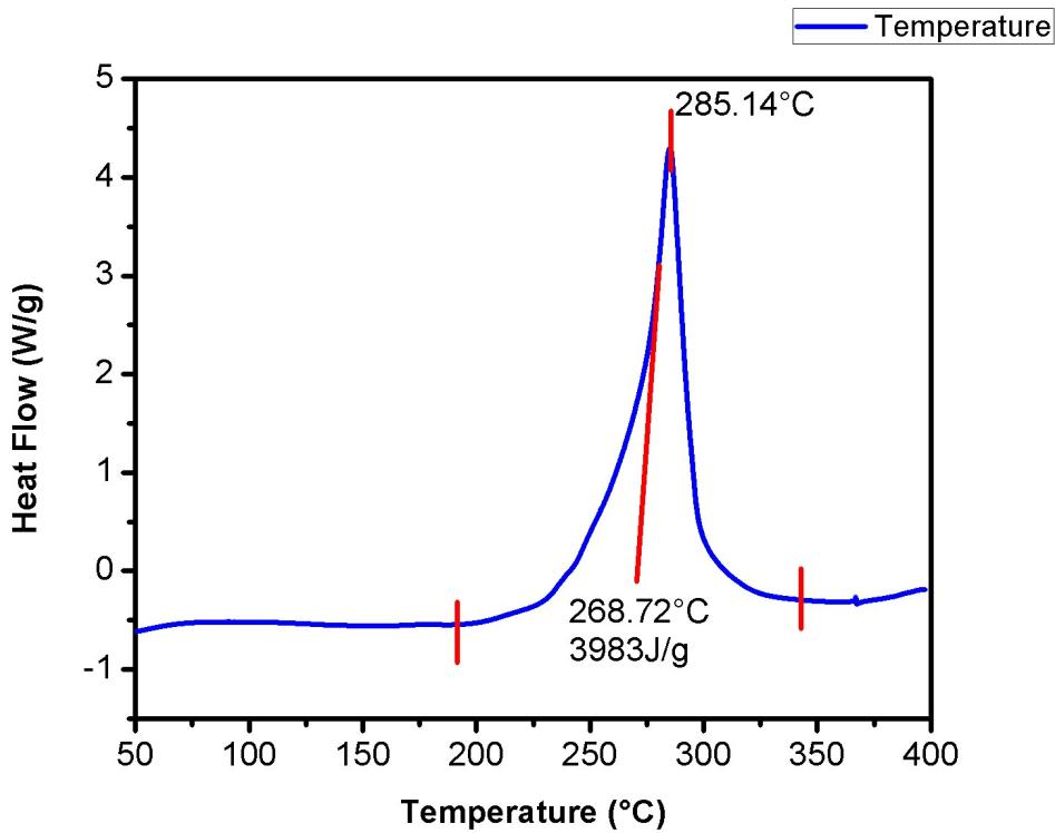
**Figure S21.** DSC thermogram of **5** with heating rate at 10 °C per min.
