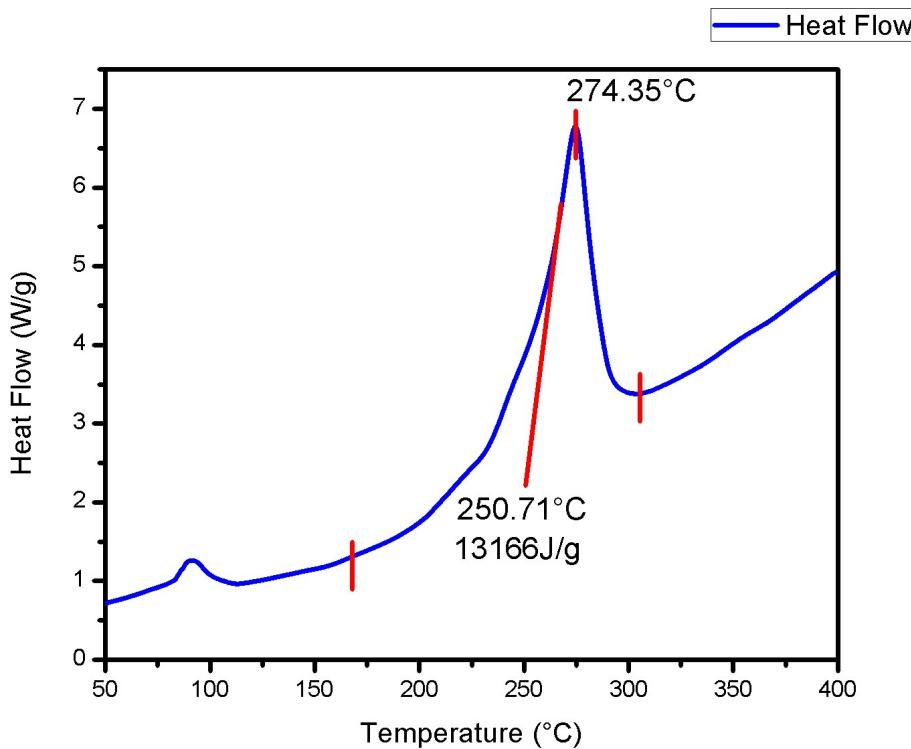
**Figure S20.** DSC thermogram of **5** with heating rate at 5 °C per min.
