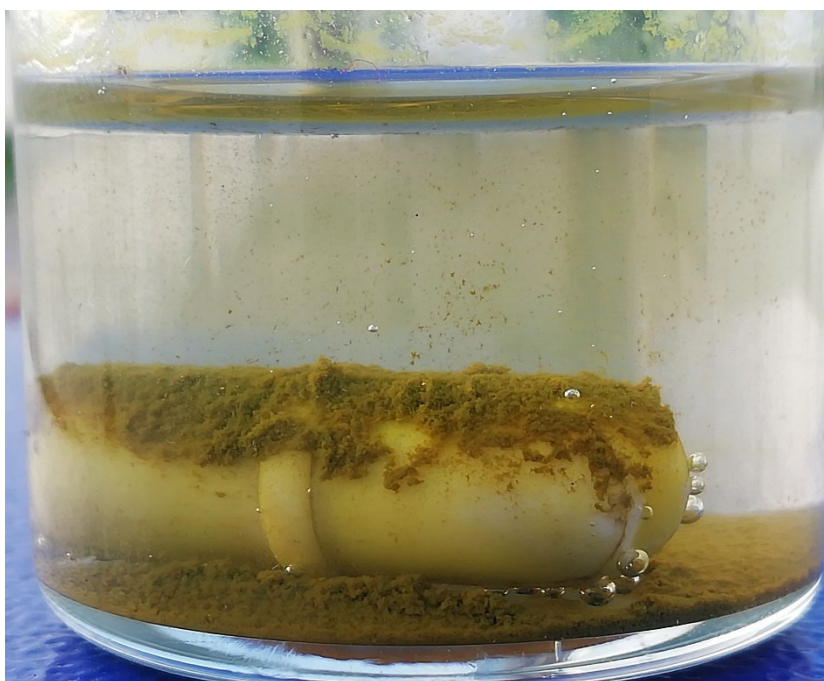
Figure S15: (a) Long-term stability of the optimized CdS/SnS 2 -WS 2 nanocomposite under continuous photo-irradiation (b) Digital photograph of the hydrogen bubbles during the photocatalytic experiment
