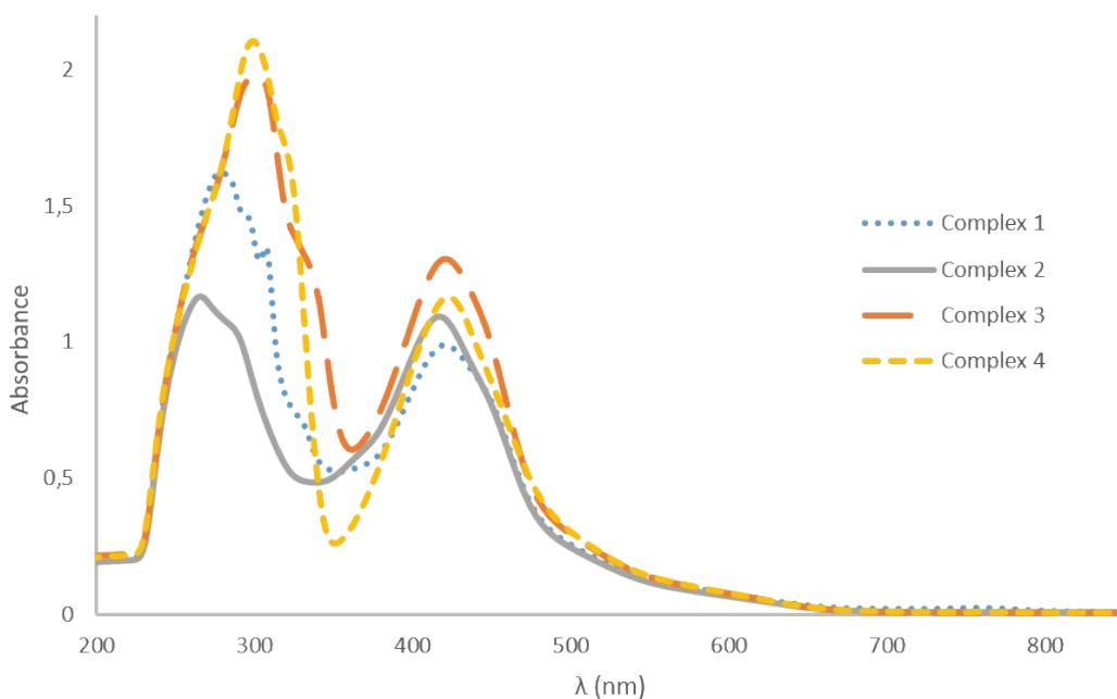
Figure S46. Experimental UV/Vis spectra of the different complexes under study in  $\text{CH}_2\text{Cl}_2$  at  $6 \cdot 10^{-5}$  M.
