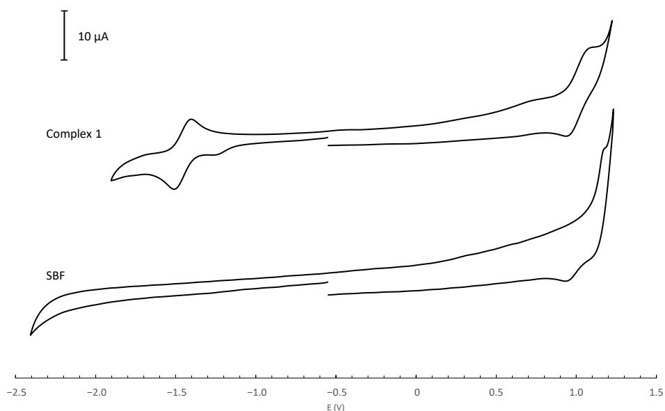
Figure S47. Cyclic voltammograms of 1mM solutions of complex **1** and SBF in  $\text{CH}_2\text{Cl}_2$ , with 0.1 M  $\text{TBAPF}_6$  as supporting electrolyte. Scan rate: 0.2 V/s
