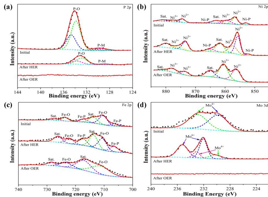
**Fig. S14.** XPS high-resolution spectrum before and after HER/OER of NiMo-Fe-2-P.
