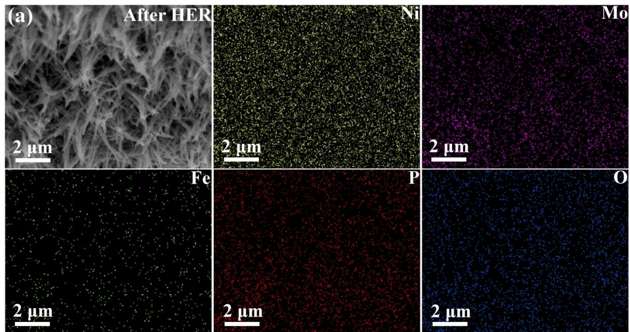
**Fig. S13.** Morphology and element distribution of NiMo-Fe-2-P after HER test.
