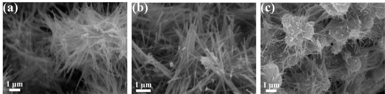
**Fig. S4.** SEM images of (a) NiMo-P; (b) NiMo-Fe-1-P; (c) NiMo-Fe-3-P.
