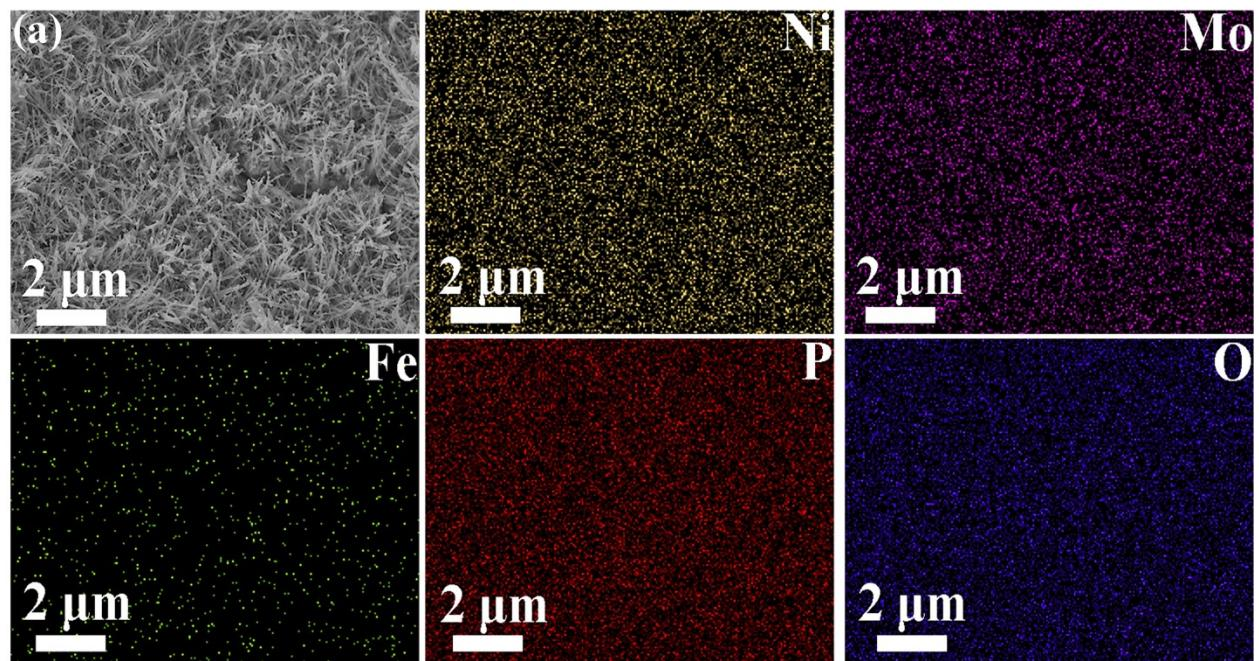
**Fig. S11.** Morphology and element distribution of NiMo-Fe-2-P.
