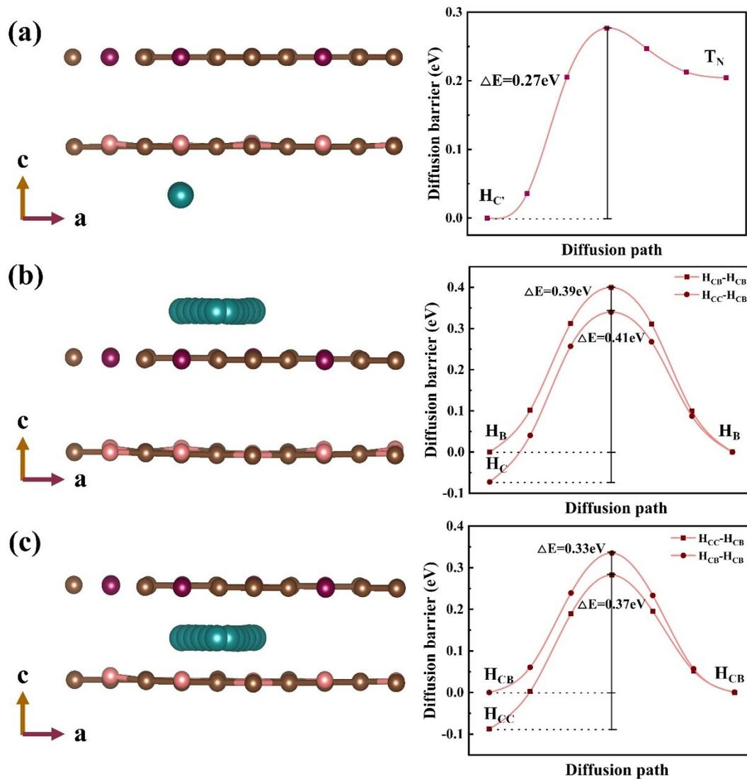
Fig. S6 Front view of migration path and energy barrier of Li diffusion (a) on the outside of  $C_3N$  of the  $C_3N/C_3B$  heterostructure ( $Li/C_3N/C_3B$ ); (b) on the outside of  $C_3B$  of the  $C_3N/C_3B$  heterostructure ( $C_3N/C_3B/Li$ ); (c) on the interlayer of  $C_3N/C_3B$  heterostructure ( $C_3N/Li/C_3B$ ).
