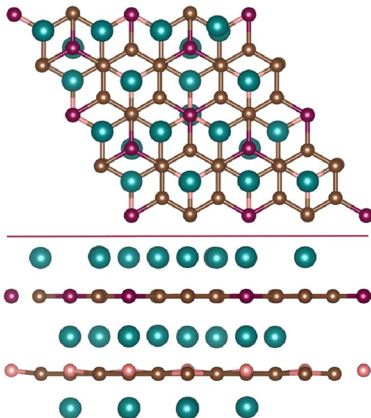
Fig. S4. Top and side views of the maximum possible Li storage in C<sub>3</sub>N/C<sub>3</sub>B heterostructure.
