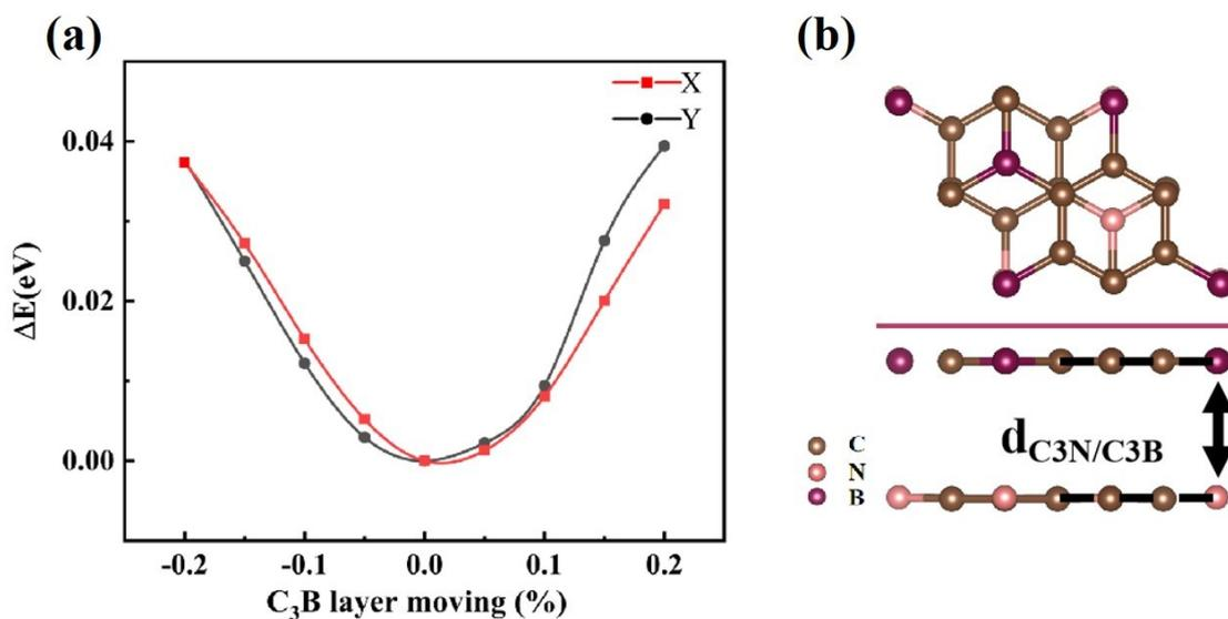
Fig. S1. (a) Energy as a function of C<sub>3</sub>B moving relative to C<sub>3</sub>N of C<sub>3</sub>N/C<sub>3</sub>B along with X and Y directions. (b) The most stable structure in which C<sub>3</sub>B's relatively moving ratio is 0.
