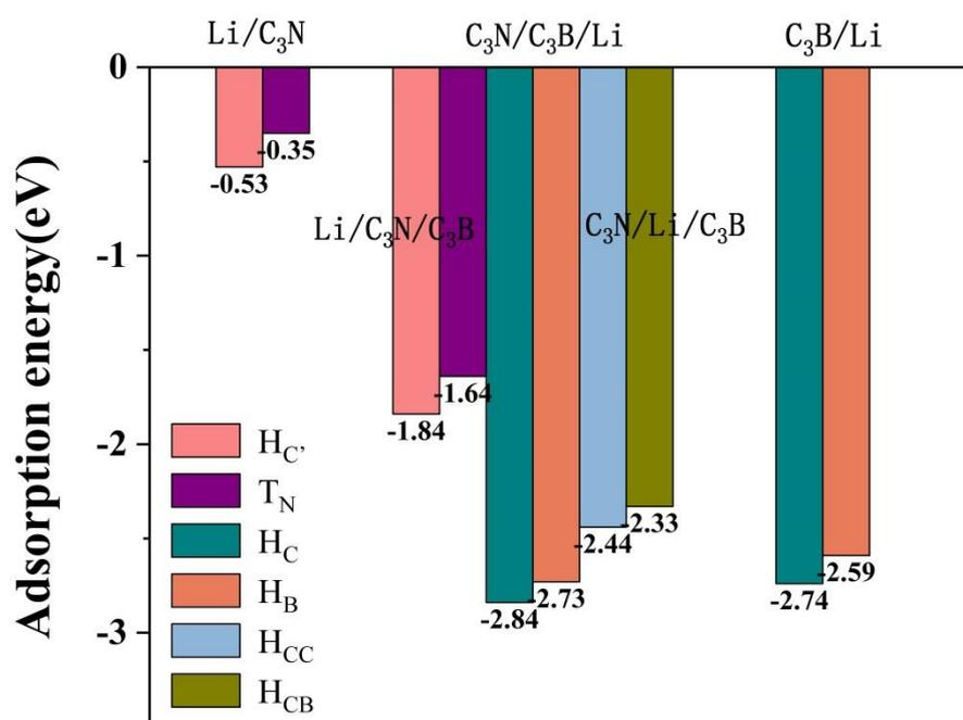
Fig. S3. The adsorption energy of Li adsorbs on C<sub>3</sub>N/C<sub>3</sub>B heterostructure.
