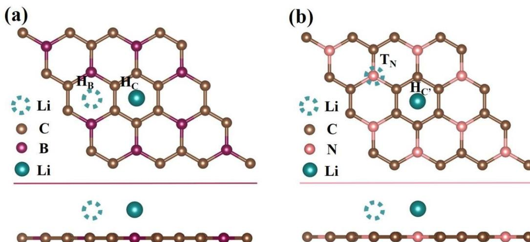
Fig. S2. Top and side views of the Li adsorption sites on the C<sub>3</sub>B and C<sub>3</sub>N monolayer (Li/C<sub>3</sub>B, Li/C<sub>3</sub>N). H<sub>C</sub> and H<sub>B</sub> sites are on the C<sub>3</sub>B, and H<sub>C'</sub> and T<sub>N</sub> sites are on the C<sub>3</sub>N.
