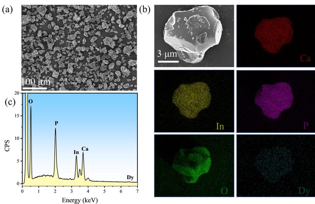
**Figure S4.** SEM image (a), EDS elemental mappings (b), and EDS spectrum (c) of  $C_{1-x}IP: 0.03Dy^{3+}$  sample.
