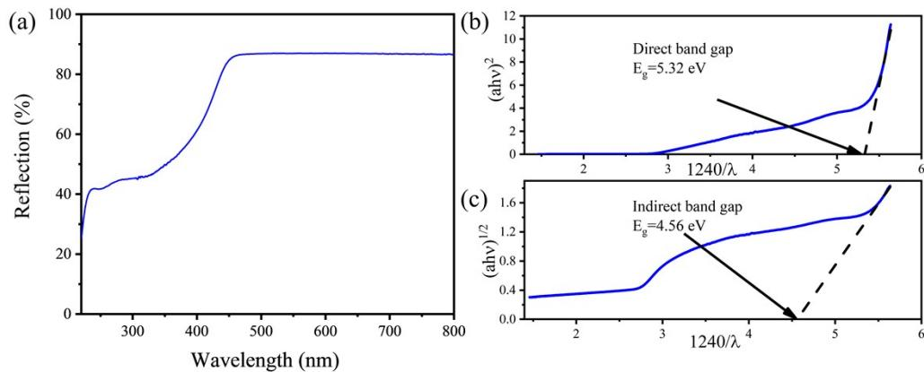
**Figure S2.** The diffuse reflectance spectra (a), extrapolation of the direct band gap (b) and indirect band gap (c) of CIP.
