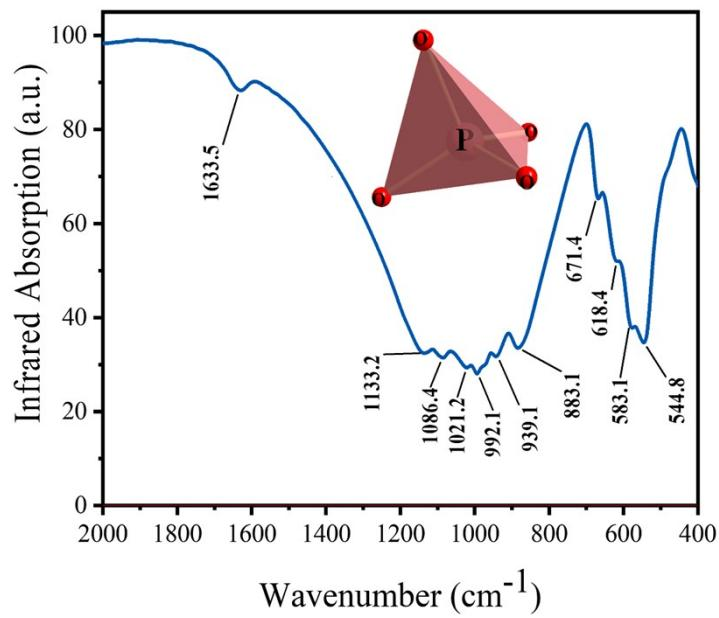
**Figure S1.** The Infrared spectroscopy of CIP from 400 to 2000  $\text{cm}^{-1}$ .
