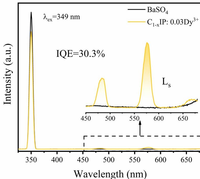
**Figure S5.** Excitation line of  $BaSO_4$  and emission spectrum for  $C_{1-x}IP: 0.03Dy^{3+}$  phosphor.
