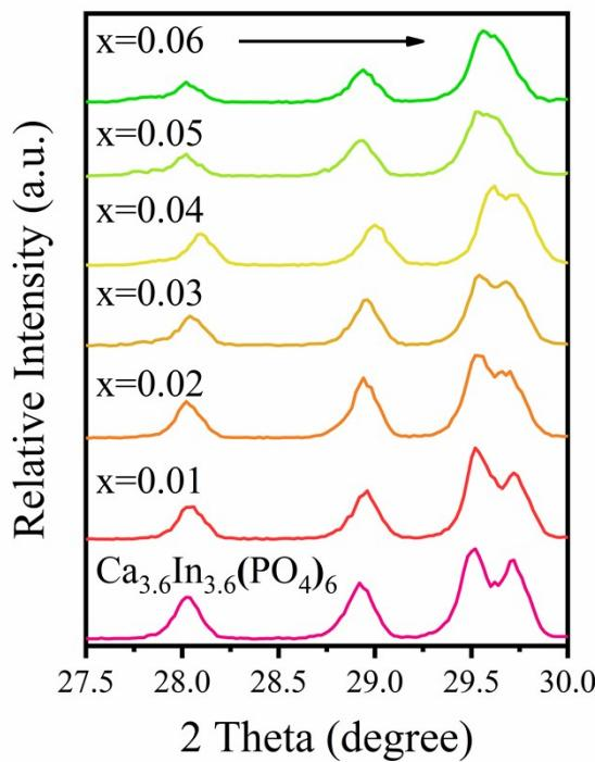
**Figure S3.** The XRD magnification between  $27.5^\circ$  and  $30^\circ$  for  $C_{1-x}IP: xDy^{3+}$ .
