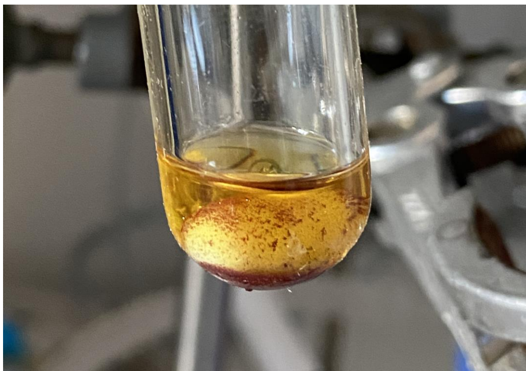
Figure S44: Image of the reddish residue obtained after reacting \text{DipTerP}(\text{PMe}_3) with 1 eq \text{SeO}_2 in \text{C}_6\text{H}_6 at 80 °C over a period of 16 h.
