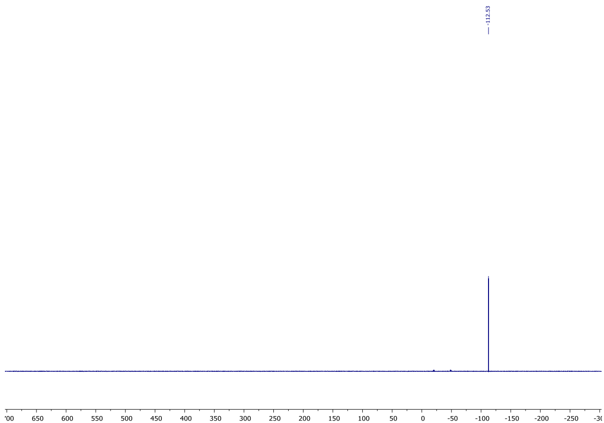
Figure S18: ^{31}\text{P}\{^1\text{H}\} NMR of 1:MesTer (given in ppm, \text{C}_6\text{D}_6 , 122 MHz, 298K).
