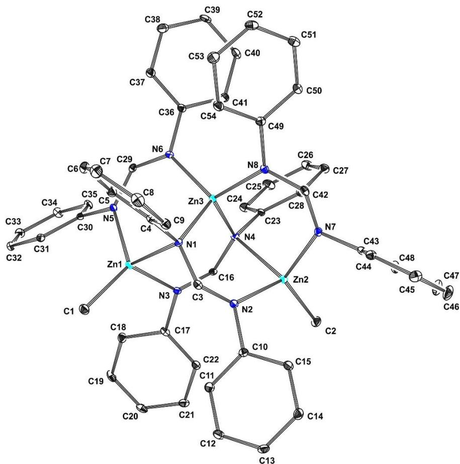
**Fig. S27.** The molecular structure of **1<sup>Me</sup>** with thermal ellipsoids set at 30% probability. Hydrogen atoms have been omitted for clarity.
