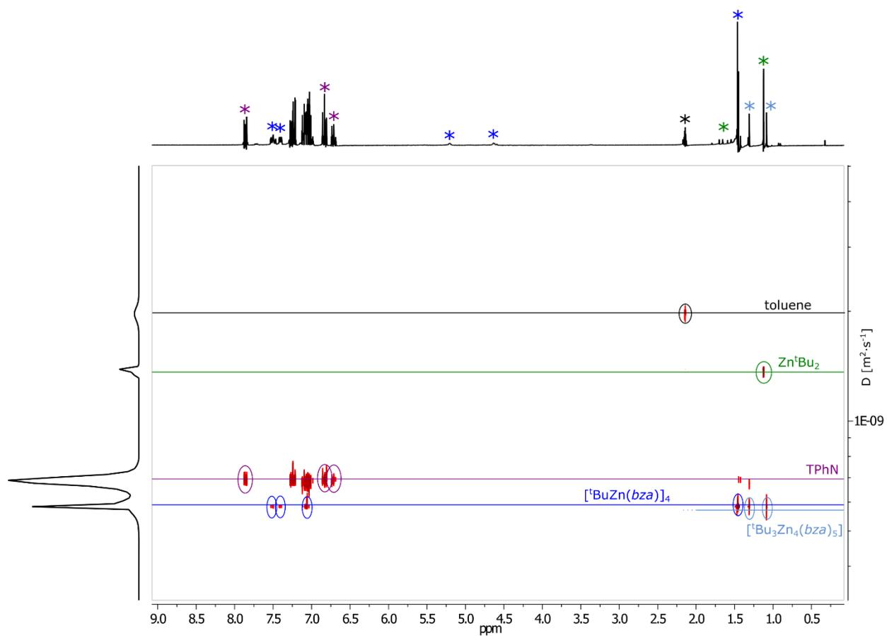
**Fig. S26.** 2D DOSY-NMR spectrum of **3** in  $d_8$ -toluene (signals used to estimate MW are marked with asterisks).
