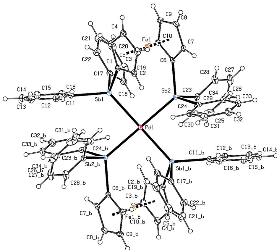
**Figure S18** PLATON plot of the molecular structure of **17b**-Me<sub>2</sub>CO showing 30% probability ellipsoids (the solvent molecule and the counter ion were omitted for clarity)
