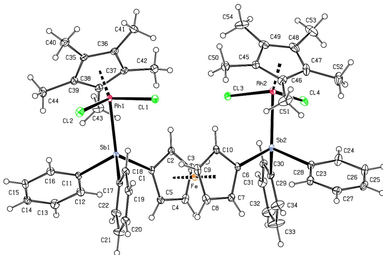
**Figure S12** PLATON plot of the molecular structure of **11**·2CH<sub>2</sub>Cl<sub>2</sub> showing 30% probability ellipsoids (the solvent molecules were omitted for clarity)
