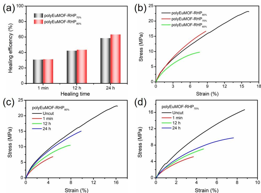
**Fig. S9.** (a) Self-healing efficiency of the polyEuMOF-RHP membranes with different amount of RHP healed at 25 °C for different time periods. (b) The stress-strain curve of polyEuMOF-RHP. The stress-strain curves of the polyEuMOF-RHP<sub>80%</sub> (c) and polyEuMOF-RHP<sub>70%</sub> (d) self-healed at 25 °C for different time.
