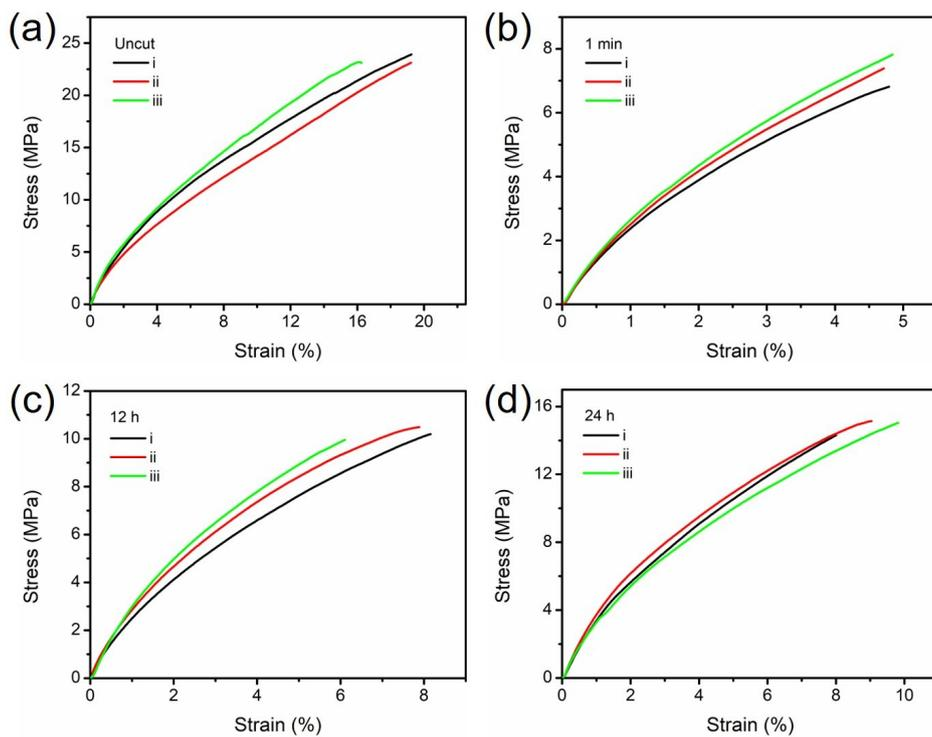
**Fig. S16.** The stress-strain curves of the polyEuMOF-RHP<sub>80%</sub> (a) and self-healed at 25 °C for 1 min (b), 12 h (c) and 24 h (d).
