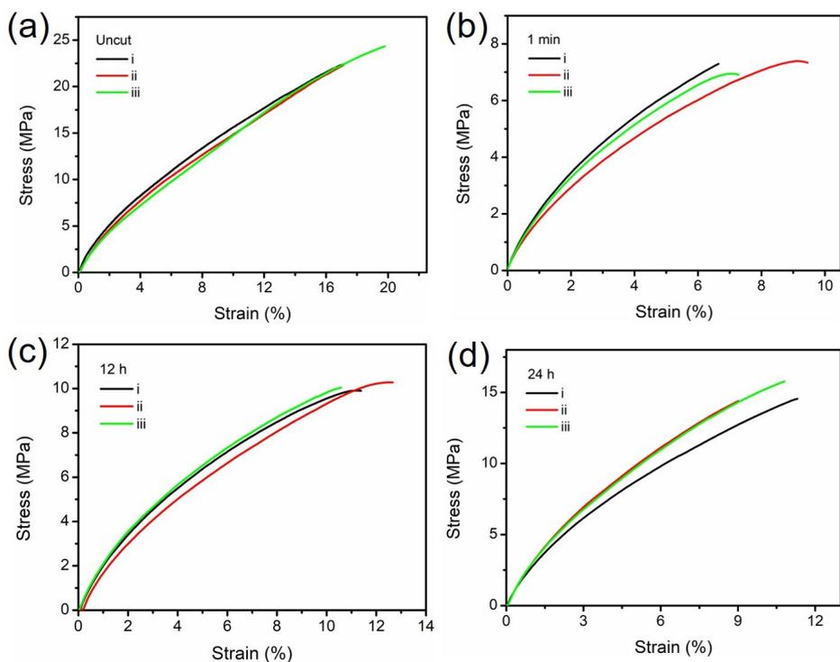
**Fig. S17.** The stress-strain curves of the polyTbMOF-RHP<sub>80%</sub> (a) and self-healed at 25 °C for 1 min (b), 12 h (c) and 24 h (d).
