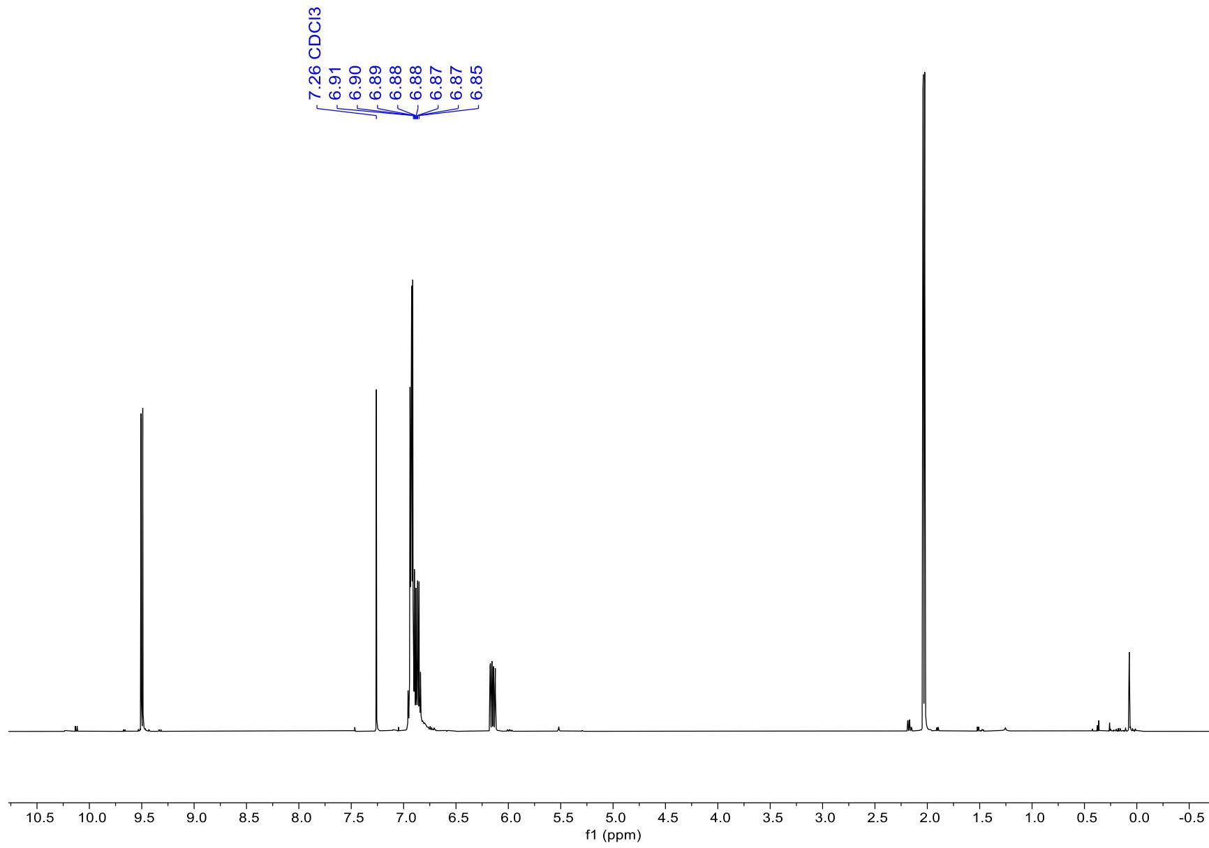
Figure S49:  $^1\text{H}$  NMR (500.2 MHz,  $\text{CDCl}_3$ ) spectrum of *trans*-crotonaldehyde and  $\text{B}(2,4,6\text{-F}_3\text{H}_2\text{C}_6\text{O})_3$  (**7**).
