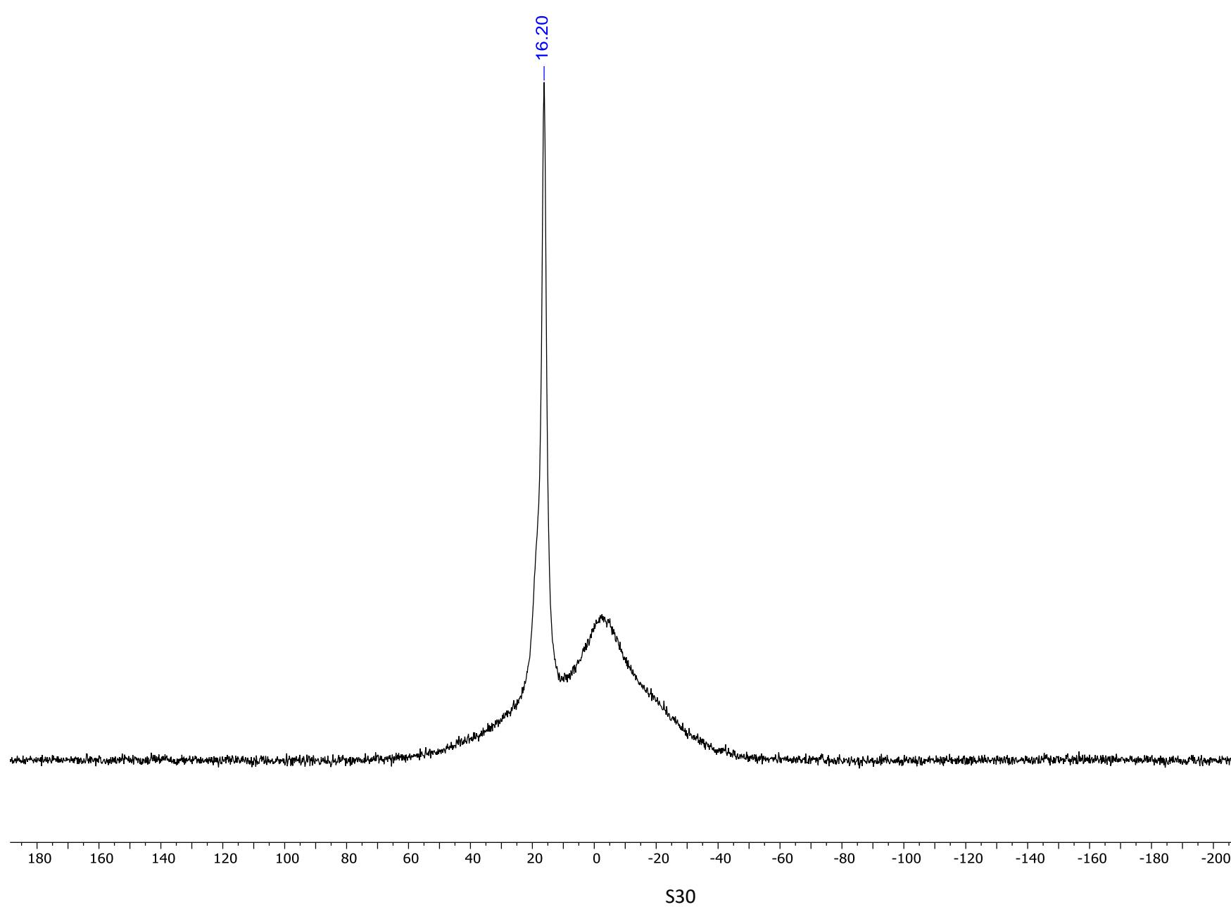
Figure S23:  $^{19}\text{F}$  NMR (376.5 MHz,  $\text{CDCl}_3$ ) spectrum of tris(2,3,4-trifluorophenyl)borate (**6**).
