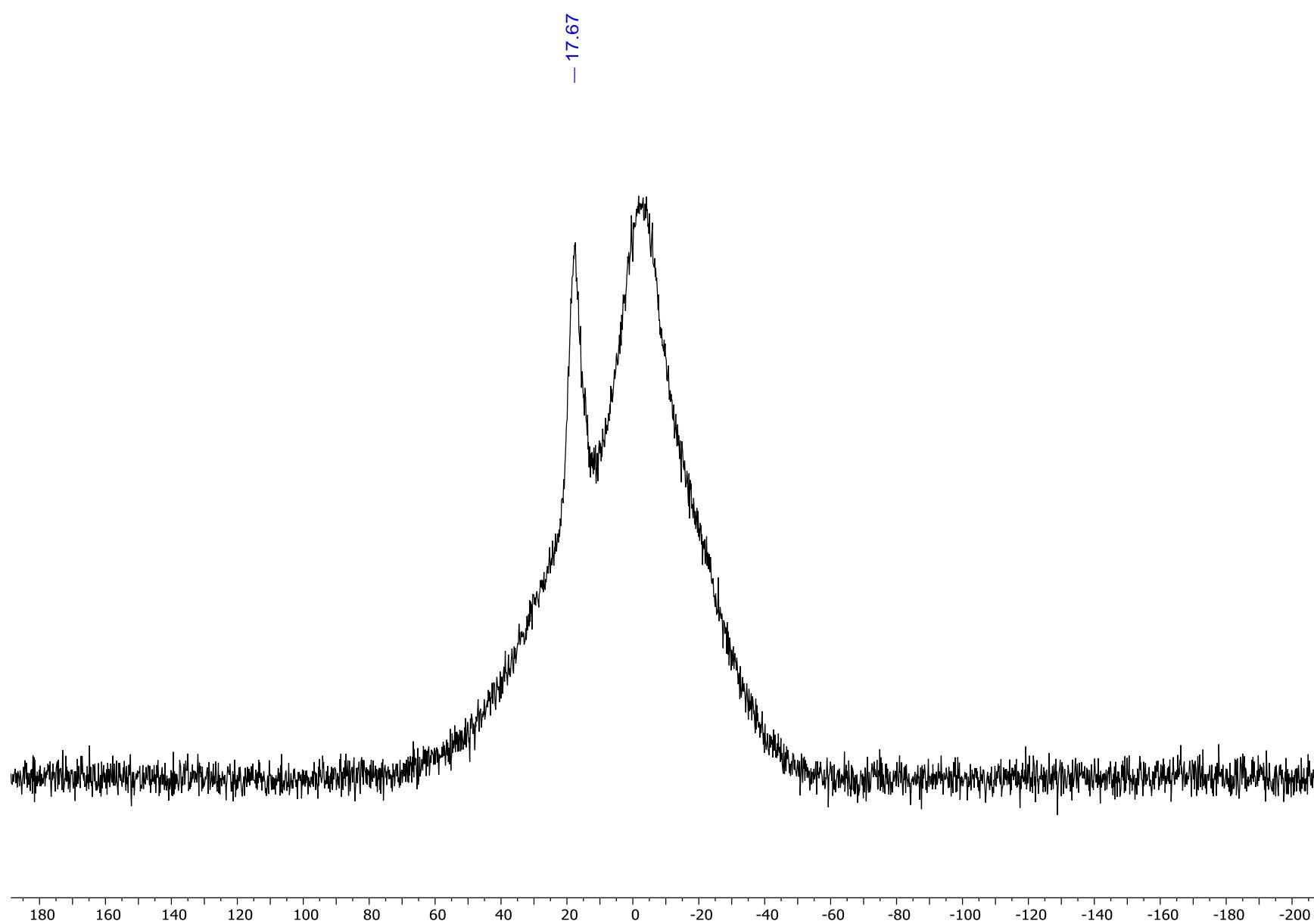
Figure S27:  $^{19}\text{F}$  NMR (470.2 MHz,  $\text{CDCl}_3$ ) spectrum of tris(2,4,6-trifluorophenyl)borate (**7**).
