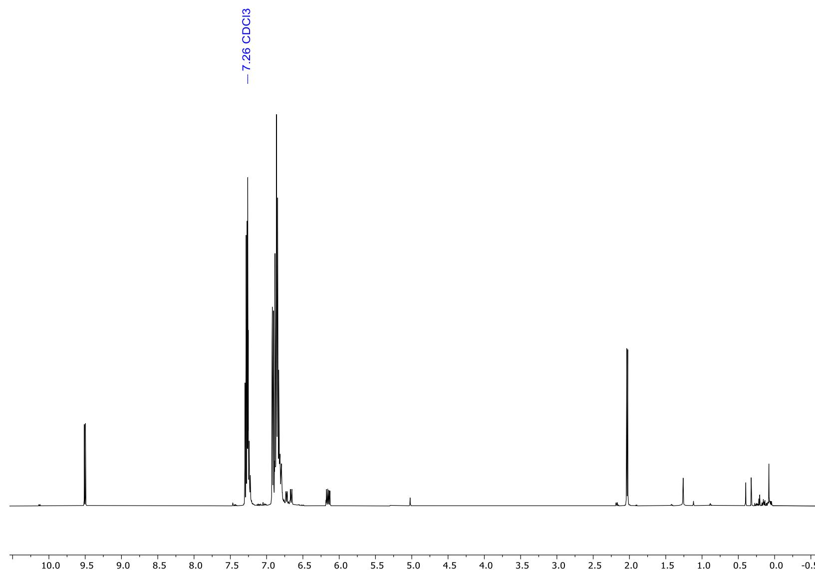
Figure S45:  $^1\text{H}$  NMR (500.2 MHz,  $\text{CDCl}_3$ ) spectrum of *trans*-crotonaldehyde and  $\text{B}(\text{4-F}_1\text{H}_4\text{C}_6\text{O})_3$  (**3**).
