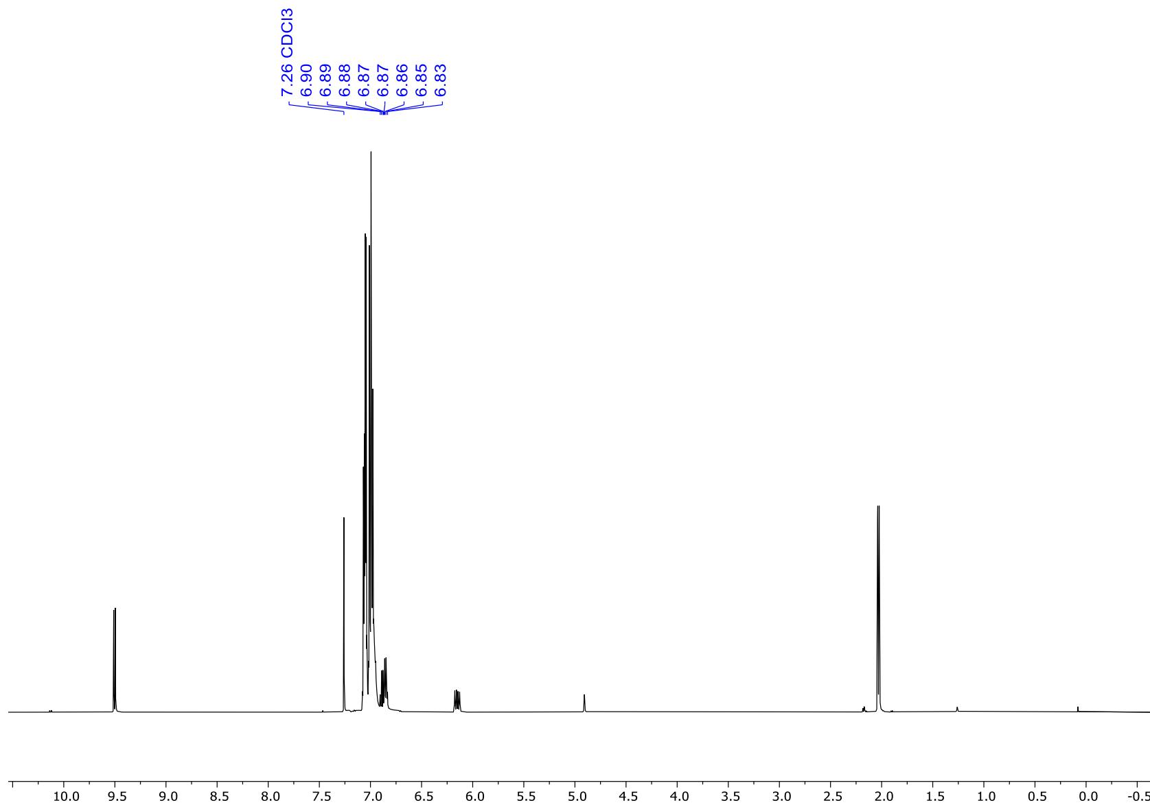
Figure S46:  $^1\text{H}$  NMR (500.2 MHz,  $\text{CDCl}_3$ ) spectrum of *trans*-crotonaldehyde and B(2,4-F<sub>2</sub>H<sub>3</sub>C<sub>6</sub>O) (**4**).
