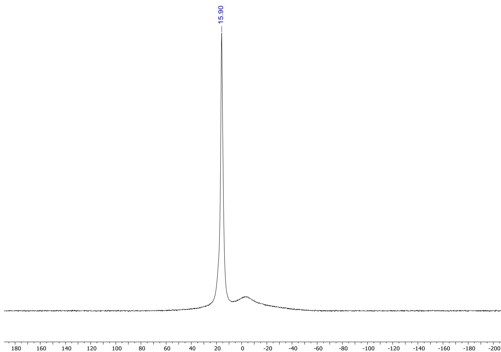
Figure S7:  $^{19}\text{F}$  NMR (376.5 MHz,  $\text{CDCl}_3$ ) spectrum of tris(3-fluorophenyl)borate (**2**).
