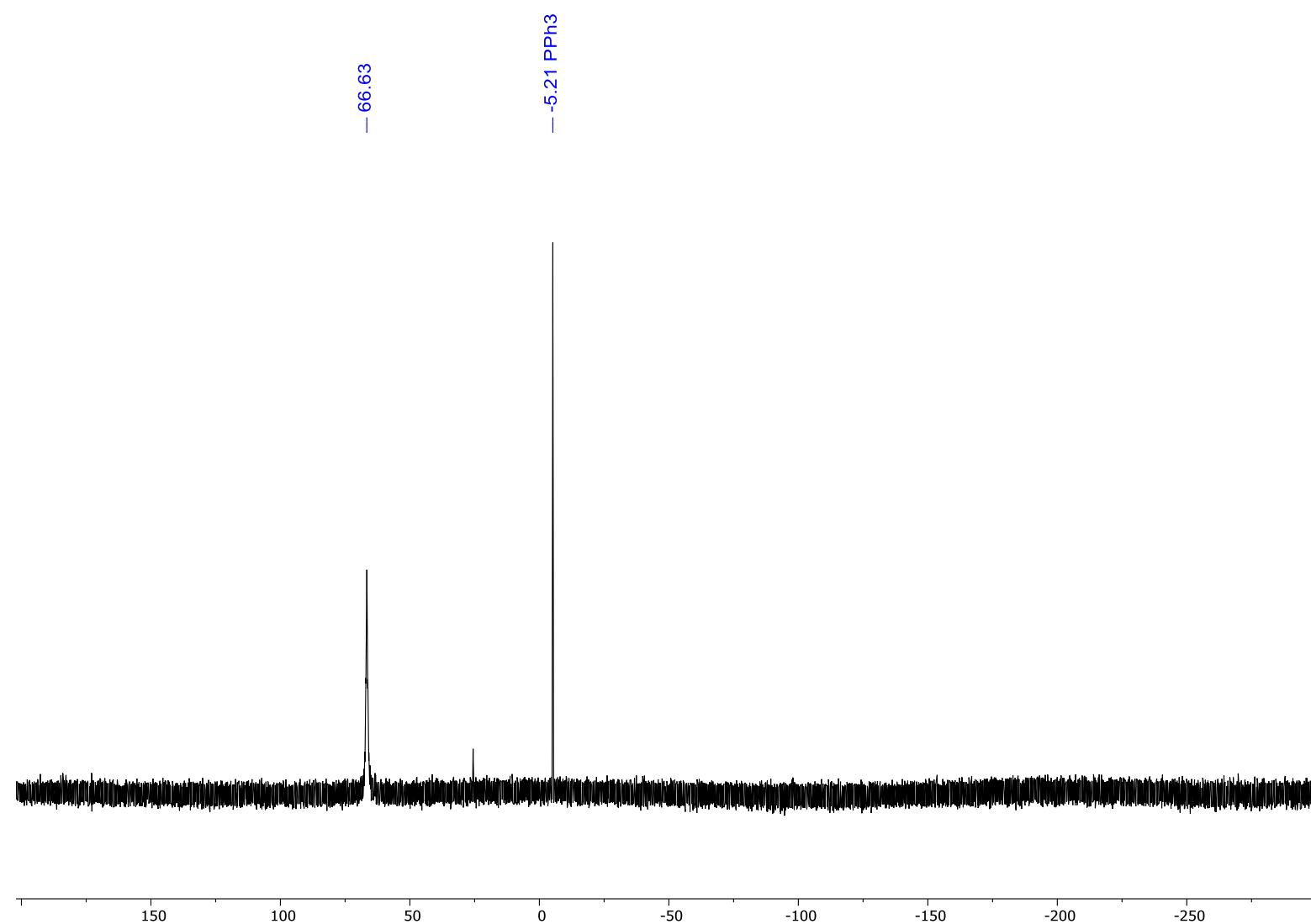
Figure S37:  $^{31}\text{P}$  NMR (202.5 MHz,  $\text{CDCl}_3$ ) spectrum of  $\text{Et}_3\text{PO}$  and  $\text{B}(2,4\text{-F}_2\text{H}_3\text{C}_6\text{O})_3$  (**4**).
