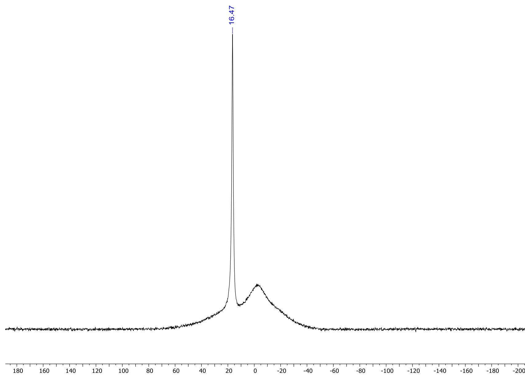
Figure S3: **<sup>19</sup>F NMR** (376.5 MHz, CDCl<sub>3</sub>) spectrum of tris(2-fluorophenyl)borate (**1**).
