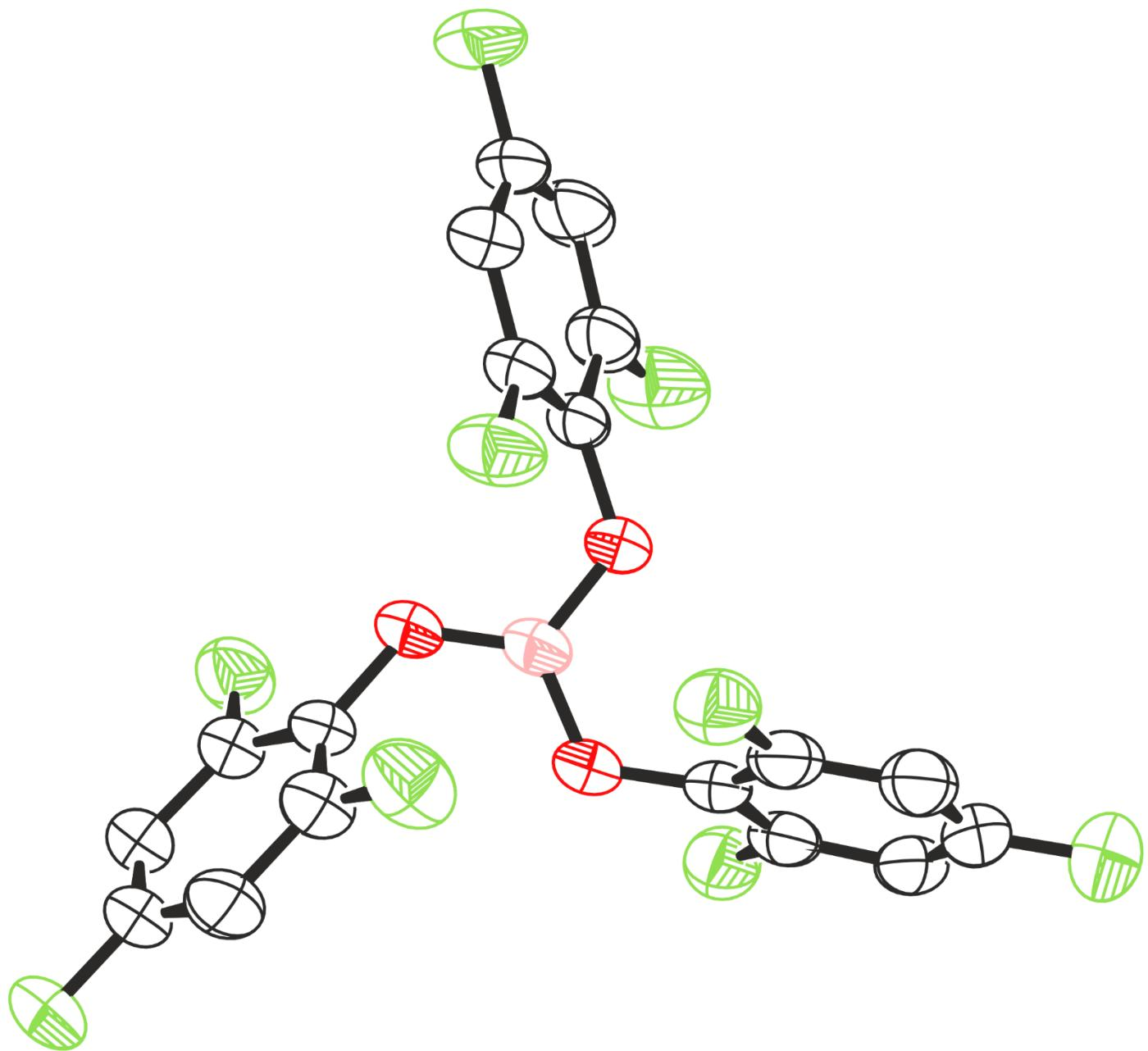
Figure S65. Solid-state structure of compound **7**, side view, thermal ellipsoids drawn at 50% probability. H atoms omitted for clarity. C atoms in black, O in red, B in pink, F in green.
