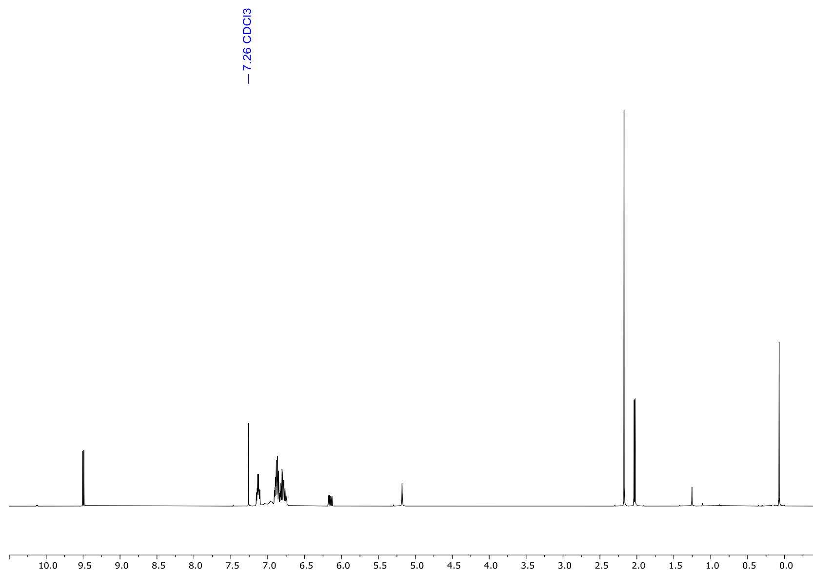
Figure S47:  $^1\text{H}$  NMR (500.2 MHz,  $\text{CDCl}_3$ ) spectrum of *trans*-crotonaldehyde and  $\text{B}(\text{3,5-F}_2\text{H}_3\text{C}_6\text{O})_3$  (**5**).
