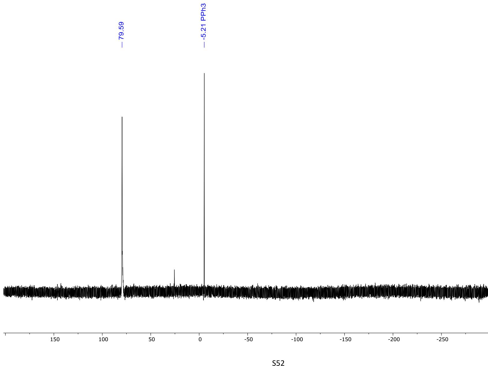
Figure S41:  $^{31}\text{P}$  NMR (202.5 MHz,  $\text{CDCl}_3$ ) spectrum of  $\text{Et}_3\text{PO}$  and  $\text{B}(3,4,5\text{-F}_3\text{H}_2\text{C}_6\text{O})_3$  (**8**).
