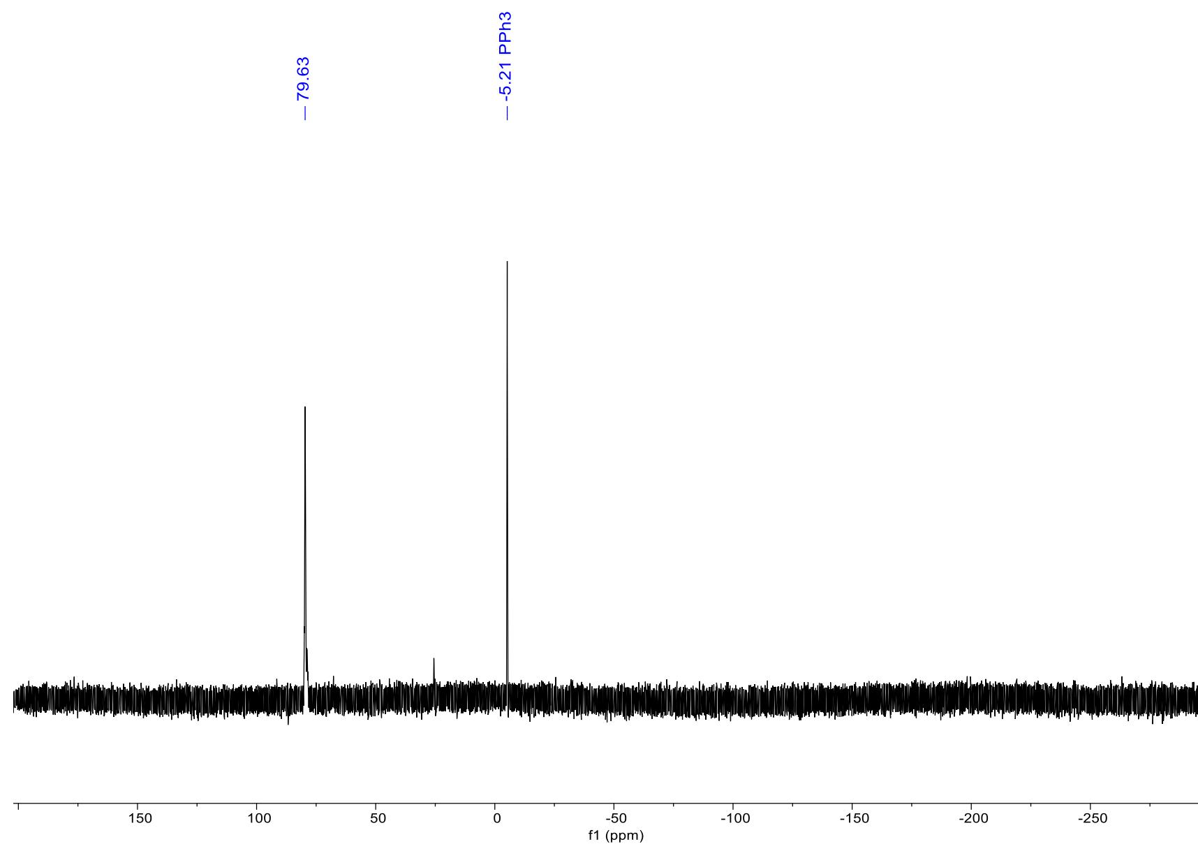
Figure S40:  $^{31}\text{P}$  NMR (202.5 MHz,  $\text{CDCl}_3$ ) spectrum of  $\text{Et}_3\text{PO}$  and  $\text{B}(2,4,6\text{-F}_3\text{H}_2\text{C}_6\text{O})_3$  (**7**).
