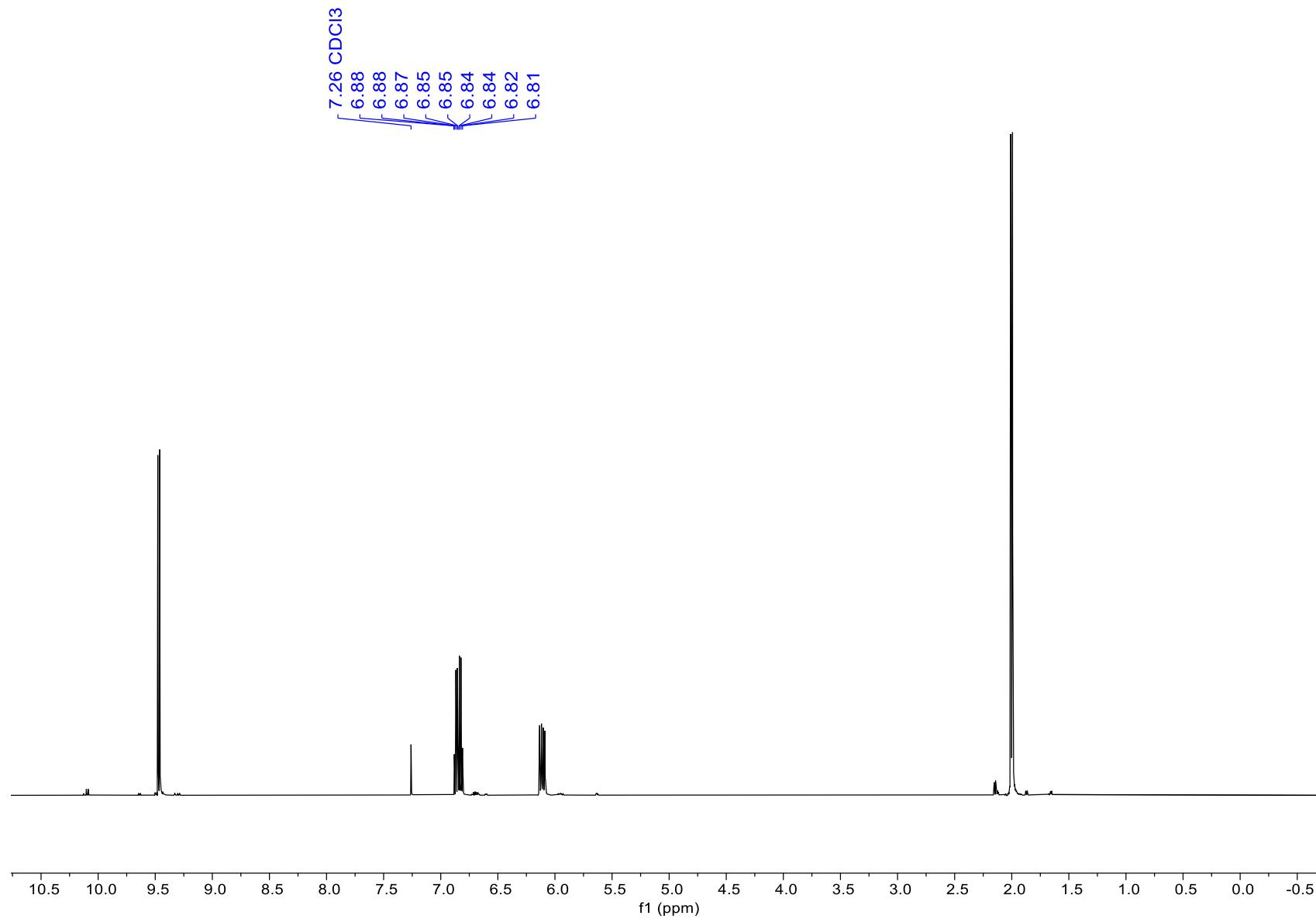
Figure S43:  $^1\text{H}$  NMR (500.2 MHz,  $\text{CDCl}_3$ ) spectrum of *trans*-crotonaldehyde and  $\text{B}(\text{2-F}_1\text{H}_4\text{C}_6\text{O})_3$  (**1**).
