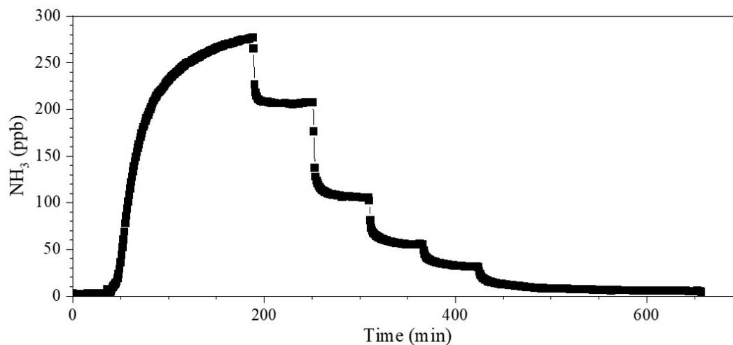
Fig. S1 Calibration of the NH<sub>3</sub> instrument using diluted standard NH<sub>3</sub> and N<sub>2</sub> gas.
