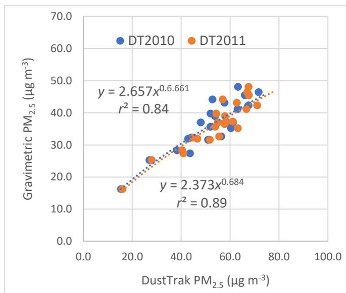
**Fig. ES11.** Scatter plot of co-located gravimetric and time-averaged DustTrak  $\text{PM}_{2.5}$  measurements for the monitor used in this study.
