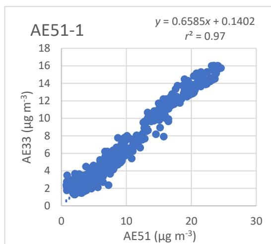
**Fig. ES12.** Scatter plot of co-located eBC measurements from an aethalometer AE33 and the micro-aethalometer AE51 used in this study.
