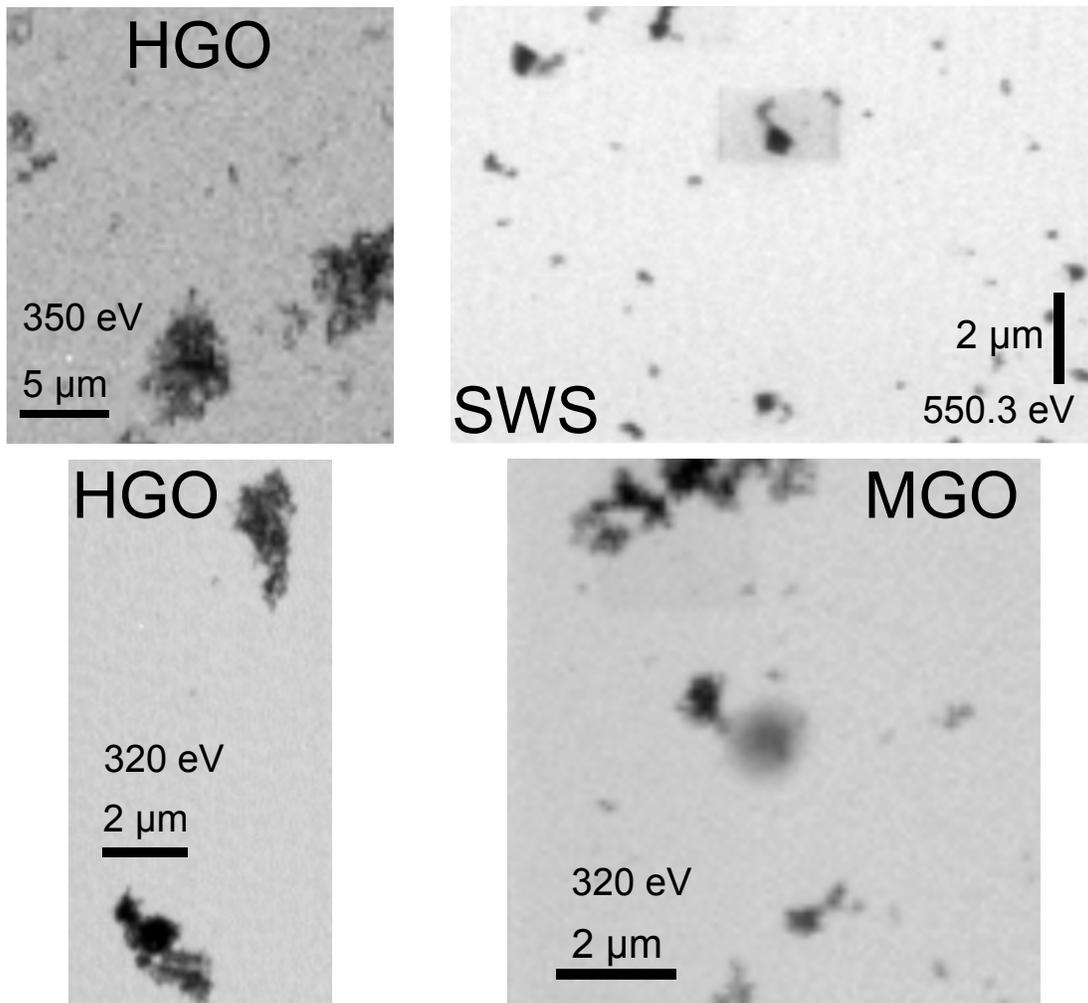
Figure S5: STXM images of exhaust particles for MGO, HGO and SWS.
