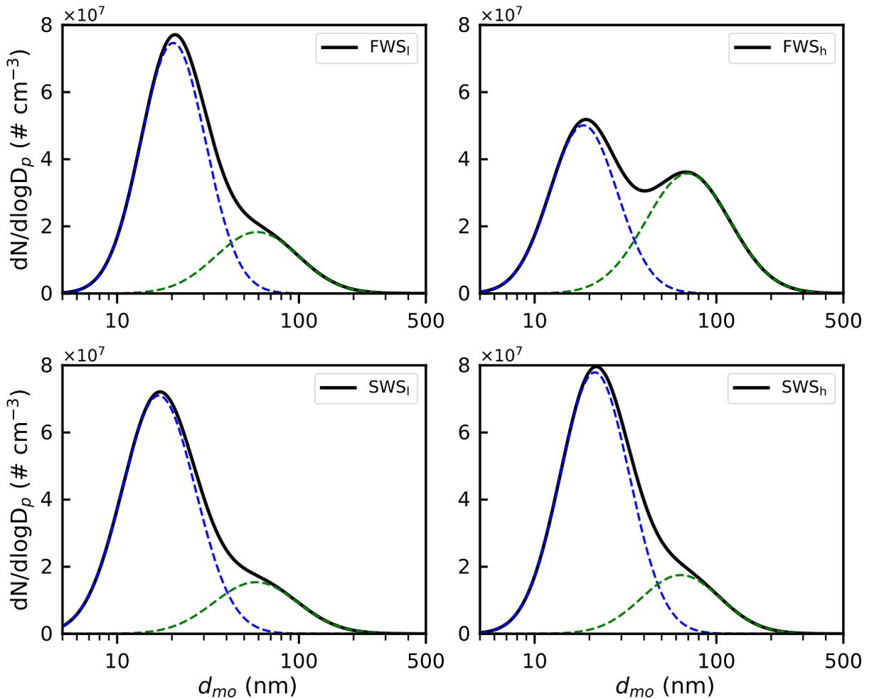
Figure S1: Bimodal lognormal fits of particle size distributions (PSDs) for all four wet scrubber cases from Figure 2 are replotted to illustrate the underlying unimodal distributions.
