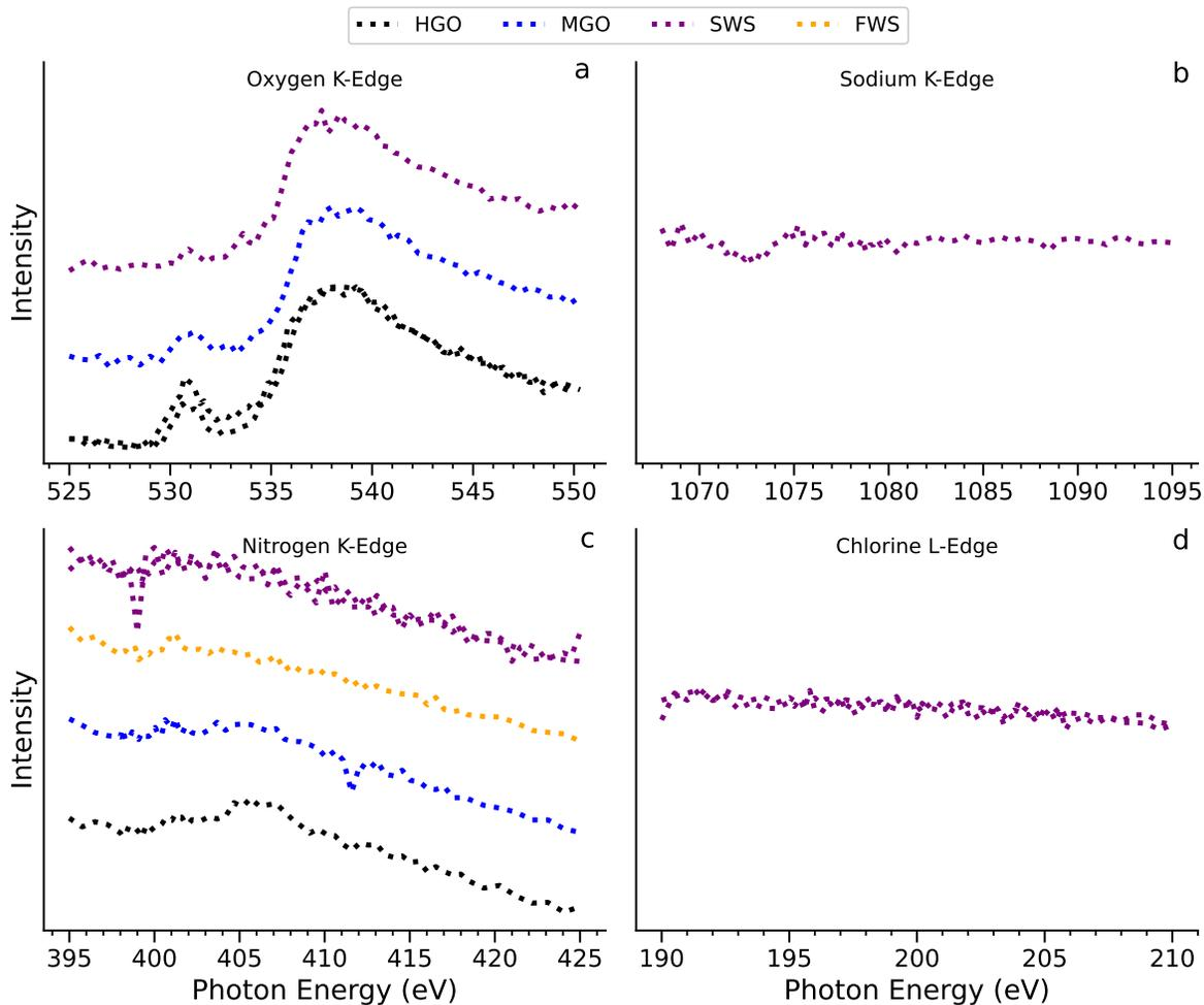
Figure S6: Near-edge X-ray absorption fine structure (NEXAFS) spectra of (a) oxygen, (b) chlorine, (c) nitrogen and (d) chlorine for HGO, MGO, FWS and SWS particles. In panels with more than one case, case-specific spectra have been shifted in their y-positions.
