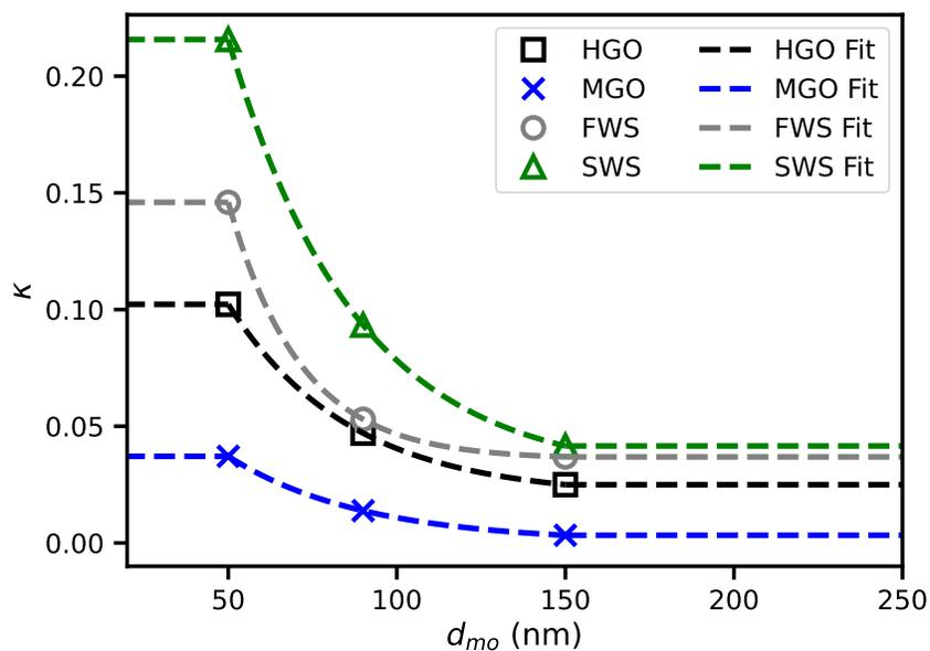
Figure S4: Calculated average  $\kappa$  values for HGO, MGO, FWS and SWS for size-selected particles at  $d_{mo} = 50, 90$  and  $150$  nm represented by markers. Data points were interpolated using least-squares exponential fit functions (Equation S1). For  $d_{mo}$  smaller than  $50$  nm and larger than  $150$  nm, constant  $\kappa$  values equal to the respective threshold values were assumed. Fitted and extrapolated data are represented by dashed lines.
