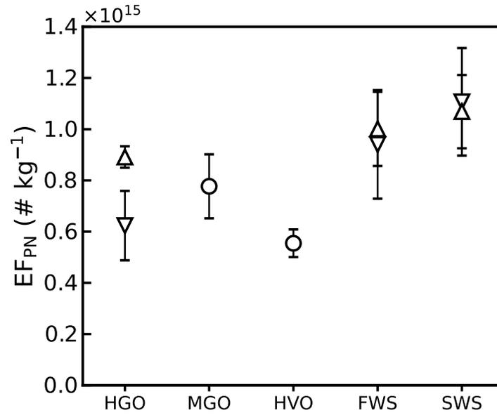
Figure S2: Particle number emission factors ( $EF_{PN}$ ) that were calculated from lognormal least-squares fits (Figure 3) are replotted for better visibility. Error bars represent  $\pm$  two standard deviations. Observed differences in combustion conditions for HGO, FWS and SWS are denoted by downward triangles for relatively low  $CO_2$  concentrations, e.g. HGO<sub>l</sub>, and upward triangles for relatively high  $CO_2$  concentrations, e.g. HGO<sub>h</sub>.
