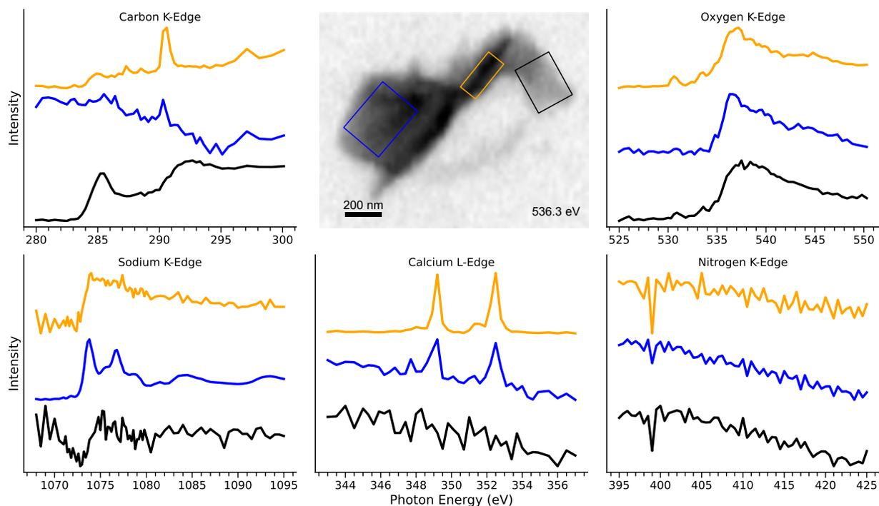
Figure S7: Carbon, oxygen, sodium, calcium and nitrogen Near-edge X-ray absorption fine structure (NEXAFS) spectra of an inhomogeneous SWS particle displayed in the top center panel. Individual spectra correspond to the region marked on the particle image with the respective color. Spectra in each panel have been shifted in their y-positions.
