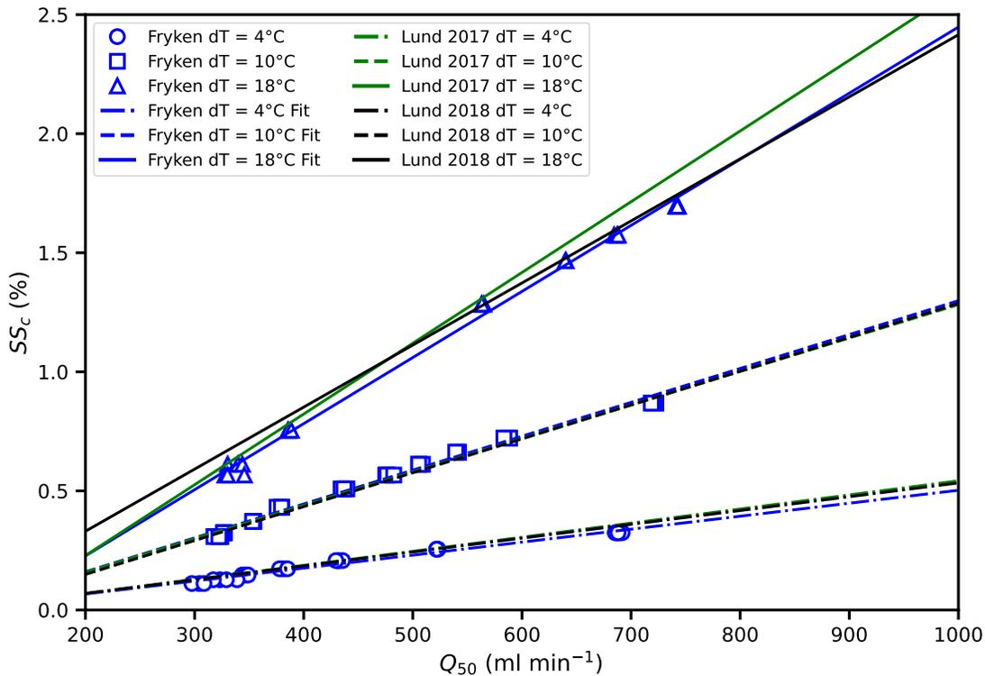
Figure S3: CCNc calibration measurements performed with ammonium sulfate (AS) at  $\Delta T=4$  K, 10 K and 18 K. The calibration data is compared to two previous calibrations conducted at the aerosol science lab at Lund University, Sweden.
