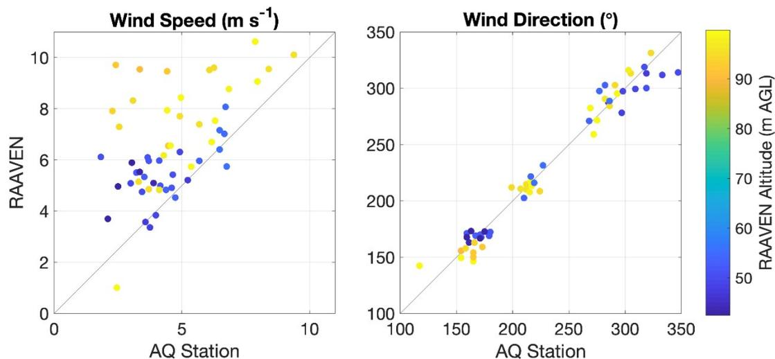
**Figure S9:** Comparison of wind speed and wind direction measured on the RAAVEN with the observations from the air quality station. Color indicates altitude of RAAVEN at the time of measurement. Data were selected when the RAAVEN was within 500 m of the Air Quality Station (mean distance of 300 m).
