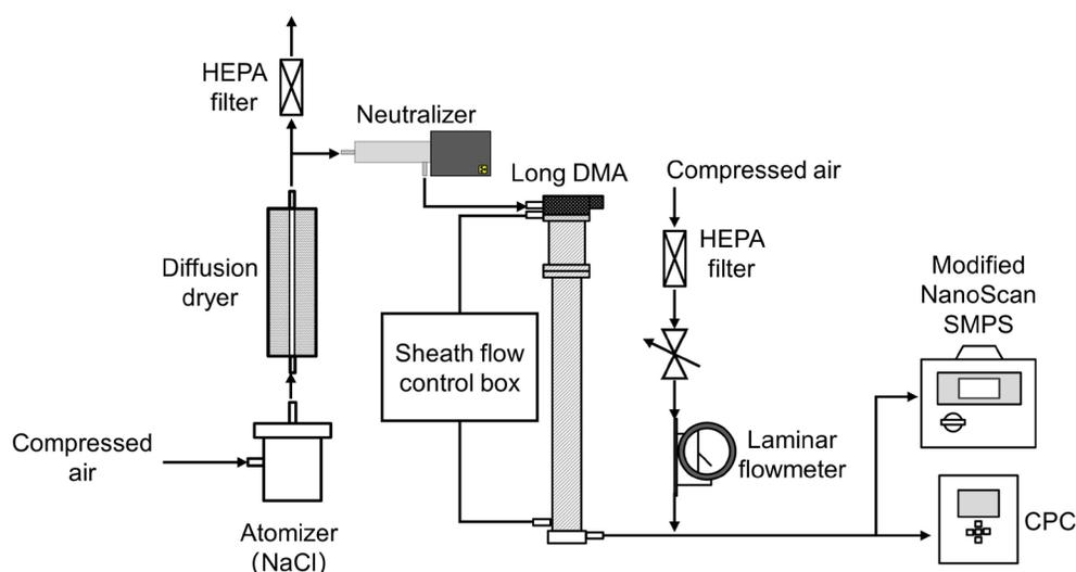
**Figure S1.** Instrument setup for measuring the combined factor of the transfer function, CPC detection efficiency, and penetration efficiency of the modified NanoScan SMPS
