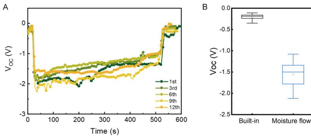
Fig. S19 (A)  $V_{oc}$  of an IPHC device in response to moisture flow at specific cycles. (In each cycle, the device was moisturized to its saturation and then baked to dry.) (B) Stability in terms of built-in voltage and voltage output for 12 cycles.
