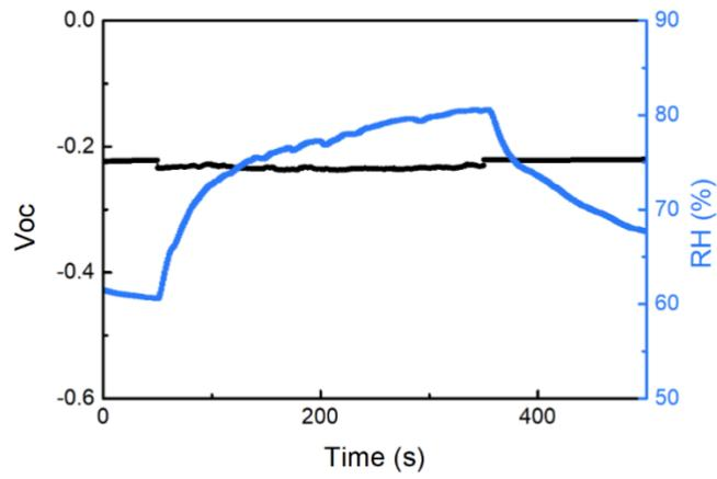
Fig. S12  $V_{oc}$  of an IPHC in response to the change of RH for the entire environmental chamber and corresponding RH.
