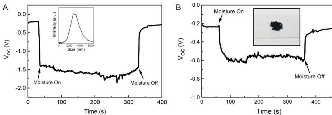
Fig. S16 (A)  $V_{oc}$  of an IPHC device comprising poly(N-isopropylacrylamide) (pNIPAm) and 2-aminoethylmethacrylate hydrochloride (AEMA) co-polymerized hydrogel microparticles (pNIPAm-AEMA) as the moisture absorbent layer. Inset shows the size distribution of as-prepared pNIPAm-AEMA. (B)  $V_{oc}$  of an IPHC device comprising polypyrrole (PPy) hydrogel nanoparticles as the replacement of pNIPAm. Inset shows the digital image of PPy nanoparticles.
