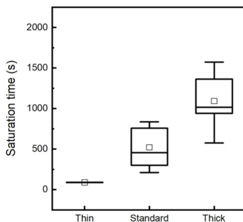
Fig. S5 Saturation time of IPHCs with different layer thickness of pNIPAm.
