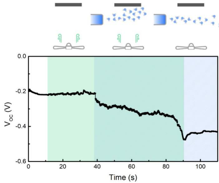
Fig. S14  $V_{oc}$  of an IPHC that was exposed to dry air at a flow rate of  $3.0\text{m s}^{-1}$  from 11s to 90s, and then moisture flow from 39s to 110s. The schematic diagram illustrates the experimental setup where the moisture was driven into the IPHC device by forced convection during 39-90s.
