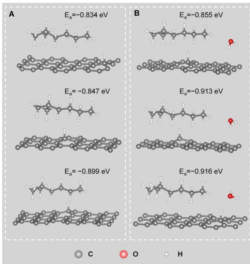
Fig. S9 Adsorption configurations of a H on (A) isoheptane-graft-graphene and (B) isoheptane-graft-graphene with  $H_2O$ , and corresponding adsorption energies.
