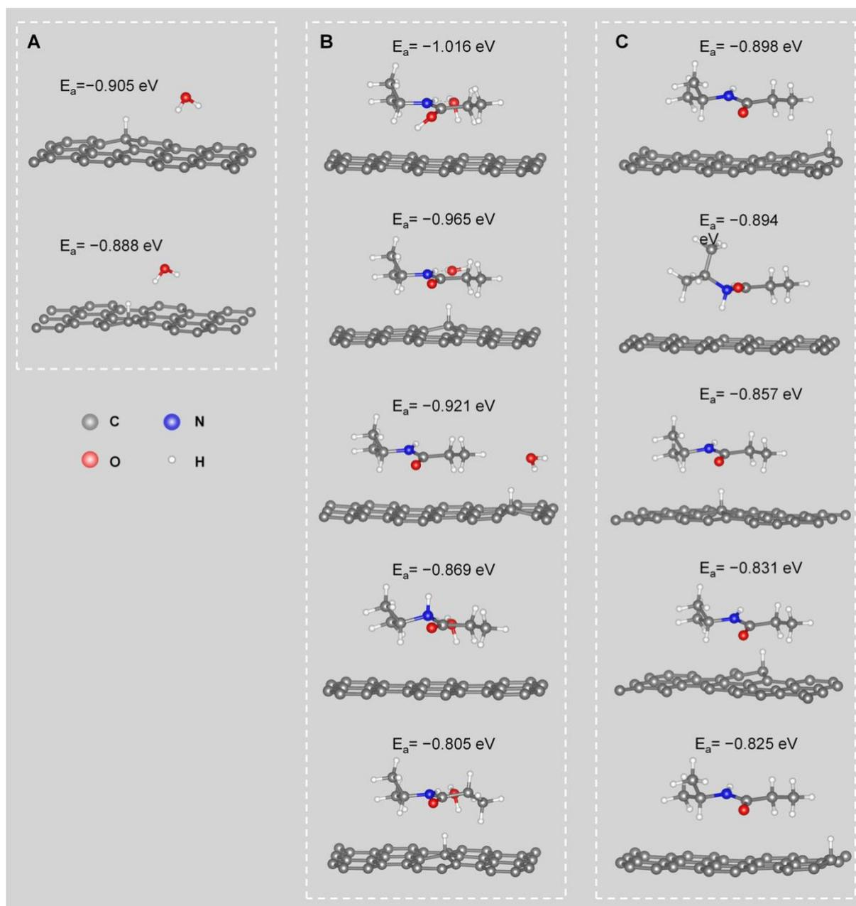
Fig. S7 Additional adsorption configurations of a H on (A) graphene with H<sub>2</sub>O molecule, (B) pNIPAM-graft-graphene with H<sub>2</sub>O, and (C) pNIPAM-graft-graphene, and corresponding adsorption energies.
