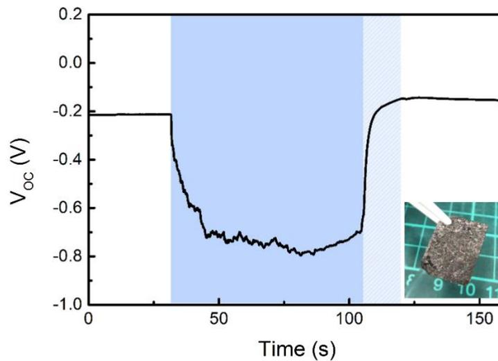
Fig. S3  $V_{oc}$  of a special IPHC sample in response to moisture flow. Blue region represents the supply of moisture flow from 30s to 120s, and light blue region indicates the reduction of voltage response after fully swollen of the pNIPAm hydrogel. Specifically, this sample was prepared by carrying out the polymerization of pNIPAm on the pored CP directly, which features an extremely thin pNIPAm layer. Insert shows digital image of the pored CP coated with pNIPAm.
