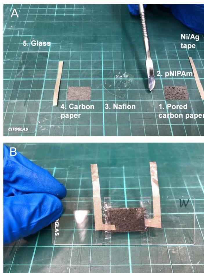
Fig. S1 (A) Materials used to fabricate IPHC consisting of a glass slice, carbon paper, Nafion polymer membrane, pNIPAm hydrogel nanoparticles, pored carbon paper with artificial holes, and Ni/Ag alloy metal tapes. (B) Digital image of an IPHC device.
