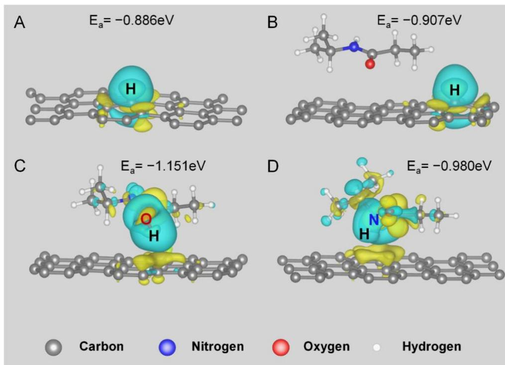
Fig. S6 Charge density difference plots for H adsorbed on (A) graphene, (B, C, and D) pNIPAm-graft-graphene at different absorption sites on the condition without water molecule. The yellow and cyan distribution corresponds to charge accumulation and depletion, respectively. The isosurface value equals to  $0.002e \text{ \AA}^{-1}$ .
