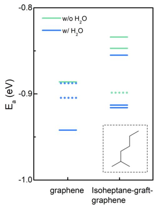
Fig. S8  $E_a$  of graphene and isoheptane-graft-graphene to H on the condition with (blue) and without (green)  $H_2O$ .  $E_a$  of meta-stable adsorption configurations are presented as dashed lines. Inset shows the structural formula of isoheptane molecule.
