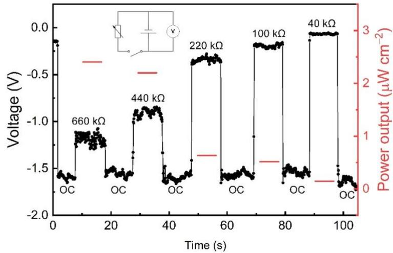
Fig. S2 Electric output of an IPHC device connecting to different load resistances. In this experiment, the device was continuously exposed to the moisture flow while different load resistances were connected in turn from large to small, which is indicated by X-axis of time. Open circuit (OC) condition is shown for the period between two resistances were changed.
