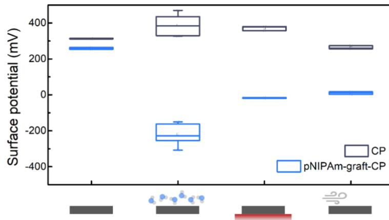
Fig. S10 Surface potential of CP and pNIPAm-graft-CP which were then subjected to moisturizing, baking, and drying via nitrogen gas in proper order.
