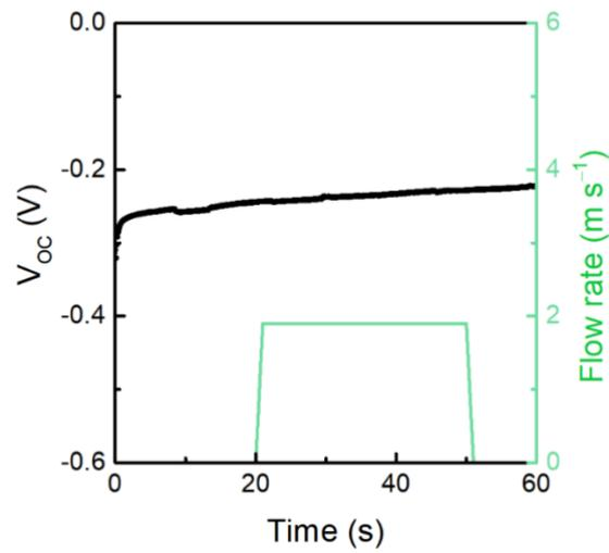
Fig. S13  $V_{oc}$  of an IPHC in response to the supply of dry air and corresponding flow rate.
