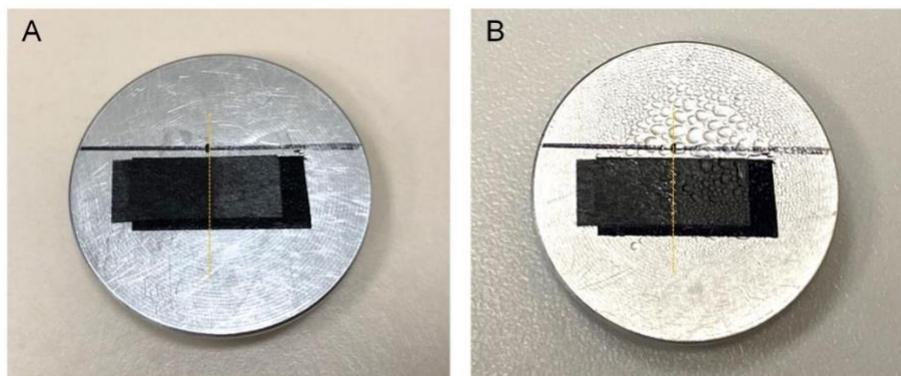
Fig. S11 Digital images of a sample with one-half pNIPAm-graft-CP (left) and one-half pristine CP (right) at (A) dry state and (B) wet state.
