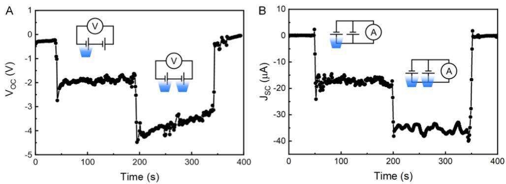
Fig. S15 (A)  $V_{oc}$  of two IPHC devices connected in series. (B)  $J_{sc}$  of two IPHC devices connected in parallel.
