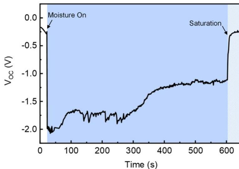
Fig. S4  $V_{oc}$  of an IPHC under continuous moisture flow until its saturation. Blue region shows the supply of moisture flow and light blue region indicates the saturation of the device even the moisture flow lasts after 600s. (The measurement uncertainty in terms of  $V_{oc}$  of *ca.*  $\pm 20\%$  could be observed when the IPHC sample was initially exposed to the moisture flow.)
