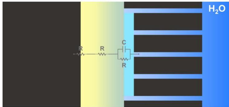
Fig. 18 Equivalent circuit of the IPHC device.
