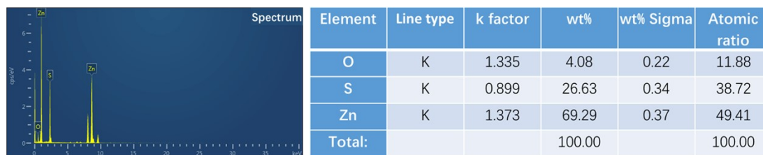
Fig. S4. EDX analysis of ZnO/ZnS nanosheets under HAADF-STEM mode.
