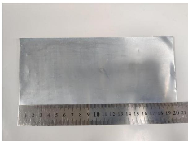
**Fig. S4** Optical image of the scale-up Zn-PA@Zn electrode.
