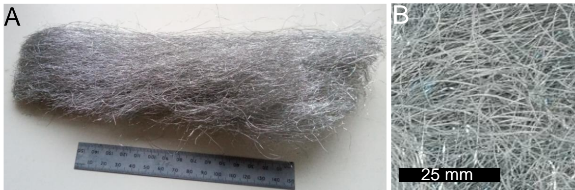
Fig. S2. Aluminium wool used in this study. A,B) Photographs of the filaments of aluminium at two different magnifications. The filaments are up to 300 mm long and have a diameter varying from 100 \mu\text{m} to 300 \mu\text{m} .
