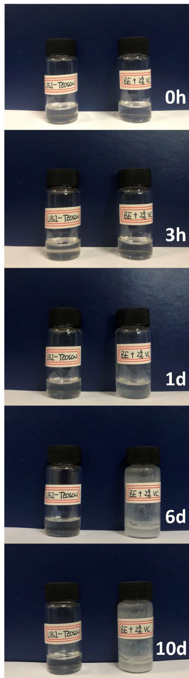
Figure S32. Photographs of LiFSI-TEOSCN and BE + 2% VC electrolyte before and after storage for different times at 25 °C and 50% humidity.
