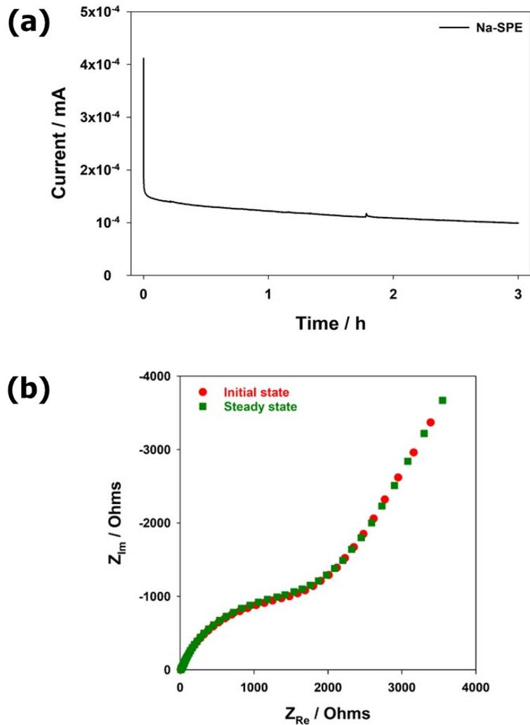
**Figure S1.** (a) Chronoamperometry and (b) impedance spectra for the Na-SPE. T= 20 °C.
