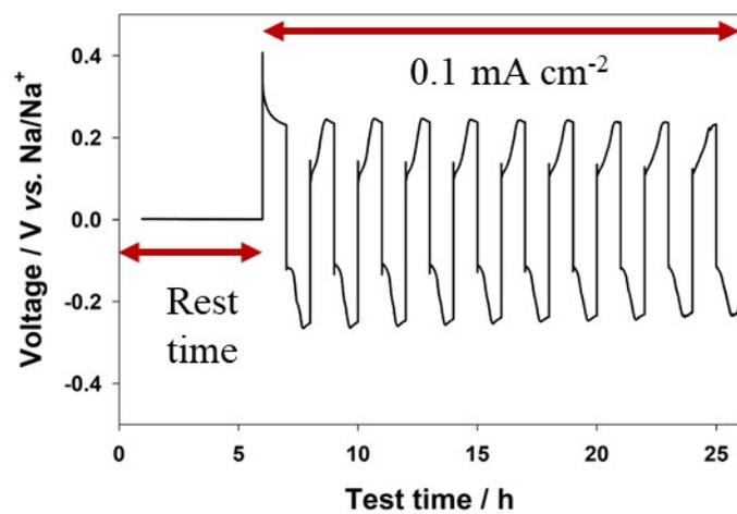
**Figure S2.** Galvanostatic Na plating and stripping performed in a symmetric Na | Na-SPE | Na cell at a current density of  $0.1 \text{ mA cm}^{-2}$ . Each plating or stripping step lasted for 1 hour.  $T = 20 \text{ }^{\circ}\text{C}$ .
