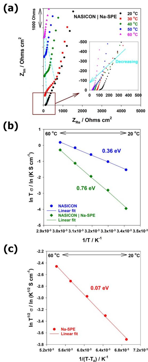
**Figure S4.** (a) Nyquist plots between NASICON | Na-SPE.  $T = 20 \sim 60$  °C. (b, c) Arrhenius plots of 3 types of electrolytes (NASICON, Na-SPE, and NASICON | Na-SPE) to measure activation energies: (b) Na-SPE and (c) NASICON and NASICON | Na-SPE.
