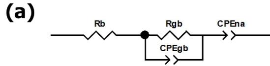
$R_b$ : Bulk resistance of NASICON solid electrolyte
