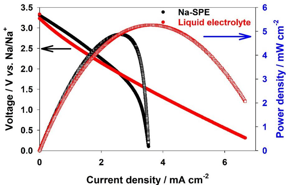
**Figure S6.** Polarization and power density curves measured at a scan rate of  $0.05 \text{ mA s}^{-1}$ . Cell configuration: Cu | Na | Na-SPE or Liquid electrolyte | NASICON | Seawater | Carbon.
