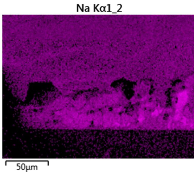
**Figures S7.** EDX mapping image of Na element (cross-sectional image cut by a FIB) for the Na metal harvested anode (composed of the Na-SPE, Na metal, and Al foil current collector).
