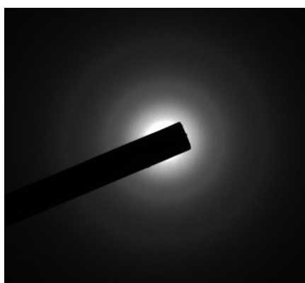
Fig. S8 The ring-like selected area electron diffraction (SAED) image of \text{Fe}_1\text{N}_2\text{O}_2/\text{NC} catalyst.
