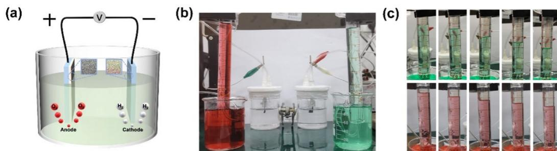
Figure S21. (a) Schematic of the electrolyzed water reaction. (b) H<sub>2</sub> (Green) and O<sub>2</sub> (Red) generated at 5, 10, 15, 20 min, respectively.
