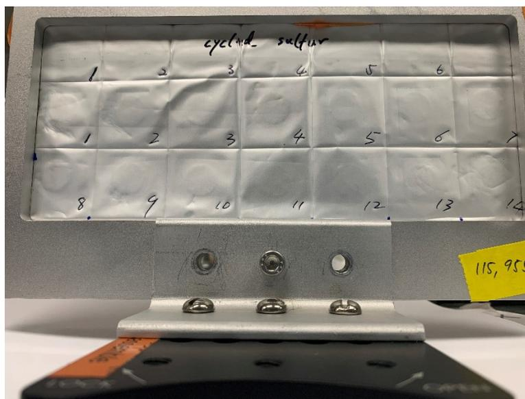
Figure S17. Photograph of sample package used in synchrotron characterization.
