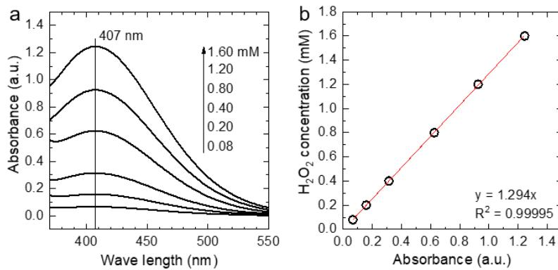
**Figure S4.** UV-Vis spectra (a) and (b) calibration curves of the titration of  $\text{H}_2\text{O}_2$  with a standardized  $\text{Ti}^{4+}$ -oxysulfate solution. The detailed information of standard samples is shown in the method section.
