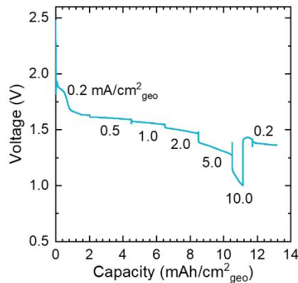
**Figure S17.** Discharge of a molten-salt Na-Ar cell with increasing discharge currents from  $0.2 \text{ mA}/\text{cm}^2_{\text{geo}}$  to  $10.0 \text{ mA}/\text{cm}^2_{\text{geo}}$ .
