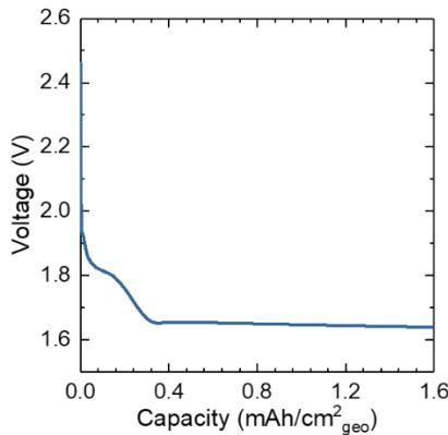
**Figure S16.** The discharge profile of a molten-salt  $\text{Na}-\text{Ar}$  battery at a current of  $0.4 \text{ mA}/\text{cm}^2_{\text{geo}}$  for  $1.6 \text{ mAh}/\text{cm}^2_{\text{geo}}$ .
