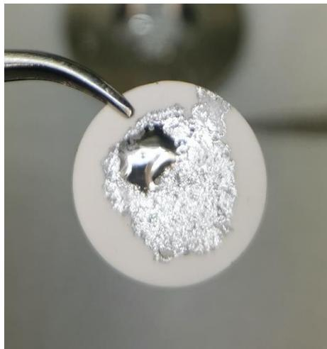
**Figure S2.** Photo of a  $\beta\text{-Al}_2\text{O}_3$  membrane after 2 hours of resting in a  $\text{Na-O}_2$  cell.
