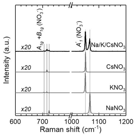
**Figure S14.** The Raman spectra of commercial  $\text{Na}_2\text{O}_2$ ,  $\text{NaNO}_3$ ,  $\text{KNO}_3$ ,  $\text{CsNO}_3$  and eutectic salts ( $\text{Na}/\text{K}/\text{CsNO}_3$ ). The eutectic salts were prepared by mixing the  $\text{NaNO}_3$  (26.4 w%),  $\text{KNO}_3$  (27.3 w%), and  $\text{CsNO}_3$  (46.3 w%) salts at 473 K for 12 h in an Ar-filled glove box. All these Raman spectra were collected at room temperature in an air-tight cell with Ar environment.
