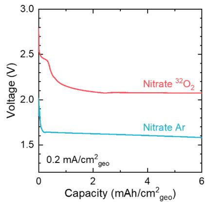
**Figure S15.** Discharge profiles of molten salt  $\text{Na}-\text{O}_2$  and  $\text{Na}-\text{Ar}$  cells for quantifications in Figure 4a.
