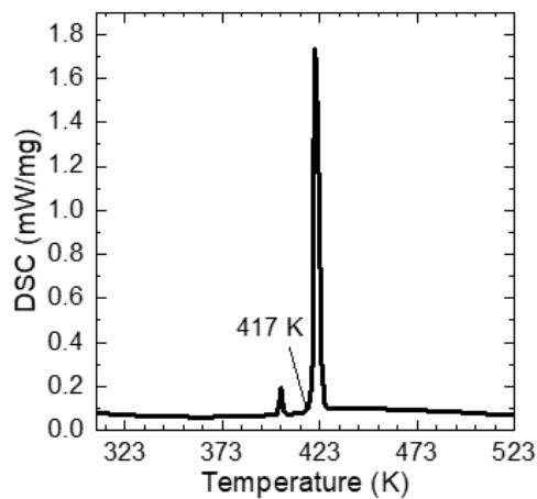
**Figure S5.** The differential scanning calorimetry (DSC) result of the eutectic salts ( $\text{NaNO}_3$  26.4 w%,  $\text{KNO}_3$  27.3 w%, and  $\text{CsNO}_3$  46.3 w%). The onset of the melting point of the eutectic salts was ~417 K.
