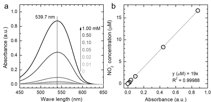
**Figure S3.** UV-Vis spectra (a) and calibration curve (b) for nitrite ( $\text{NO}_2^-$ ) titration via the Griess method<sup>2</sup>. The standard  $\text{NO}_2^-$  solutions (0, 0.01, 0.02, 0.05, 0.1, 0.5, 1 mM) were used for obtaining the calibration curve (b).
