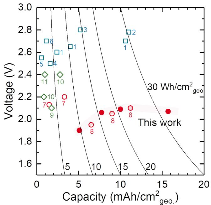
**Figure S1.** The comparison of capacity-voltage plot for alkali metal-oxygen batteries ( $\text{Li-O}_2^{1-6}$ ,  $\text{Na-O}_2^{7,8}$ ,  $\text{K-O}_2^{9-11}$  batteries). The detailed information on the reported performance was shown in Table S1.
