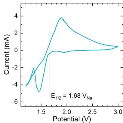
**Figure S19.** The CV of a molten-salt Na-Ar cell at scanning rate of  $0.2 \text{ mV/s}$  in the potential range from  $1.2$  to  $3.0 \text{ V}$ . The molten-salt Na-Ar cell contains liquid Na negative electrode,  $\beta\text{-Al}_2\text{O}_3$  membrane, Ni/salts positive electrode, Stainless steel (SS) plate. The salts are a mixture of  $\text{NaNO}_3$  (26.4 w%),  $\text{KNO}_3$  (27.3 w%), and  $\text{CsNO}_3$  (46.3 w%).
