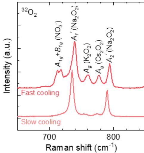
**Figure S11.** The Raman spectra of Ni/salts electrodes (8/5 in weight) with the addition of Na<sub>2</sub>O before and after reaction in 280 kPa (RT) of <sup>32</sup>O<sub>2</sub> at 443 K. The cells were cooled down with fast (~20 K/min) and slow rates (1 K/min).
