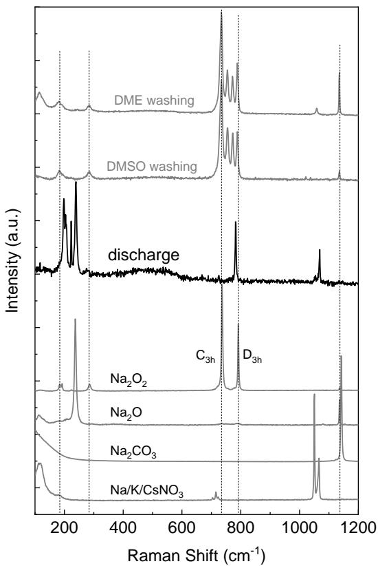
**Figure S12.** The Raman spectra of Ni/NaNO<sub>3</sub>/KNO<sub>3</sub>/CsNO<sub>3</sub>/SS electrode after discharge with different washing procedures. Raman spectra of commercial Na<sub>2</sub>O<sub>2</sub>, Na<sub>2</sub>O, Na<sub>2</sub>CO<sub>3</sub> and eutectic salts (Na/K/CsNO<sub>3</sub>) were used as the references
