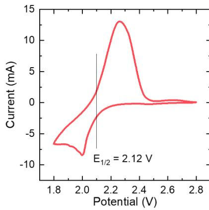
**Figure S13.** The CV of a molten salt Na-O<sub>2</sub> cell in O<sub>2</sub> atmosphere ranging from 1.8 to 2.8 V. The scanning rate was set as 0.2 mV/s. The molten-salt Na-O<sub>2</sub> cell contains liquid Na negative electrode, β-Al<sub>2</sub>O<sub>3</sub> membrane, Ni/salts positive electrode, 280 kPa O<sub>2</sub> (RT), Stainless steel (SS) plate. The salts are a mixture of NaNO<sub>3</sub> (26.4 w%), KNO<sub>3</sub> (27.3 w%), and CsNO<sub>3</sub> (46.3 w%).
