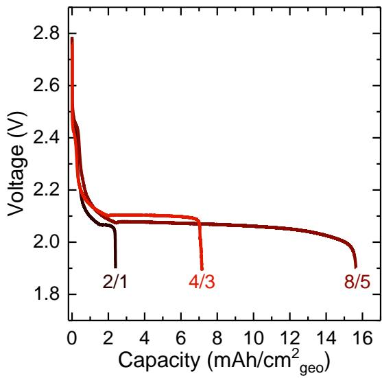
**Figure S6.** The discharge profiles of molten-salt Na-O<sub>2</sub> batteries with the different ratios of Ni/salts (2/1, 8/5, and 4/3). The discharge current is 0.2 mA/cm<sup>2</sup><sub>geo</sub>. The operation temperature was 443 K. The O<sub>2</sub> pressure in the cell is ~280 kPa at room temperature. The salts were the mixture of NaNO<sub>3</sub> (26.4 w%), KNO<sub>3</sub> (27.3 w%), and CsNO<sub>3</sub> (46.3 w%).
