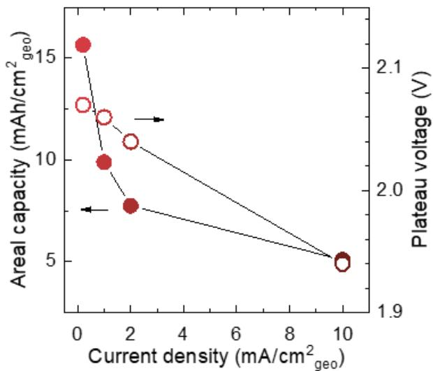
**Figure S7.** The change of the areal capacities and plateau voltages with increasing discharge currents (0.2, 1.0, 2.0, 10.0 mA/cm<sup>2</sup><sub>geo</sub>).
