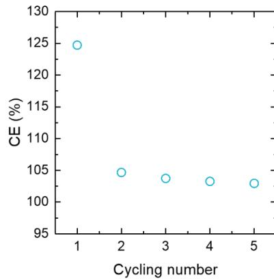
**Figure S18.** The Coulombic efficiencies of a molten-salt Na-Ar battery at a current density of  $1 \text{ mA}/\text{cm}^2_{\text{geo}}$  for 5 cycles with a limited discharge capacity of  $2.0 \text{ mA}/\text{cm}^2_{\text{geo}}$  at the temperature of 443 K.
