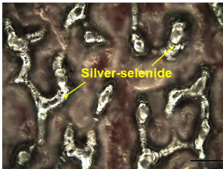
Figure S9. Optical microscopy image showing sublimation of the silver-selenide nanostructures under excessive input energy.
