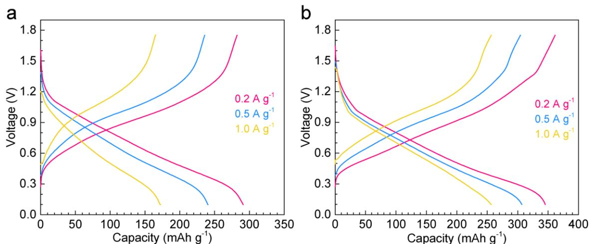
**Fig. S3** The GCD curves of TDT cathode with a)  $1.2 \text{ mg cm}^{-2}$  loading and 5% carbon, b)  $10 \text{ mg cm}^{-2}$  loading and 10% carbon.
