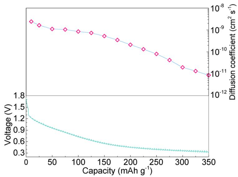
**Fig. S7** GITT curves and calculated diffusion coefficients of TDT.
