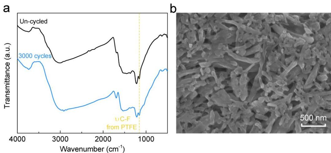
**Fig. S5** (a) FT-IR spectra of pristine TDT cathode and after 3000 cycles. (b) SEM image of TDT cathode after 3000 cycles.
