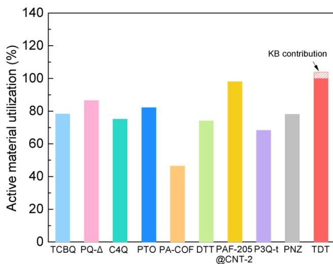
**Fig. S4** Active material utilization comparison of TDT with reported organic cathode materials in aqueous zinc batteries.
