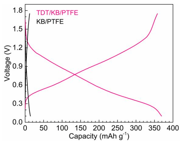
**Fig. S2** The GCD curves of TDT electrode and the electrode containing only KB and PTFE (the specific capacity is calculated based on the loading of TDT for direct comparison).
