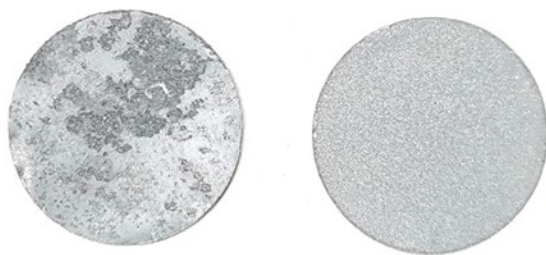
Figure S12. The optical images of cycled Zn anodes after 50 cycles in different electrolytes (left: ZS; right: SPS10).
