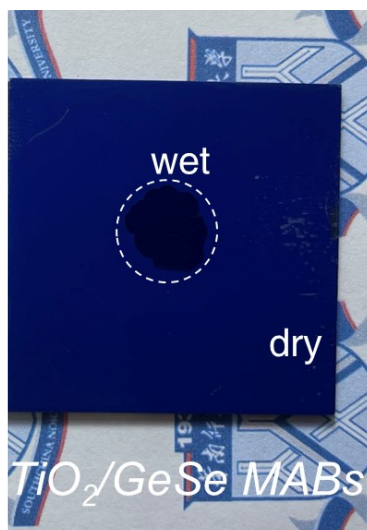
Figure S12. Photograph of the TiO 2 /GeSe MABs film in dry and wet state.
