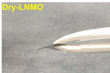
Figure S17. Adhesion check between electrode and current collector after 300 cycles. Side view of cycled (A) dry-LNMO and (B) slurry-based LNMO.
