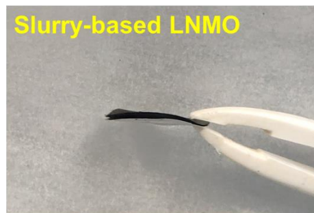
Figure S17. Adhesion check between electrode and current collector after 300 cycles. Side view of cycled (A) dry-LNMO and (B) slurry-based LNMO.
