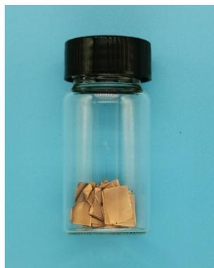
Figure S18. Separated copper foil pieces from spent anodes of different battery manufacturers.
