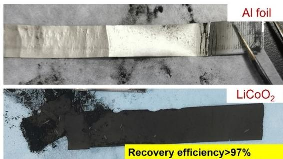
Figure S20. Pictures of recycled Al foil and LCO materials via our rolled-over heating method.
