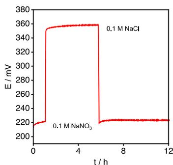
Figure S3 : Response of nitrate-selective electrode in 0.1 M  $\text{NaNO}_3$  for 1h followed by immersion in 0.1 M  $\text{NaCl}$  for 6h. The electrodes were then again immersed in 0.1 M  $\text{NaNO}_3$  to check the signal recovery. No water layer formation could be observed during the testing period.
