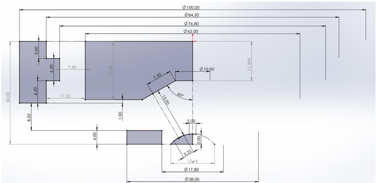
Figure S5 : Schematic side cut of sensing dome and its housing. The dimension are given in mm.
