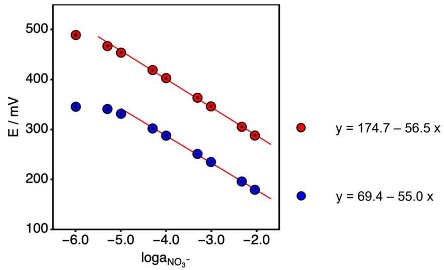
Figure S7 : Potentiometric response of same nitrate-selective electrode versus double-junction reference electrode before immersion in real sample (red trace) and after 75h immersion in real sample (blue trace). Error bars represent standard deviation (n=3).
