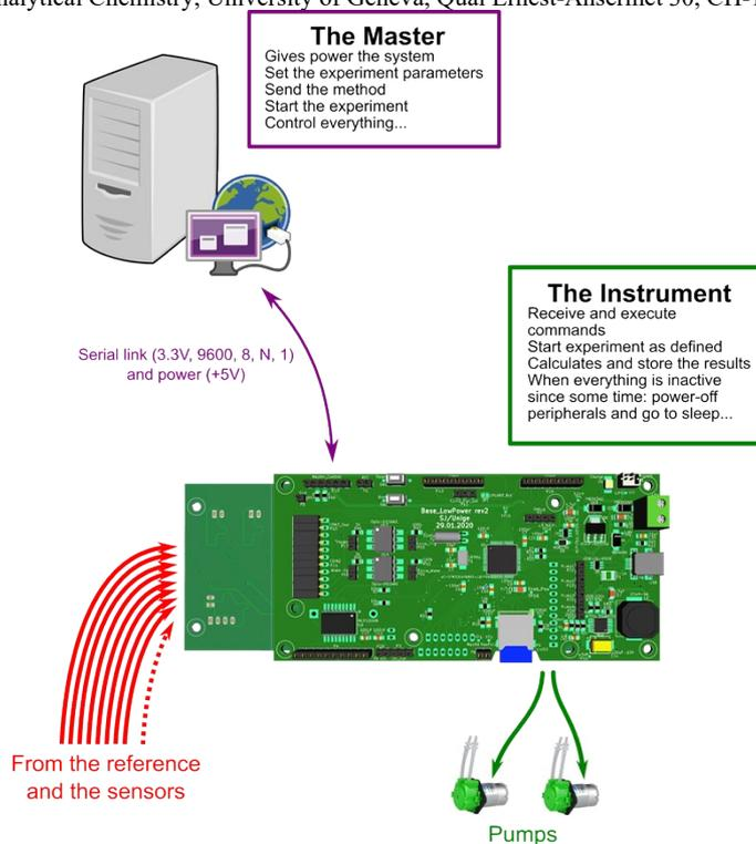
Figure S1 : Scheme of main board controlling the probe. The Master (user) controls the probe and sets up the experiment that is run by the instrument. Through commands the instrument activates pump and executes different operations
