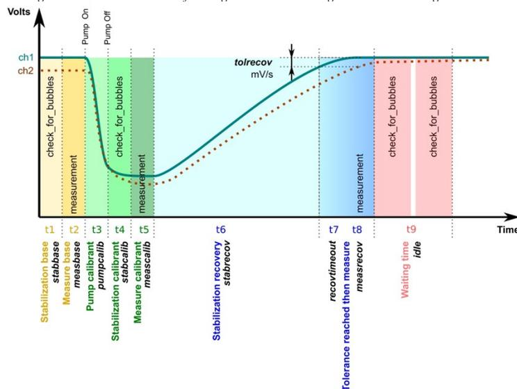
Figure S6 : Preprogrammable calibration routine. All timed events ( $t1 - t9$ ) can be determined individually to customise the protocol to the adequate length and their description can be found in Table S5
