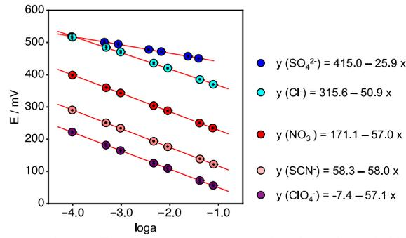
Figure S4 : Potentiometric response of electrode for several anions. The selectivity experiment was performed according to the MSSM, where calibrations were performed sequentially according to the lipophilicity of the anions. From top to bottom, potentiometric response towards:  $\text{Na}_2\text{SO}_4$  (blue),  $\text{NaCl}$  (cyan),  $\text{NaNO}_3$  (red),  $\text{NaSCN}$  (pink) and  $\text{NaClO}_4$  (purple).
