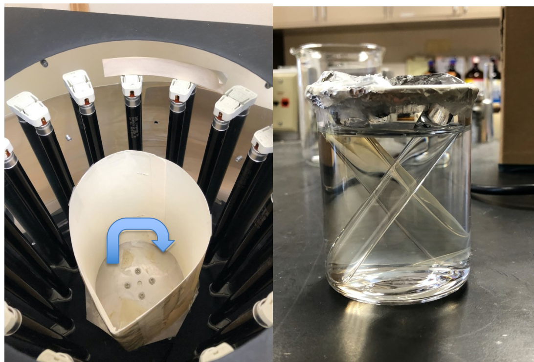
Figure S1: Pictures of the plastics mounted on cardstock on a rotating platform in the photochemical reactor when exposed in air with arrow representing the rotation of the platform. Quartz beaker containing polymer thin film held in place by quartz test tubes. Beaker replaces the cardstock support and is simply placed on the rotating pedestal.
