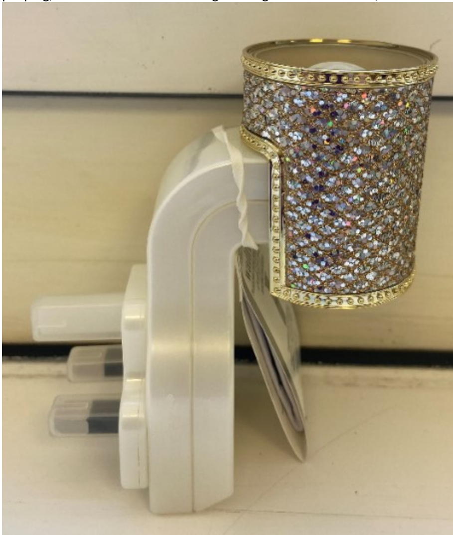
Figure 4 – images showing the plug-in diffuser used in this study. It consists of a standard UK three-pin plug, and a small tank containing the fragrance oil and wick, covered with a fascia plate.
