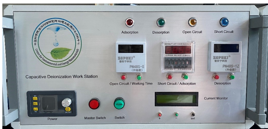
Fig. S1. Photograph of home-made real-time current and energy consumption detector.
