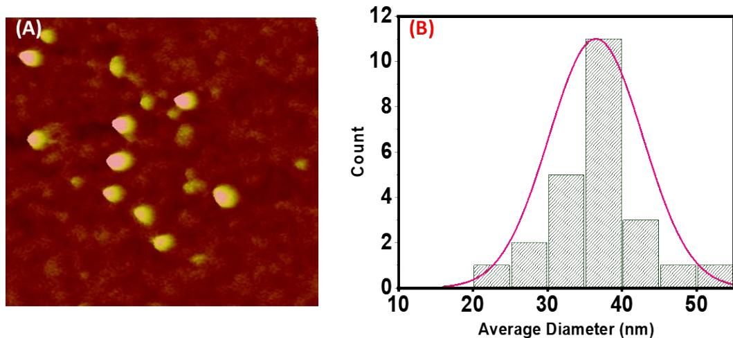
Figure S4(A): Atomic Force Microscopic image showing the morphology of CuNi/IL alloy nanoparticles and (B) histogram of average size of CuNi/IL alloy nanoparticles calculated using Gwydion software.
