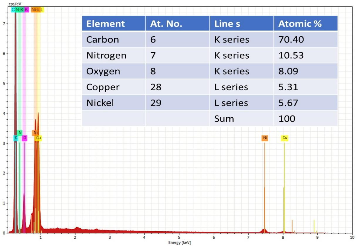
Figure S-13: EDS spectrum of CuNi/IL@MWCNTs nanocomposite.
