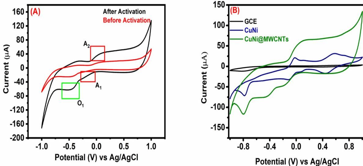
Figure S6: (A) Cyclic voltammetry response of CuNi/IL@MWCNTs before and after activation for 60 cycles in 0.1M PBS at 100mVs<sup>-1</sup> scan rate. (B) CV response of GCE, CuNi/IL, CuNi@MWCNTs towards IMD sensing in 0.1M PBS at 100mVs<sup>-1</sup> scan rate.
