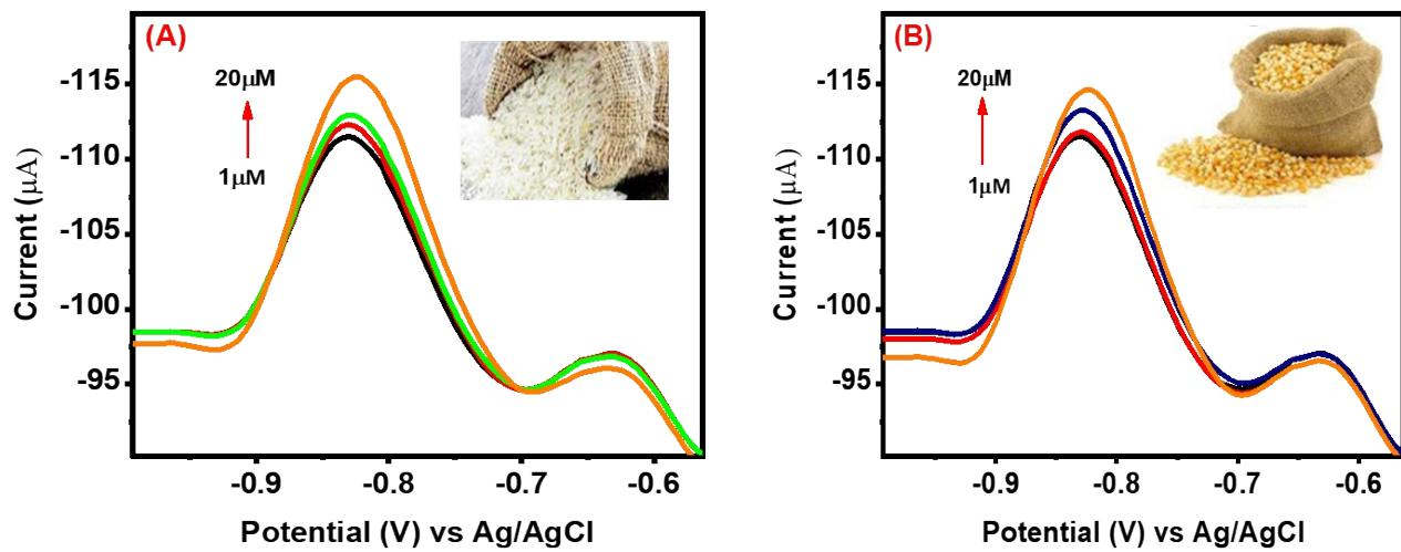
Figure S9: DPV response of CuNi/IL@MWCNTs towards IMD sensing (A) in rice samples; (B) in corn samples.
