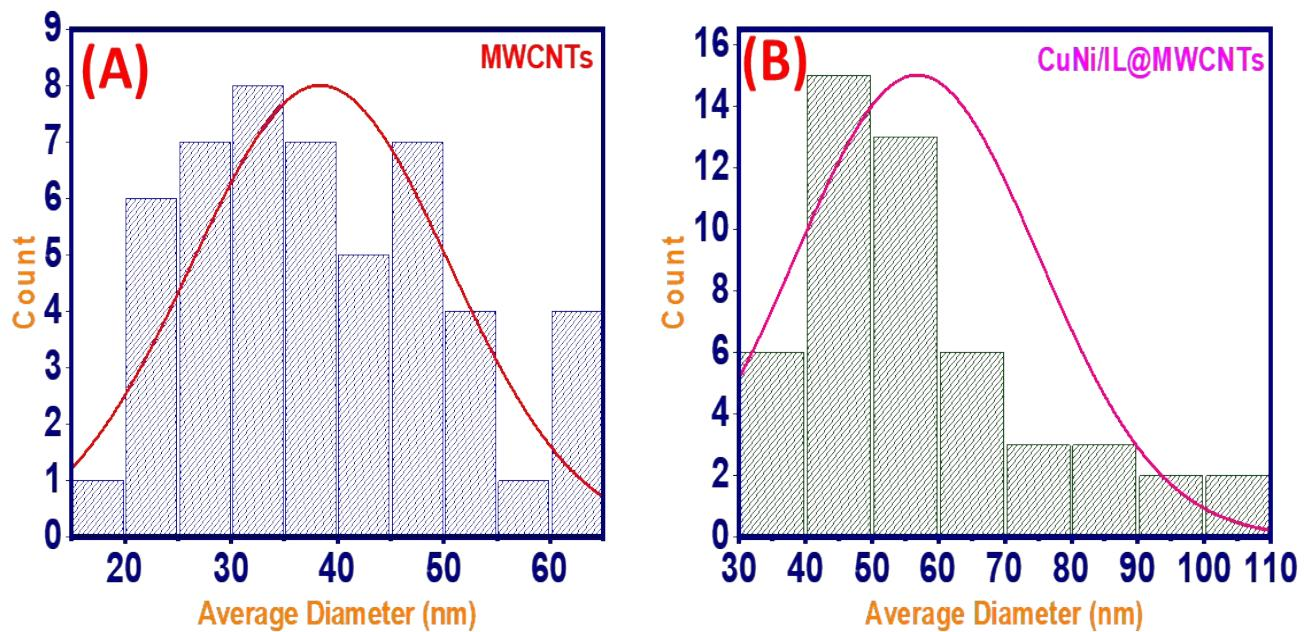
Figure S5: (A) Histogram of average size of MWCNTs and (B) CuNi/IL@MWCNTs nanocomposite calculated using Gwydion software from AFM images.
