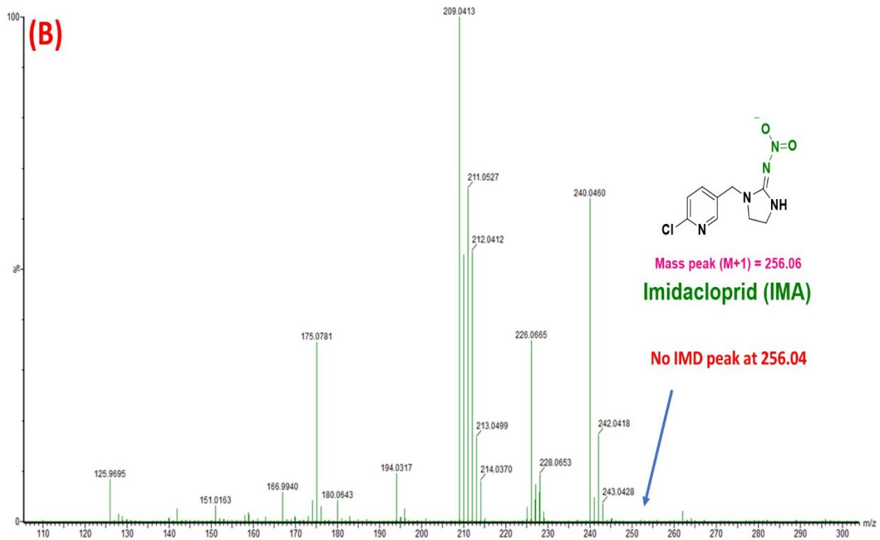
Figure S10: MS data of IMD in presence of (A)  $\text{NaBH}_4$  (B)  $\text{CuNi/IL@MWCNTs}$  with  $\text{NaBH}_4$ .
