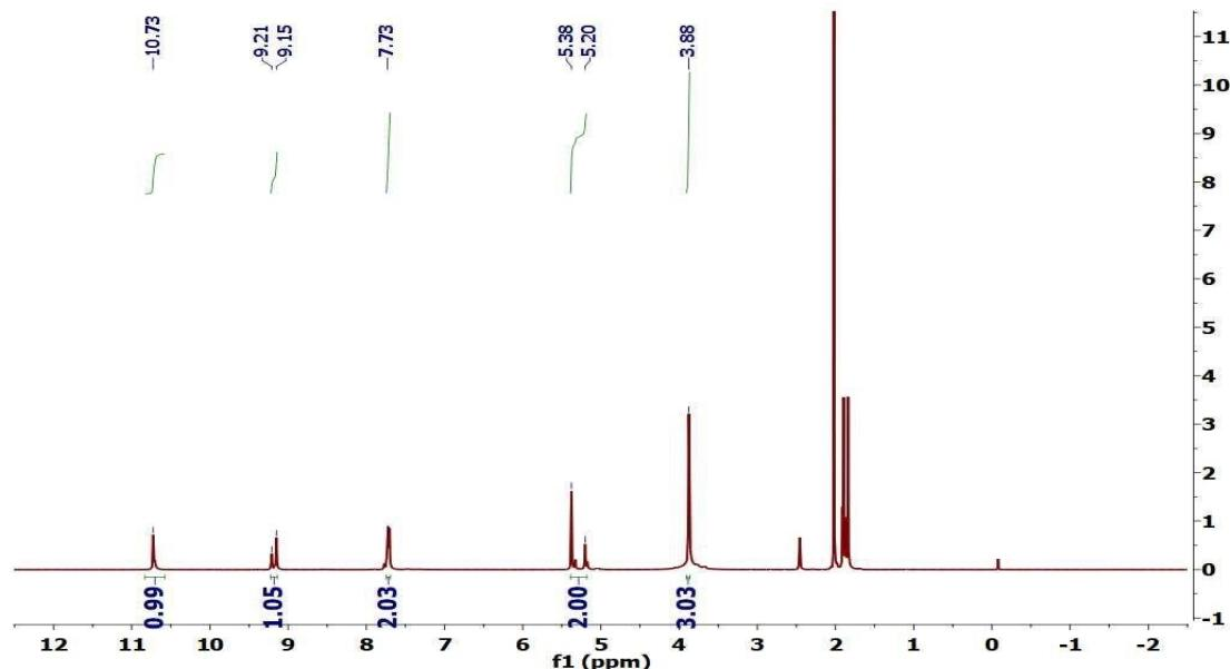
Figure S2:  $^1\text{H}$ -NMR spectrum of Ionic liquid (IL);  $^1\text{H}$  NMR (400MHz, DMSO-d6) –  $\delta$  10.73 (s, 1H, NH), 9.21-9.15 (s, 1H, C2H-Im), 7.33, 7.70 (d, 2H, C4H, C5H-Im), 5.38-5.20 (s, 2H, CH2CO), 3.88 (s, 3H, CH3-N).
