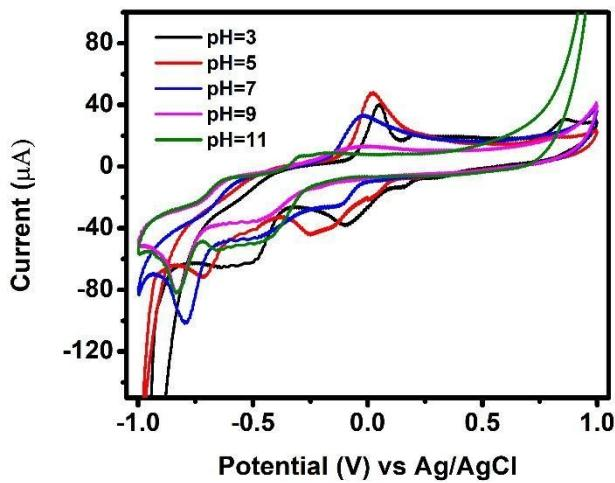
Figure S7: Cyclic voltammetry response of CuNi/IL@MWCNTs towards IMD sensing in different pH (3to11) in 0.1M PBS at  $100\text{mVs}^{-1}$  scan rate.
