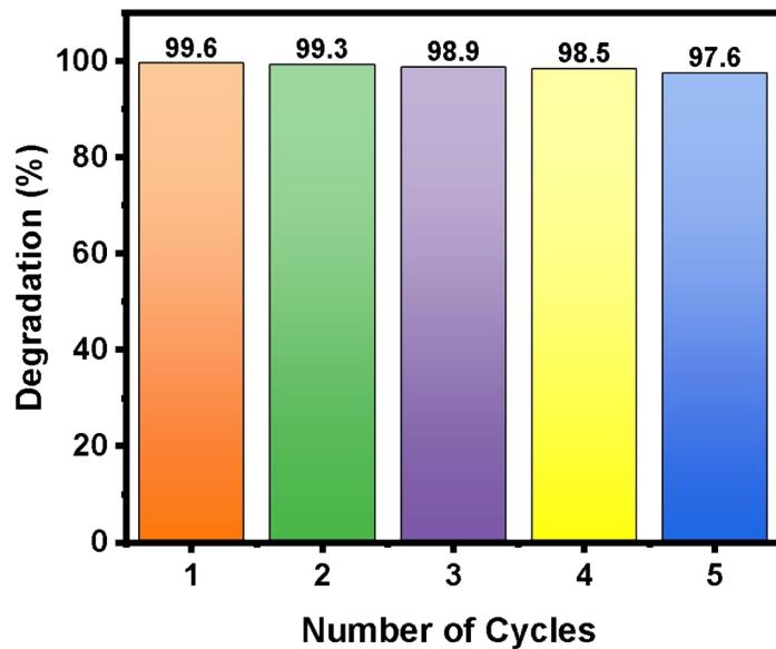
Figure S11: Reusability of  $\text{CuNi/IL@MWCNTs}$  for degradation of IMD after 5 cycles.
