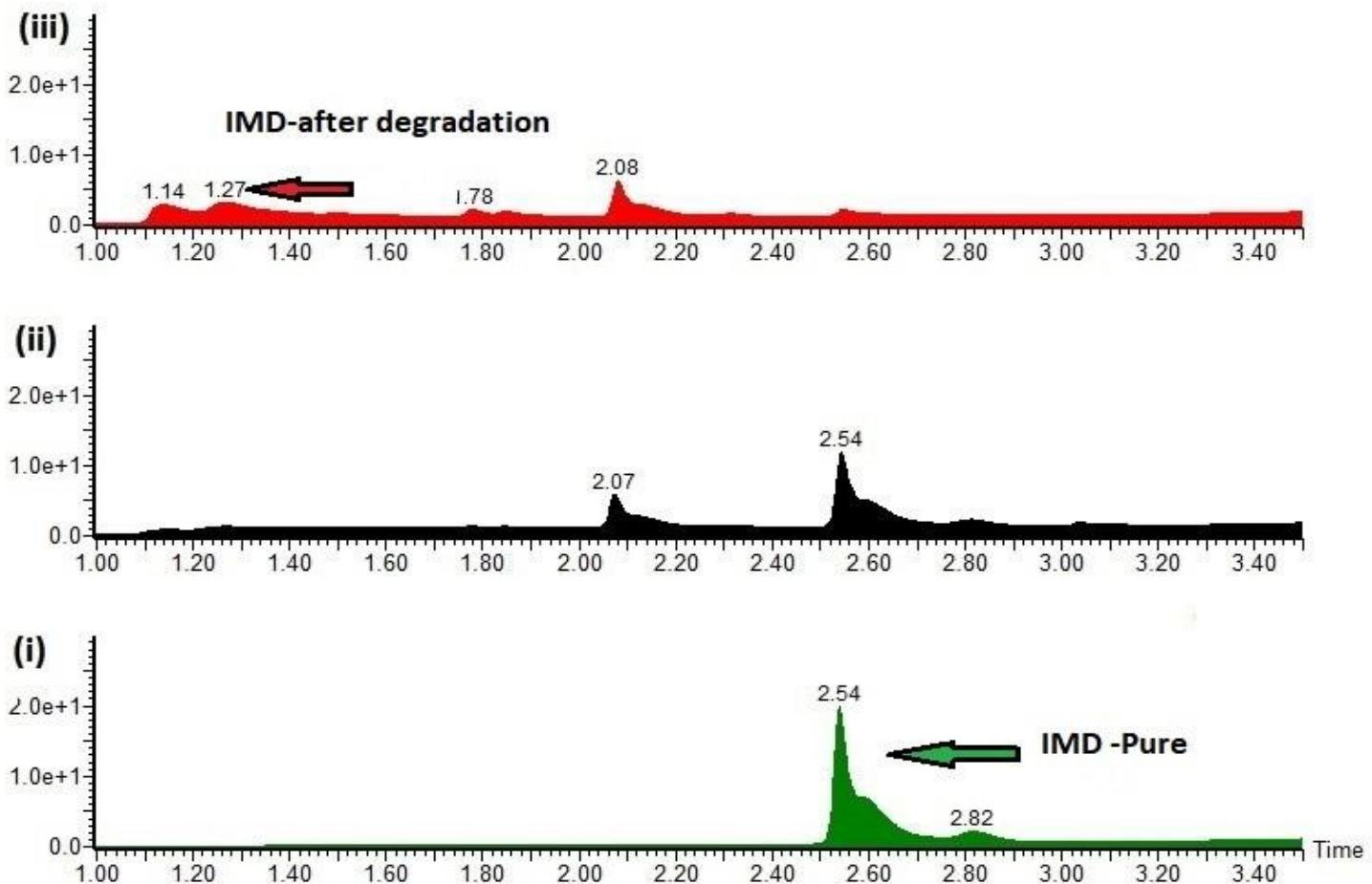
Figure S-12: LC-MS chromatograms: (i) pure IMD, (ii) Intermediate during reduction, (iii) after complete reduction;
