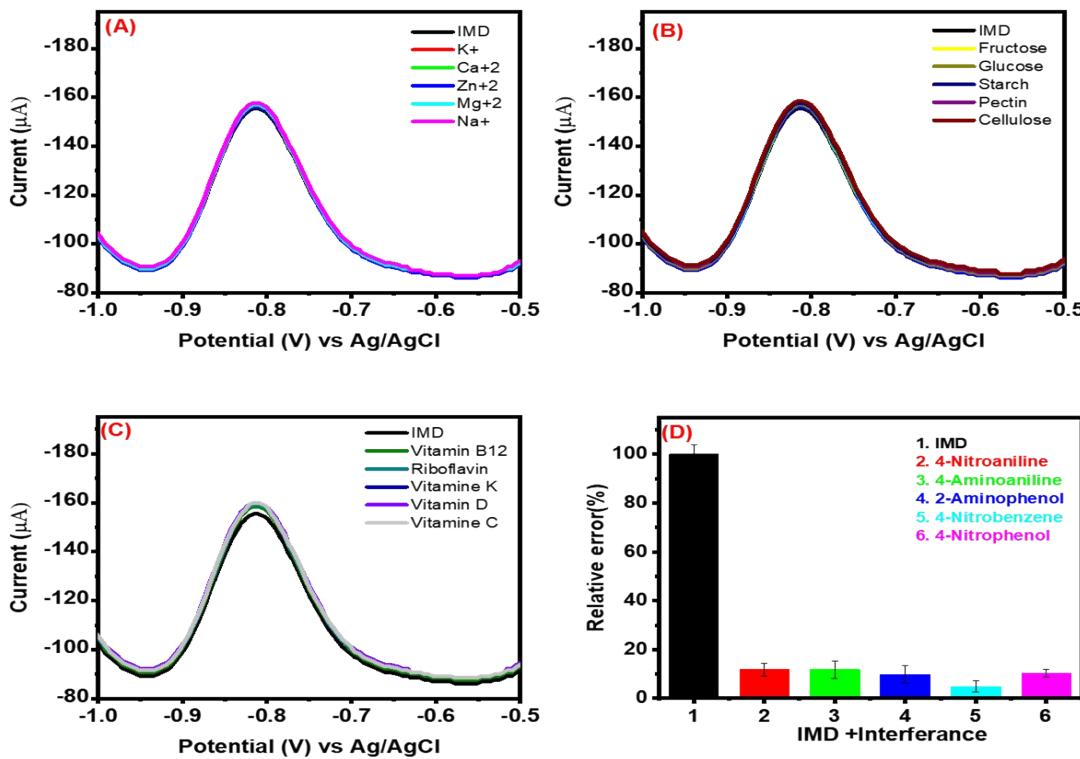
Figure S8: DPV response of CuNi/IL@MWCNTs (A) anions; (B) polysaccharides; (C) Vitamins; (D) Bar graph showing change in current response of CuNi/IL@MWCNTs towards IMD in presence of nitroaromatic compounds.
