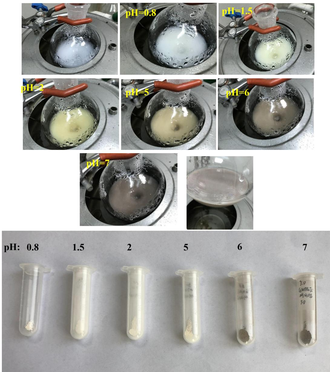
**Fig. S2.** The color of precipitant at different pH values and the relevant  $\text{Ce}_{0.027}\text{W}_{0.02}\text{Mn}_{0.054}\text{TiO}_x$  precursor during the preparation process using the two-step precipitation approach.
