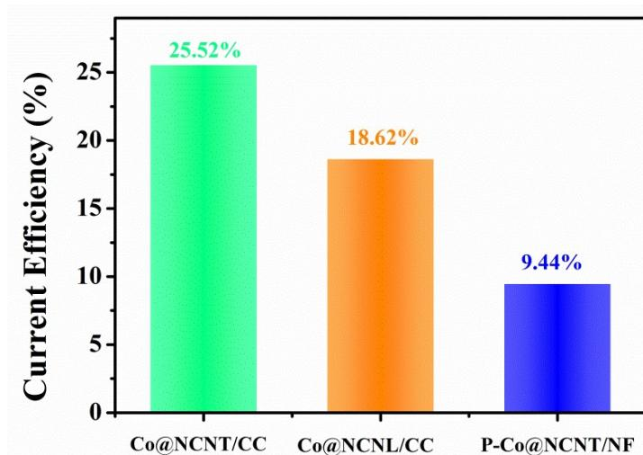
**Fig. S6.** Current efficiency CE(%) of three investigated electrodes for ENRR at  $10 \text{ mA cm}^{-2}$ .
