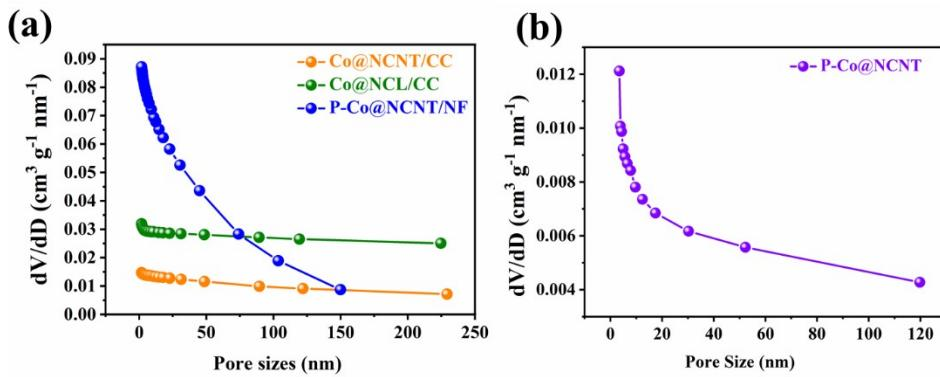
**Fig. S11.**  $\text{N}_2$  adsorption–desorption isotherms and pore-size distributions of (a) three electrode samples and (b) P-Co@NCNT.
