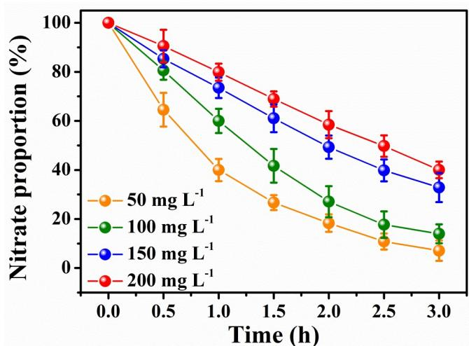
**Fig. S16.** Effect of initial nitrate concentration on the ENRR performance of Co@NCNT/CC. Experimental conditions: 1.5 g L<sup>-1</sup> NaCl, 100 mL of electrolyte, 10 mA cm<sup>-2</sup> current density, and initial pH = 7. 50.
