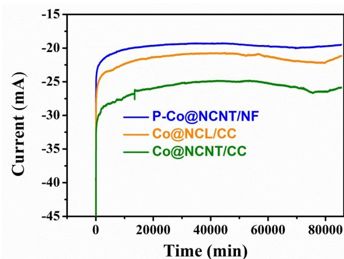
**Fig. S4.** I-t curves of three investigated catalysts at -1.3 V vs. SCE.
