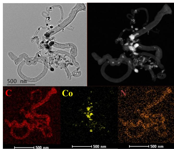
**Fig. S3.** HRTEM elemental mapping of Co@NCNT/CC.
