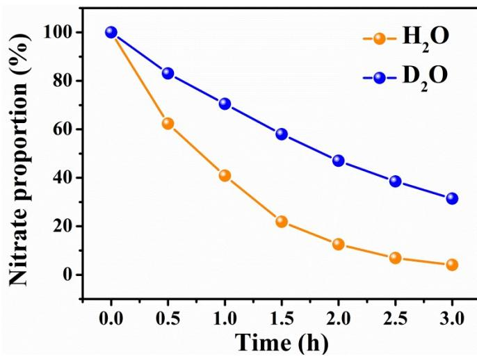
**Fig. S17.** Effect of D<sub>2</sub>O replacement on the ENRR performance of Co@NCNT/CC. Experimental conditions: 1.5 g L<sup>-1</sup> NaCl, 100 mL of electrolyte, 10 mA cm<sup>-2</sup> current density, and initial pH = 7. 50.
