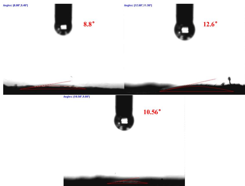
**Fig. S10.** Contact angles of P-Co@NCNT powders.
