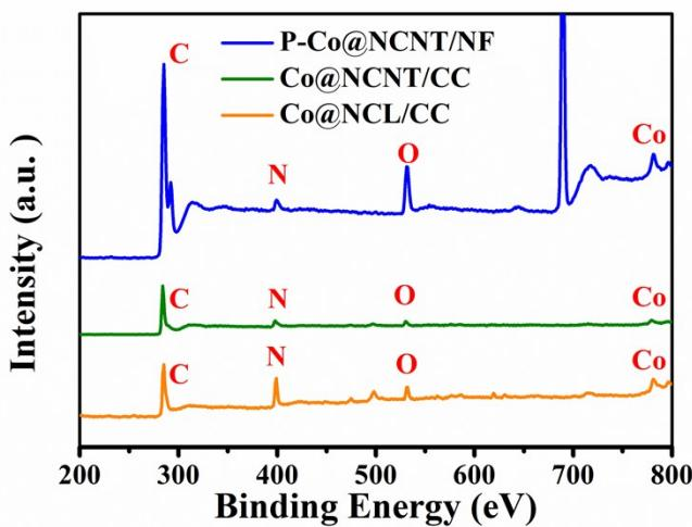
**Fig. S1.** XPS survey spectra of Co@NCNT/CC, Co@NCL/CC and P-Co@NCNT/NF.
