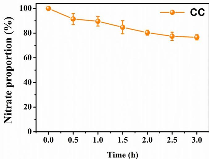
**Fig. S5.** Time courses of nitrate proportion for the pure CC towards ENRR. Experimental conditions: initial  $[NO_3^-N] = 50 \text{ mg L}^{-1}$ , current density of  $10 \text{ mA cm}^{-2}$ , and electrolysis time of 3 h.
