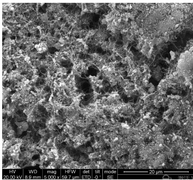
**Fig. S19.** SEM image of reacted Co@NCNT/CC (after 30 cycles).
