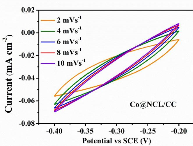
**Fig. S13.** CV curves of Co@NCL/CC at various scan rates recorded in  $50 \text{ mg L}^{-1} \text{NO}_3^-$ -N and under  $\text{N}_2$ -saturated conditions.
