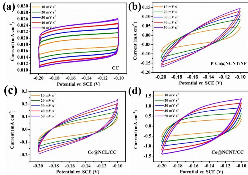
**Fig. S12.** CV curves of different electrode samples at various scan rates for identifying EASA.
