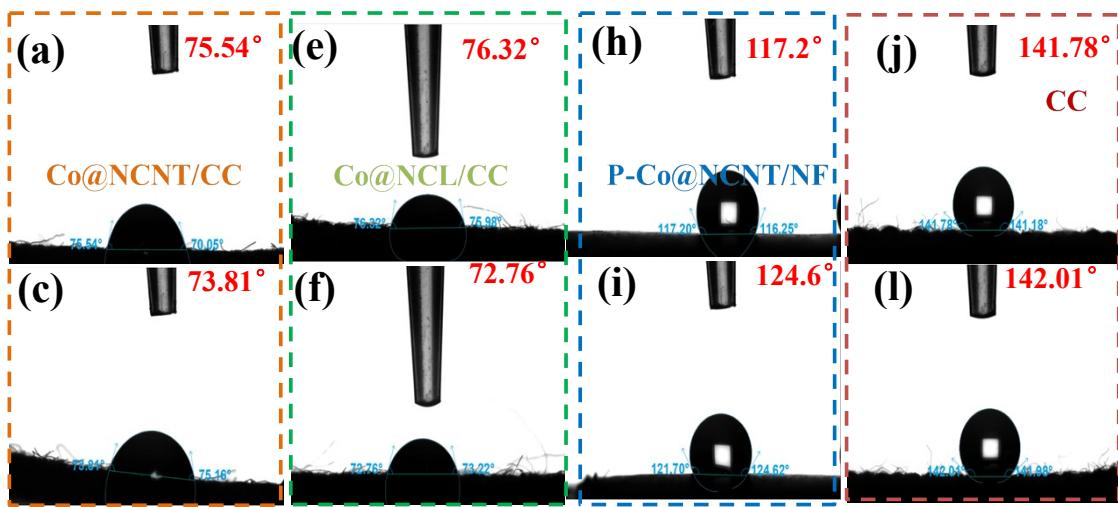
**Fig. S9.** Comparison of contact angles of the four samples.
