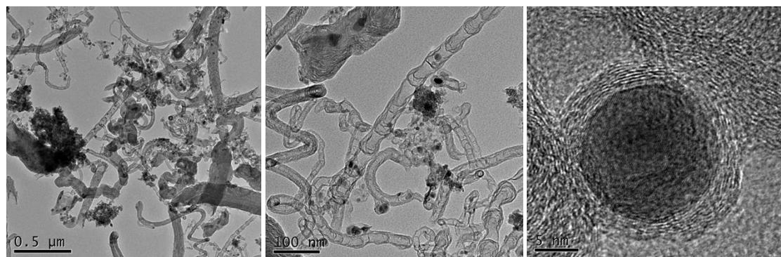
**Fig. S20.** HRTEM images of reacted Co@NCNT/CC (after 30 cycles) at different magnifications.
