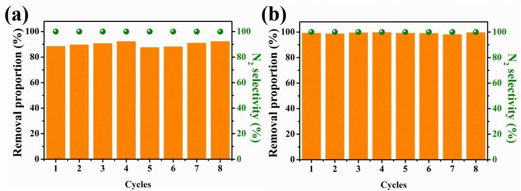
**Fig. S21.** Long-term operation stability of Co@NCNT/CC for ENRR at an initial pH of (a) 3 and (b) 14. Reaction conditions: electrolyte containing  $50 \text{ mg L}^{-1} \text{NO}_3^-$ -N,  $50 \text{ mM Na}_2\text{SO}_4$ , and  $1.5 \text{ g L}^{-1} \text{NaCl}$ ; current density of  $10 \text{ mA cm}^{-2}$ ; and electrolysis of 3 h.
