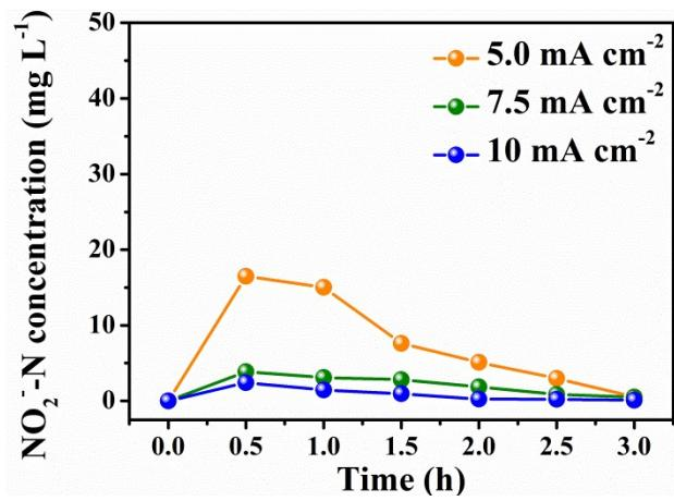
**Fig. S15.** Time courses of  $\text{NO}_2^-$ -N concentration for ENRR on Co@NCNT/CC as a function of current density.
