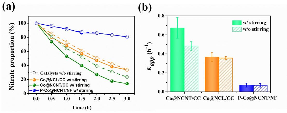
**Fig. S8.** Comparisons of (a) nitrate removal efficiency and (b) corresponding  $K_{app}$  values of three catalysts during the stirring-control experiments. The initial concentration of  $NO_3^-$ -N was 100 mg L<sup>-1</sup>.
