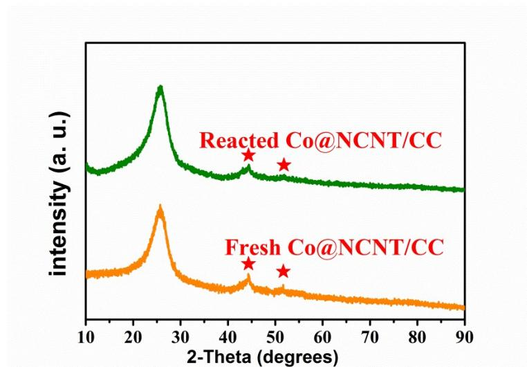
**Fig. S18.** XRD patterns of fresh and reacted Co@NCNT/CC (after 30 cycles).
