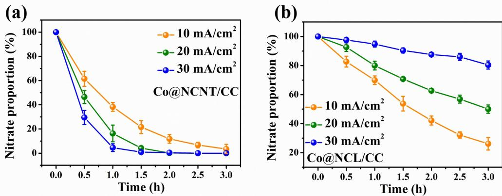
**Fig. S7.** Effect of current density on the ENRR performance of Co@NCNT/CC and Co@NCL/CC.
