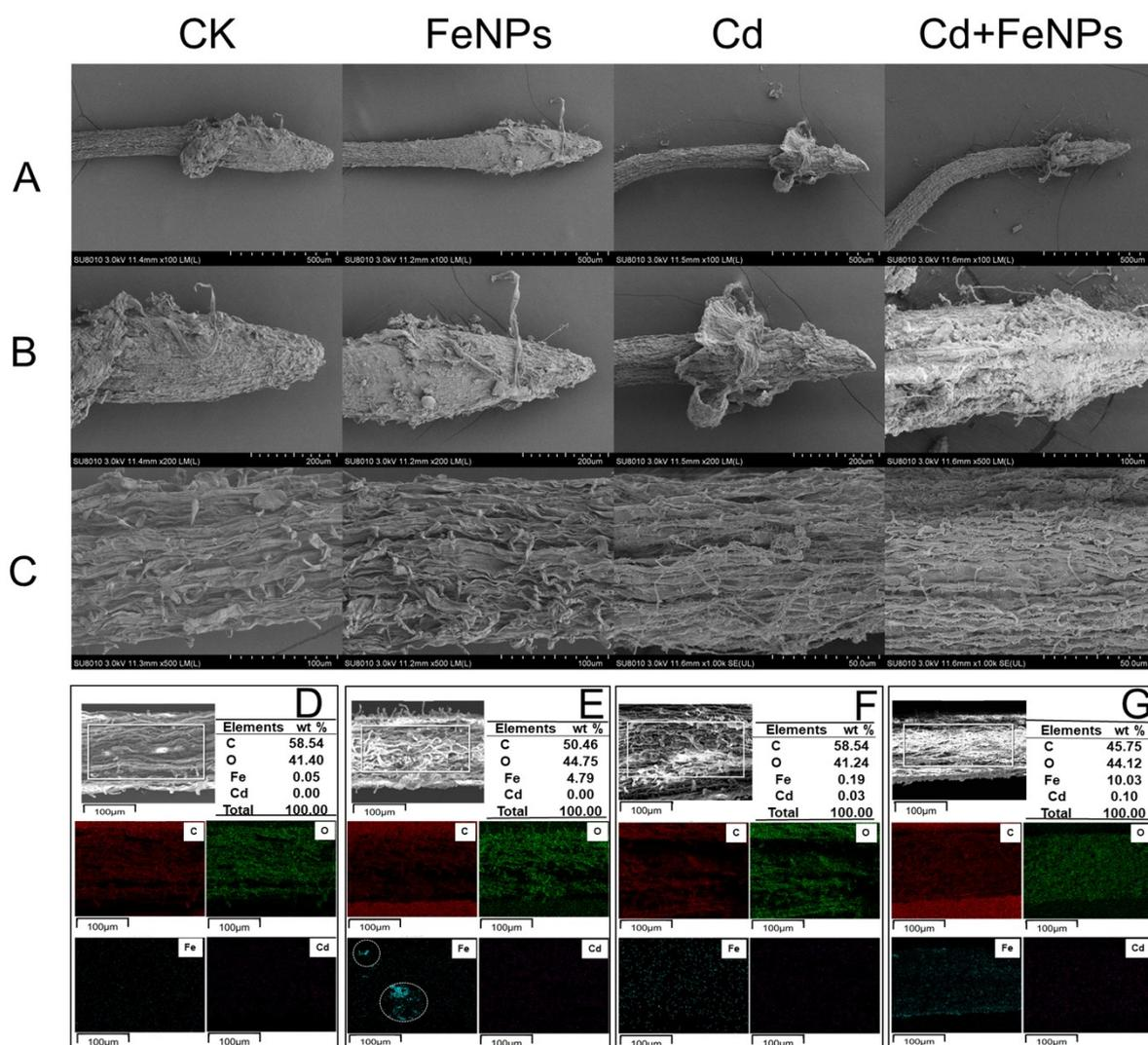
**Figure S2.** Scanning electron microscopic (SEM) image of the rice seedlings (A, B, and C) and EDS analysis of the elements on the root surface including C, O, Fe, and Cd (D, E, F, G) in CK, FeNPs, Cd, and Cd+FeNPs treatments, respectively.
