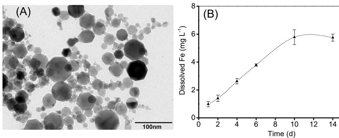
**Figure S1.** Transmission electron microscopic (TEM) image of Fe<sub>2</sub>O<sub>3</sub> NPs (A) and its dynamic dissolution in the Kimura B nutrient solution (B).
