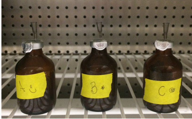
Figure S1. Serum bottle microcosm for bulk soil respiration potential assessment. Bottles were incubated for 1 hour in a controlled growth chamber.
