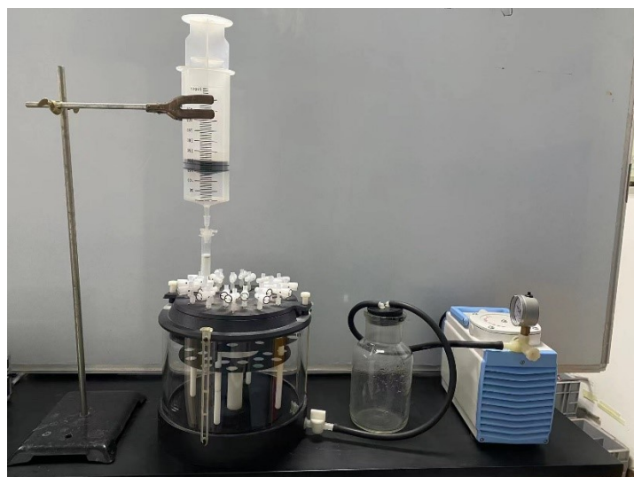
Fig. S2 The setup picture of the fixed-bed column experiments.
