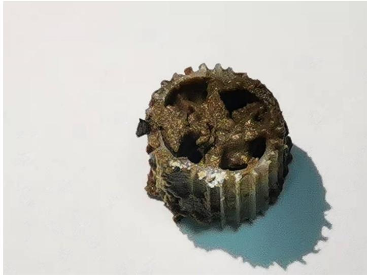
**Figure A.3: Thick biofilm in biocarrier (after 65 d long-term operation).**
