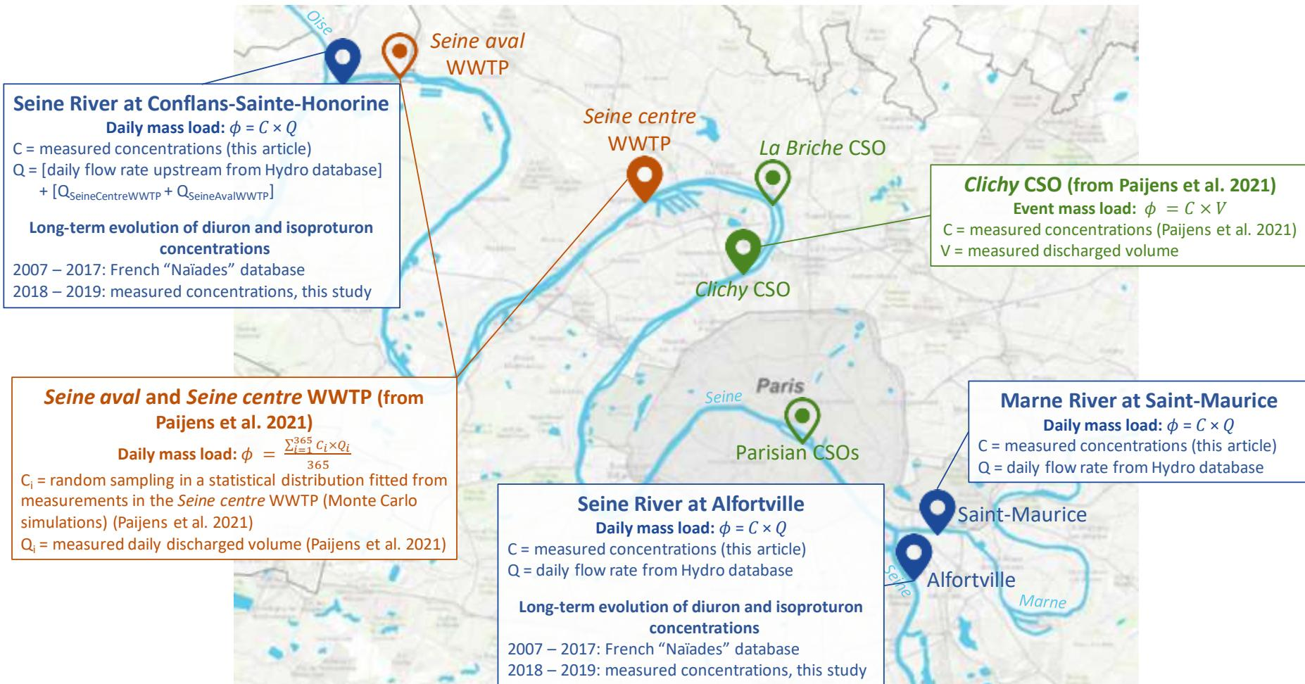
**Fig. S3.** Overview of the overall estimation approach to estimate daily mass loads and to study long-term evolutions of diuron and isoproturon concentrations
